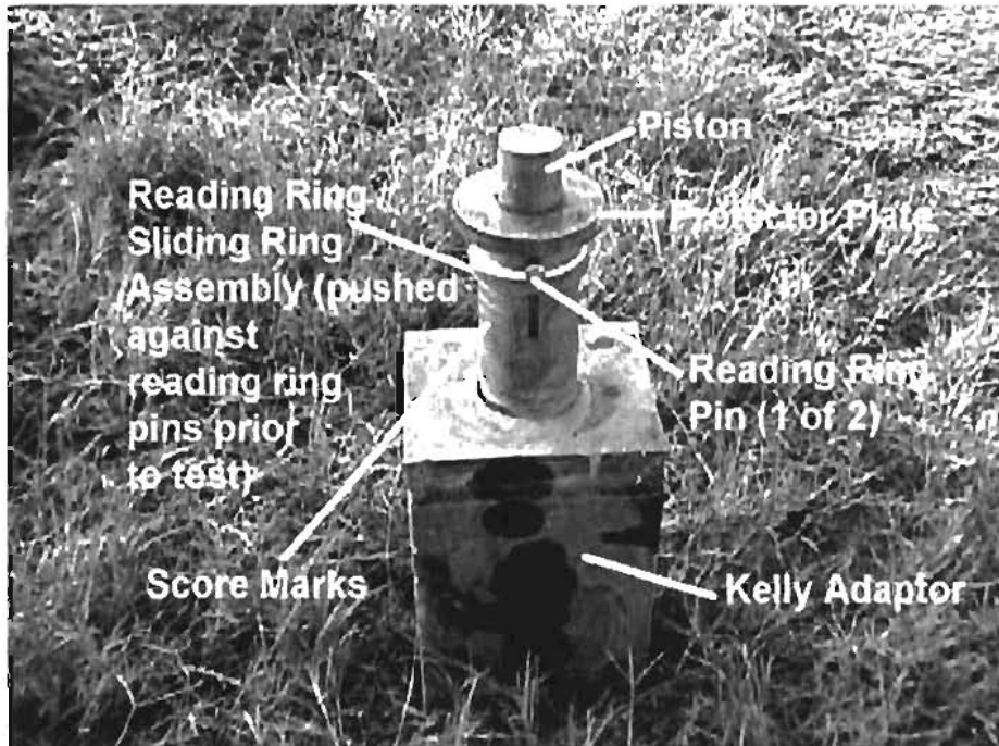
Fig. A.1.1 Penetrometer, Inverted, Prior to Mounting on Kelly
