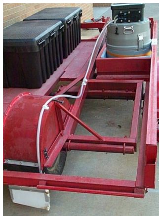
Figure 4-13. ISCO Sampler Collection Hose and Intake Collector
