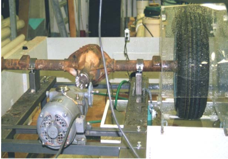
Figure 3-2. Testing Drive Train and Laboratory Simulator
