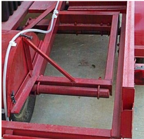
Figure 4-4. Third-Wheel-Frame and Sampling Wheel Axle Attachments
