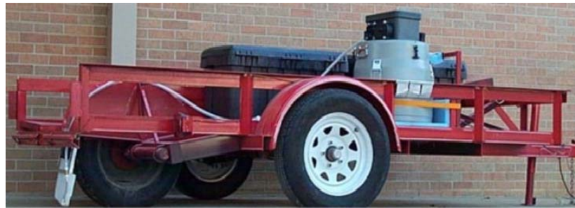
Figure 4-2. Third Wheel in Down Position for Sampling.
