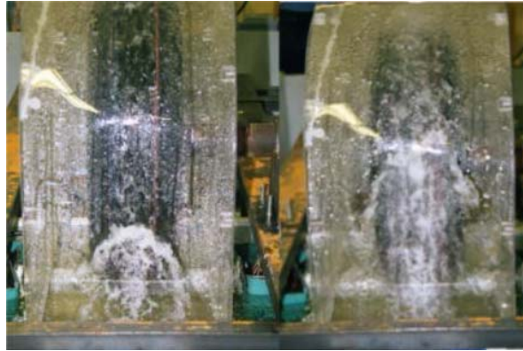
Figure 3-4. Water Discharge Pattern on Rear Finder
