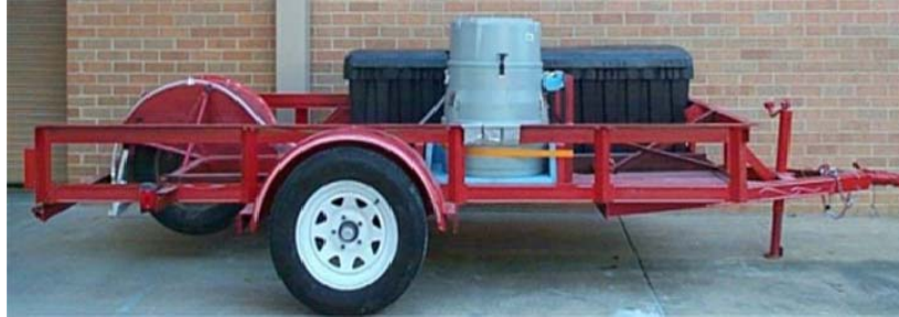
Figure 4-1. Third Wheel (Sampling Wheel) in Up Position for Transport
