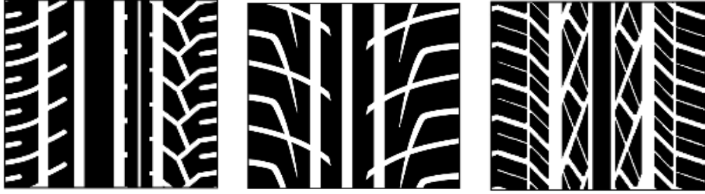
Figure 2-4. Asymmetrical, Unidirectional, and Symmetrical Tread Patterns
