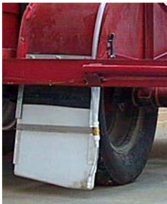
Figure 4-15. Intake Collector From Rear
