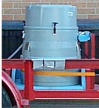
Figure 4-9. ISCO Sampler Mounted on Trailer
