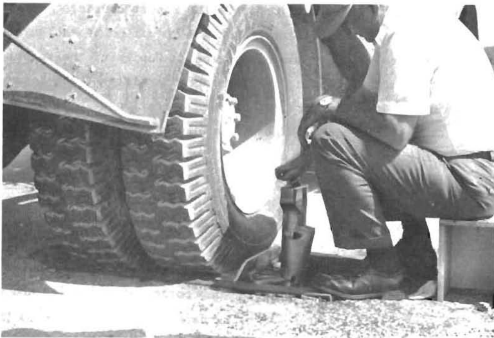
Fig 2.3a. Static wheel load weigher (loadometer).
