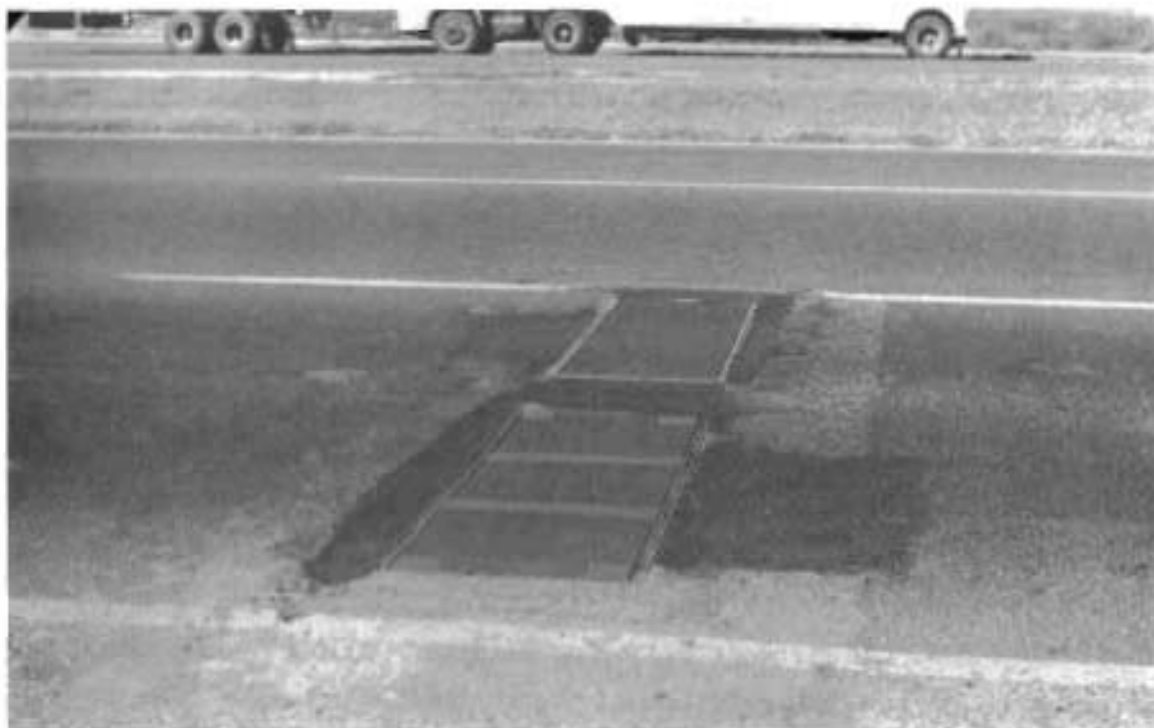
Fig 3.1. Wheel load transducers.
