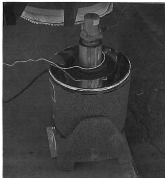
Figure 5.4 – Set up for Calibration of FWD Sensor Outside Holder
