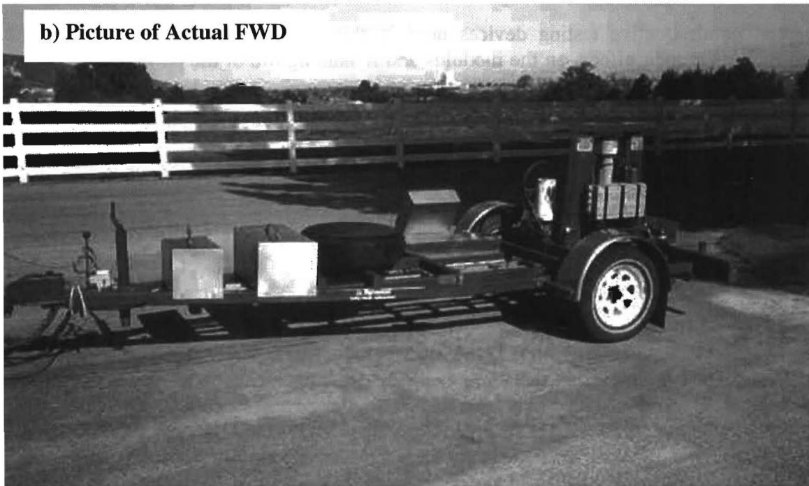
Figure 2.1 Falling Weight Deflectometer
