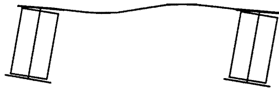
b) Excessive Top Flange Distortion
