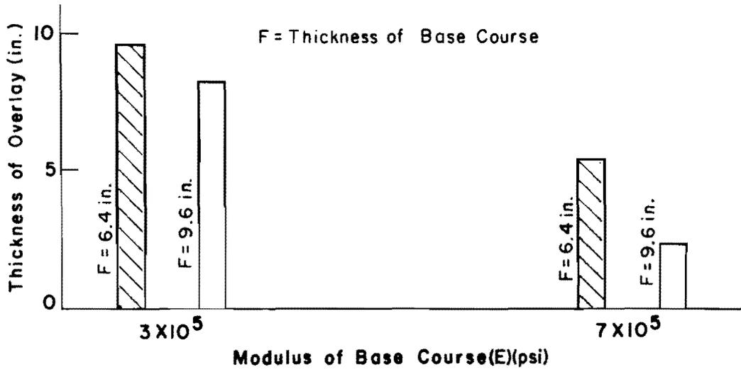
Fig 4.5. Interaction between modulus of base course (E) and thickness of base course (F).
