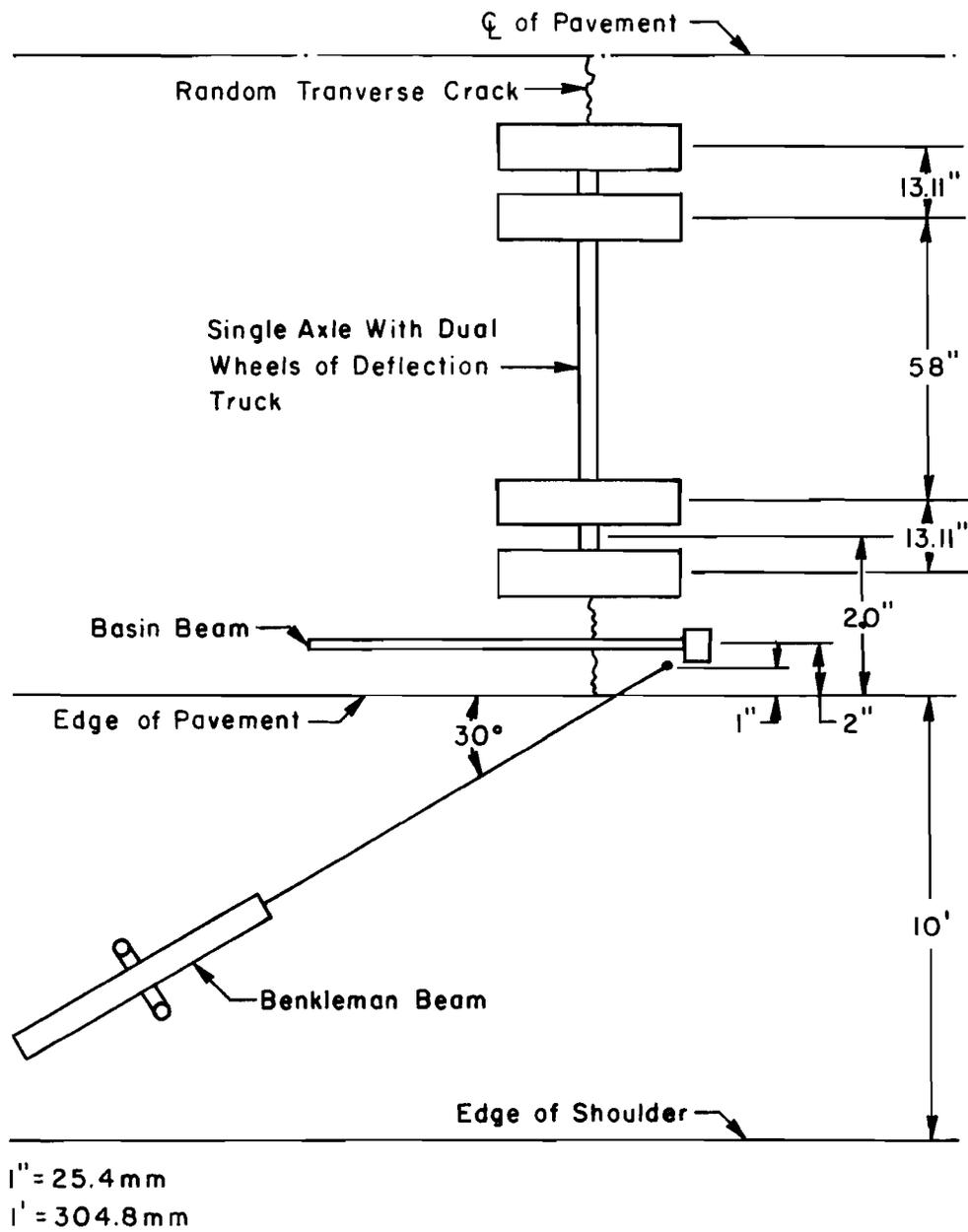
Fig 3.2. Plan view of equipment arrangement for Benkleman Beam.
