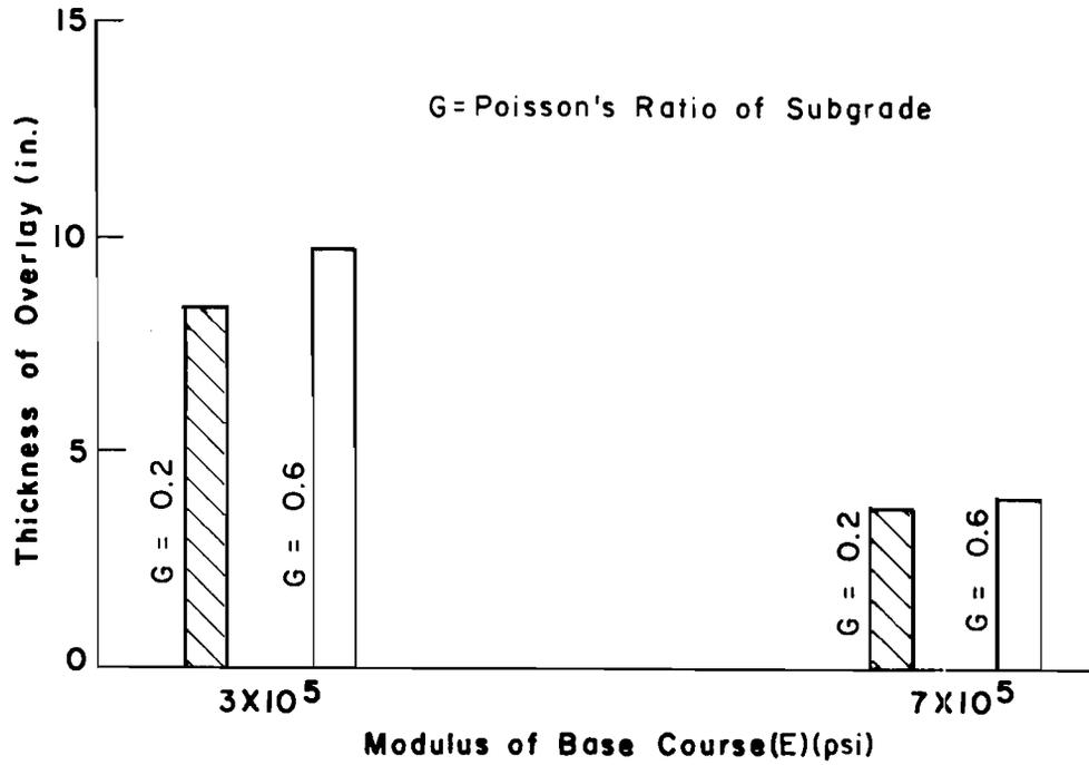
Fig 4.7. Interaction between modulus of base course (E) and Poisson's ration of subgrade (G).
