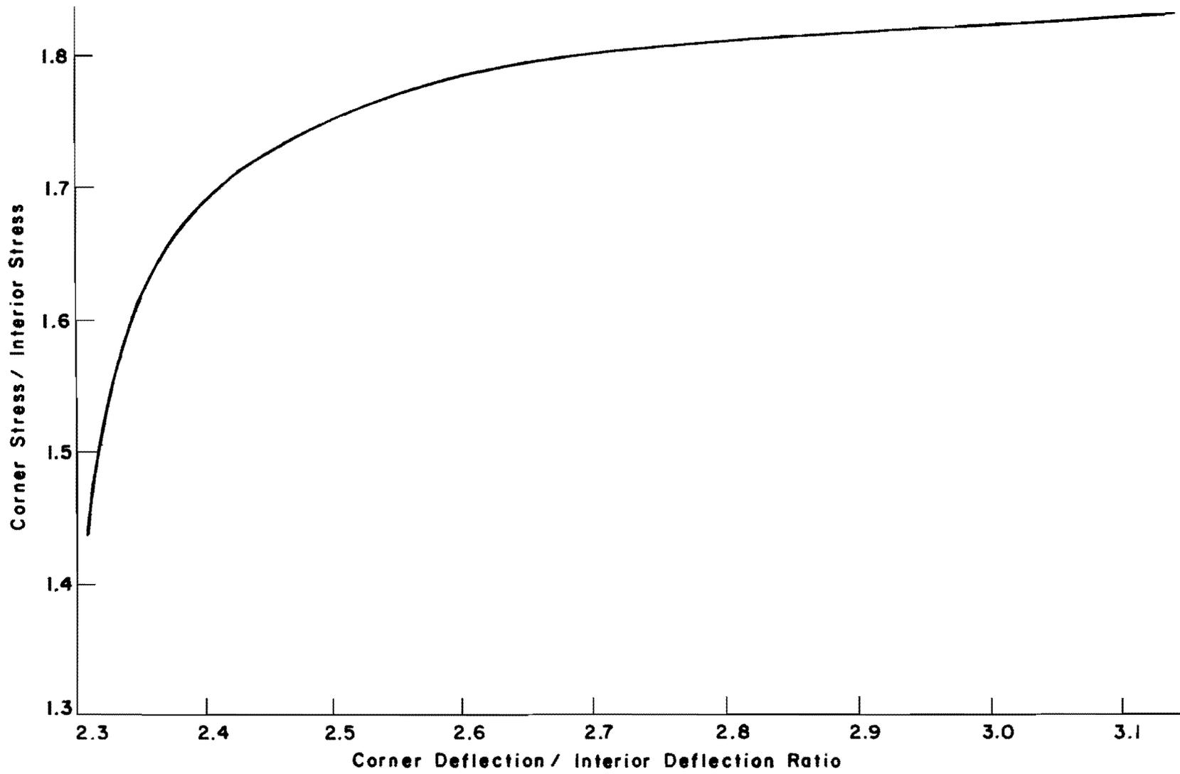
Fig 3.1. Stress ratio curve for design.
