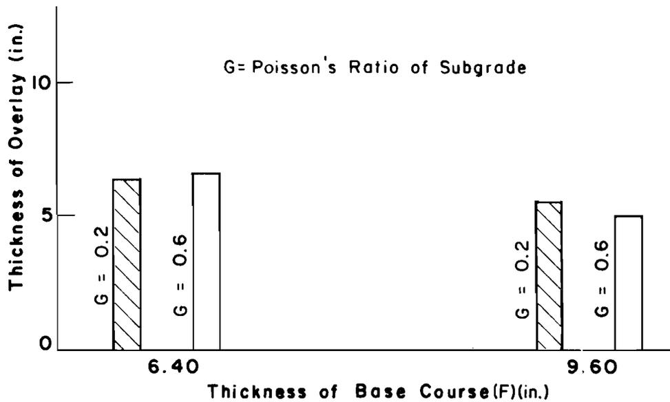
Fig 4.8. Interaction between thickness of base course (F) and Poisson's ratio of subgrade (G).
