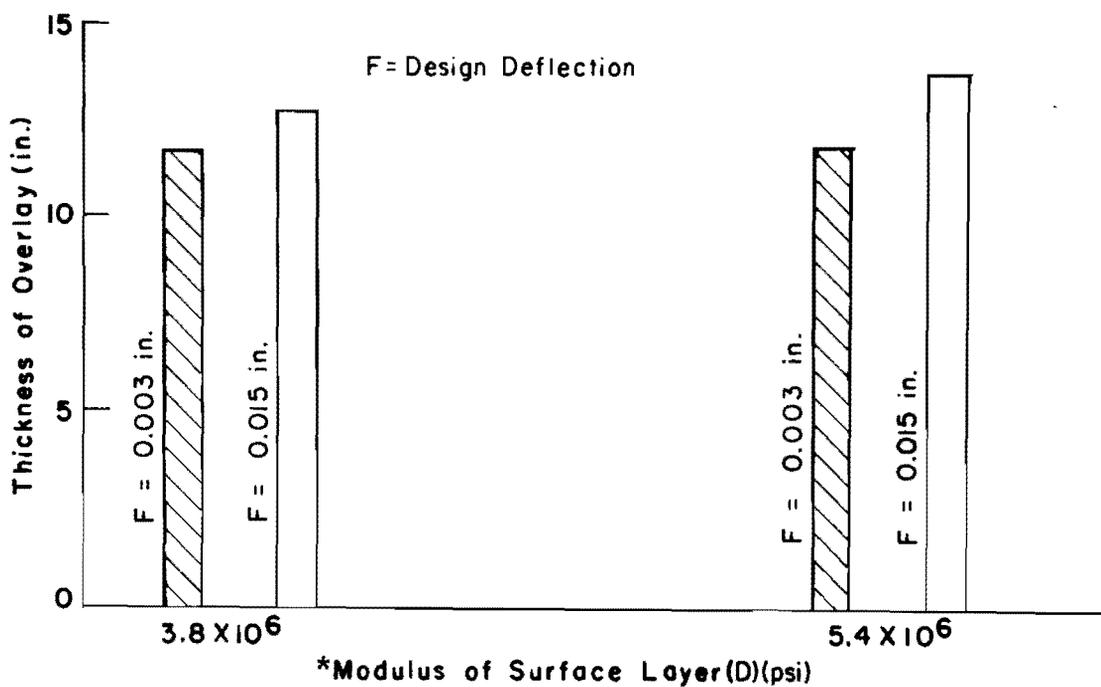
Fig 4.34. Interaction between modulus of surface layer (D) and design deflection (F).
