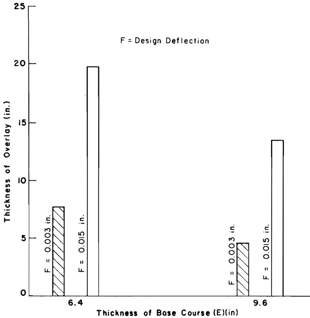
Fig 4.29. Interaction between thickness of base course (E) and design deflection (F).
