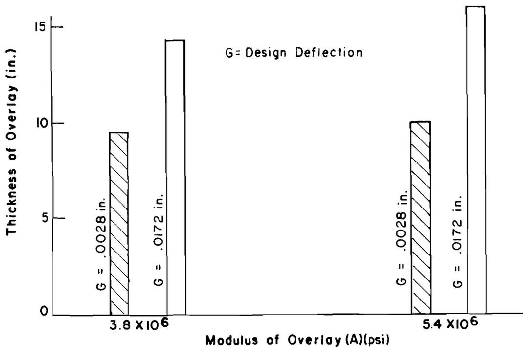
Fig 4.12. Interaction between modulus of overlay (A) and design deflection (G).
