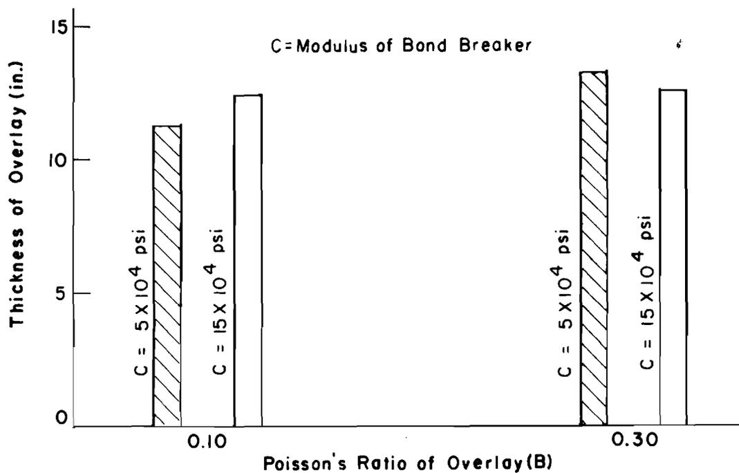
Fig 4.13. Interaction between Poisson's ratio of overlay (B) and modulus of bond breaker (C).
