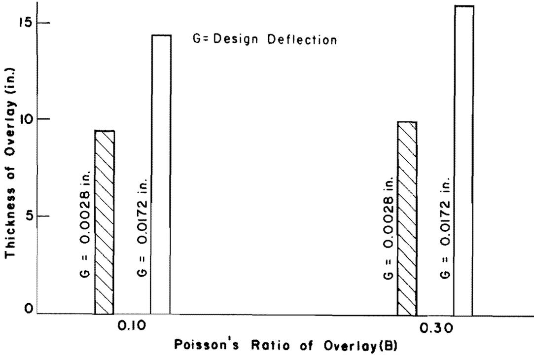
Fig 4.14. Interaction between Poisson's ratio of overlay (B) and design deflection (G).
