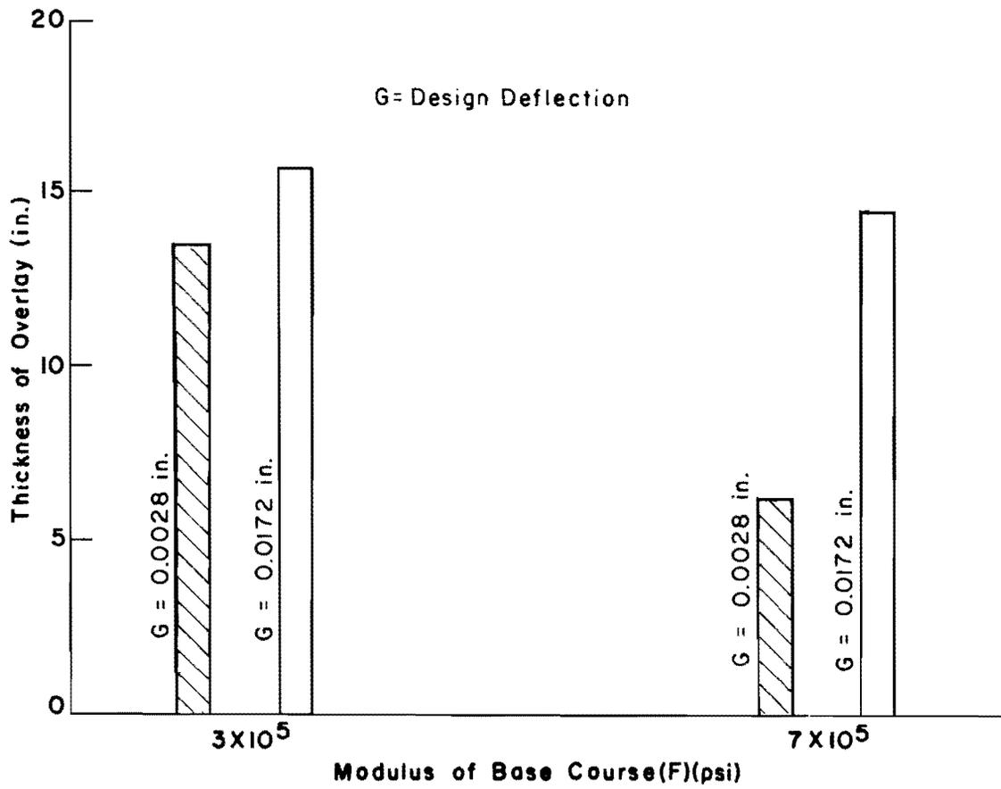
Fig 4.18. Interaction between modulus of base course (F) and design deflection (G).
