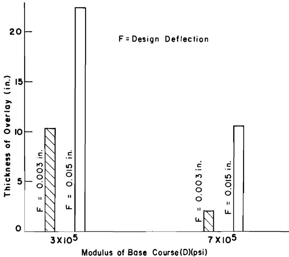
Fig 4.28. Interaction between modulus of base course (D) and design deflection (F).
