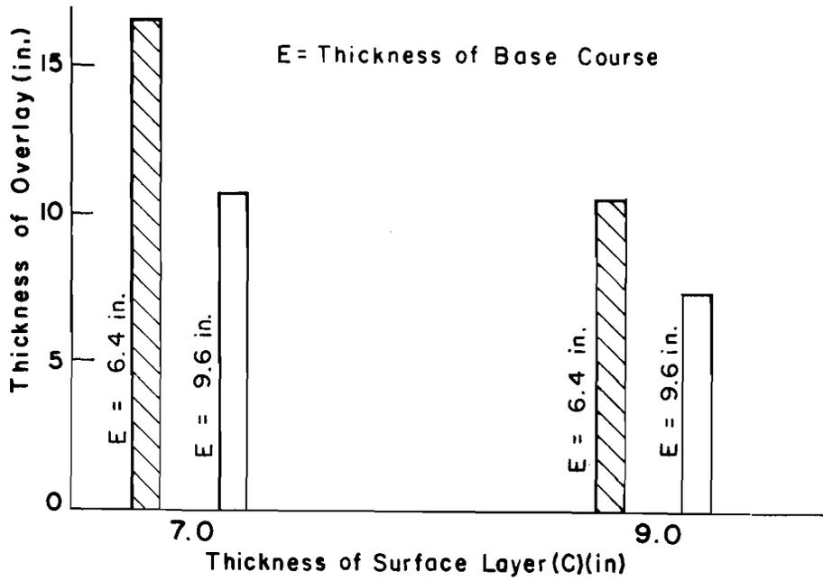
Fig 4.25. Interaction between thickness of surface layer (C) and thickness of base course (E).
