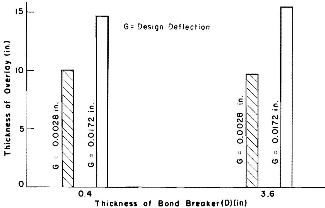
Fig 4.16. Interaction between bond breaker thickness (D) and design deflection (G).
