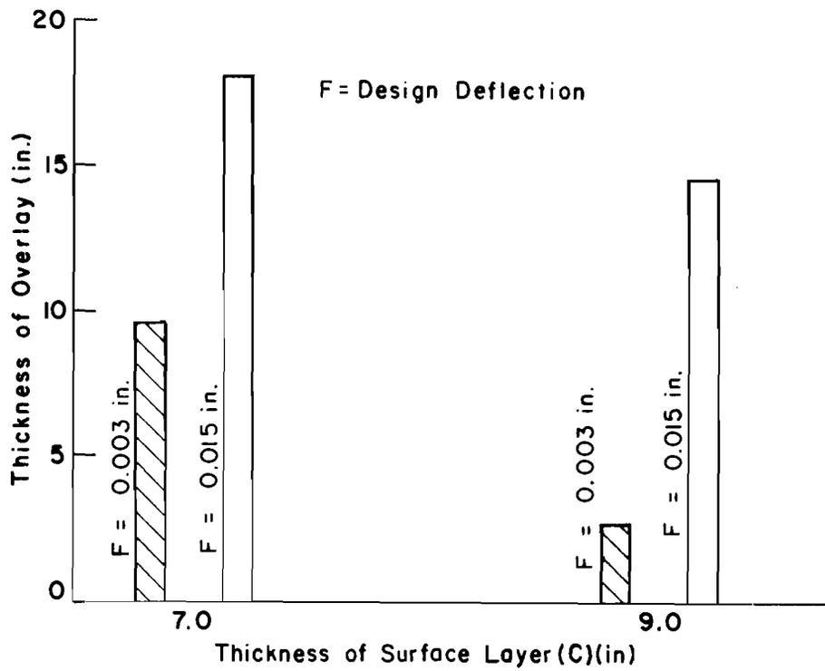
Fig 4.26. Interaction between thickness of surface layer (C) and design deflection (F).
