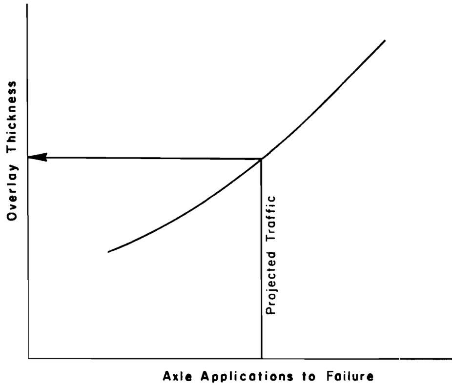
Fig 2.4. Relation of thickness and fatigue life used in selecting required overlay thickness for rigid pavements.
