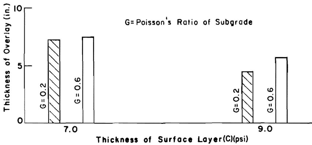
Fig 4.6. Interaction between thickness of surface layer (C) and Poisson's ration of subgrade (G).
