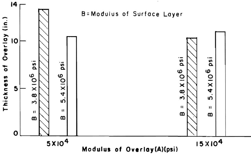
Fig 4.21. Interaction between modulus of overlay (A) and modulus of surface layer (B).
