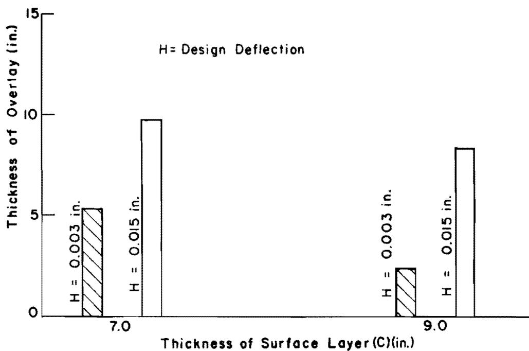
Fig 4.9. Interaction between thickness of surface layer (C) and design deflection (H).
