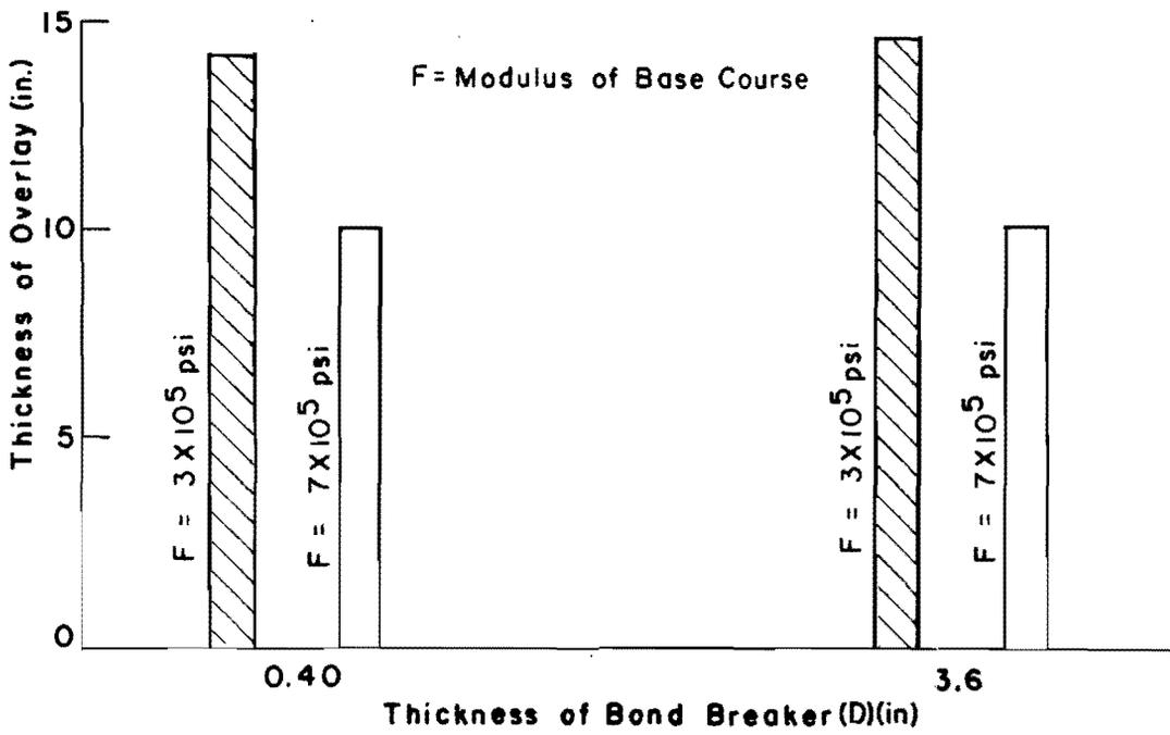
Fig 4.15. Interaction between bond breaker thickness (D) and modulus of base (F).
