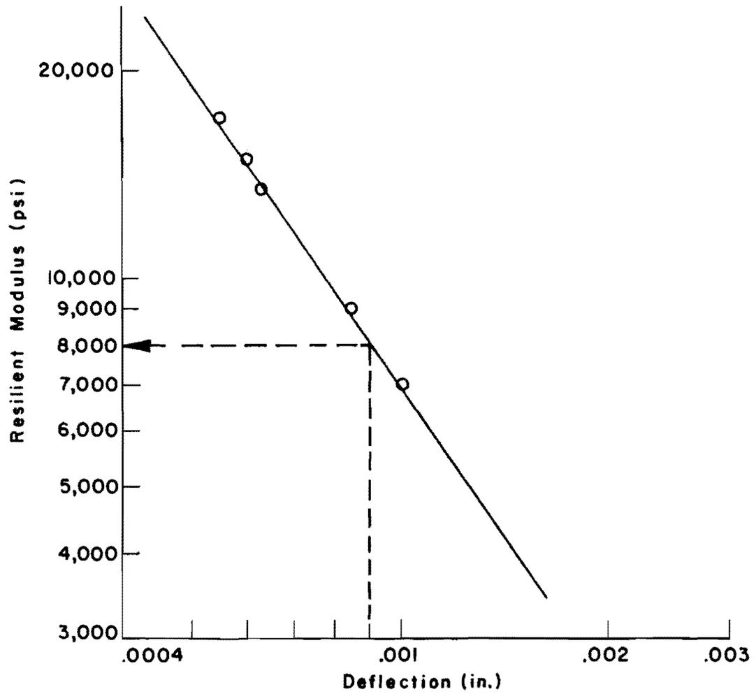
Fig 2.3. Relationship of computed deflection and subgrade modulus.
