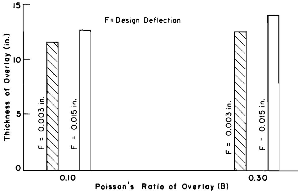
Fig 4.33. Interaction between Poisson's ratio of overlay (B) and design deflection (F).
