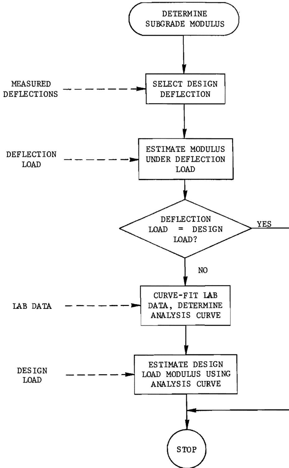
Fig 2.2. Determination of subgrade modulus.
