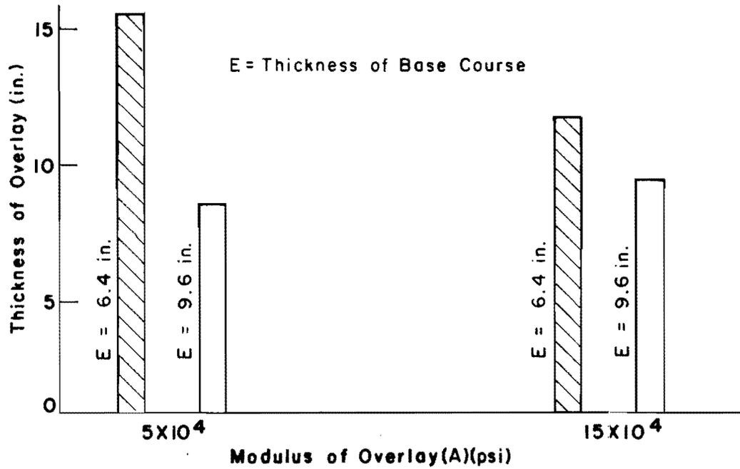
Fig 4.22. Interaction between modulus of overlay (A) and thickness of base course (E).
