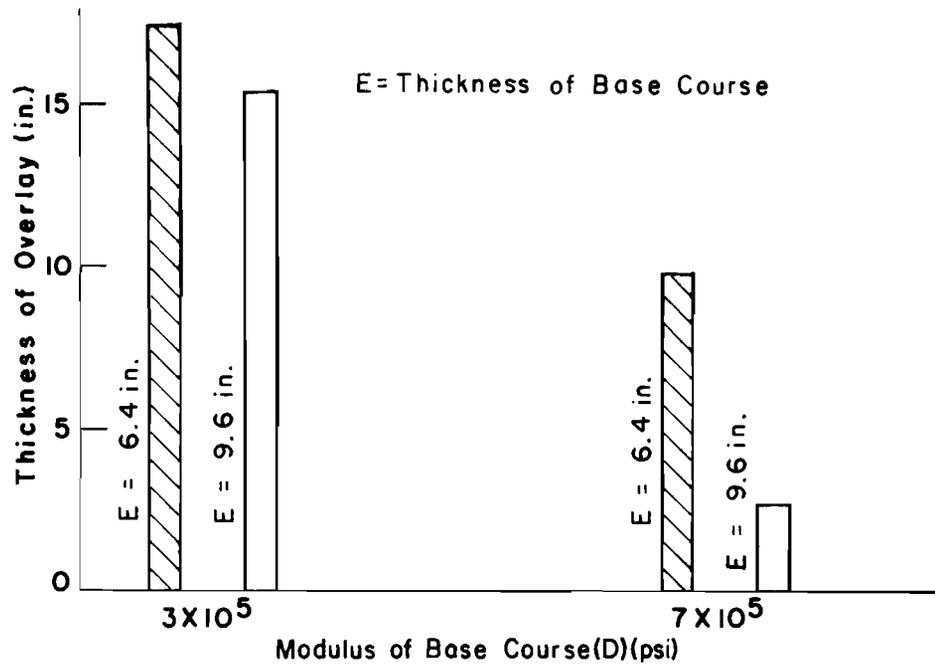
Fig 4.27. Interaction between modulus of base course (D) and thickness of base course (E).
