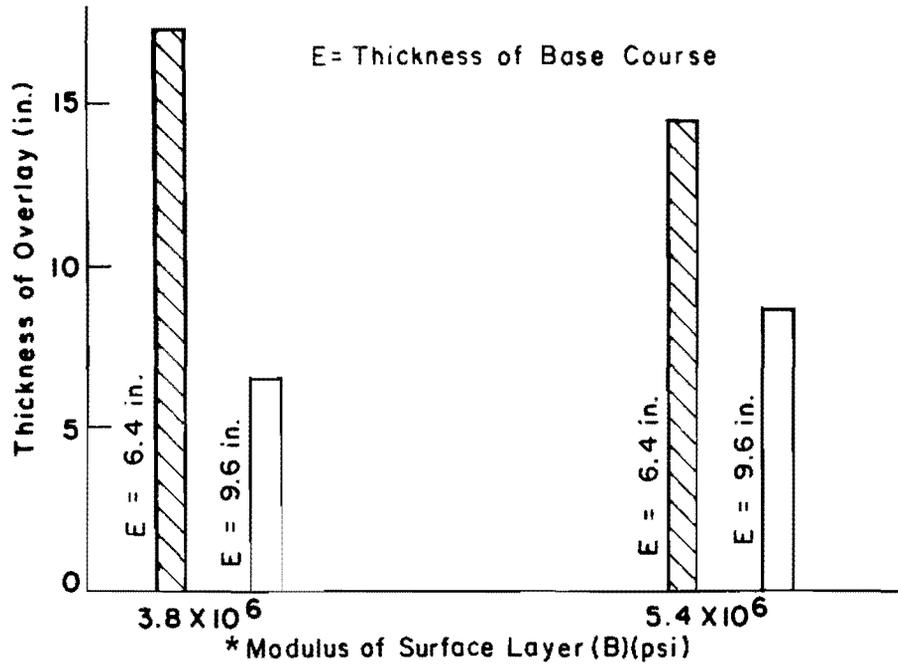
Fig 4.23. Interaction between modulus of surface layer (B) and thickness of base course (E).
