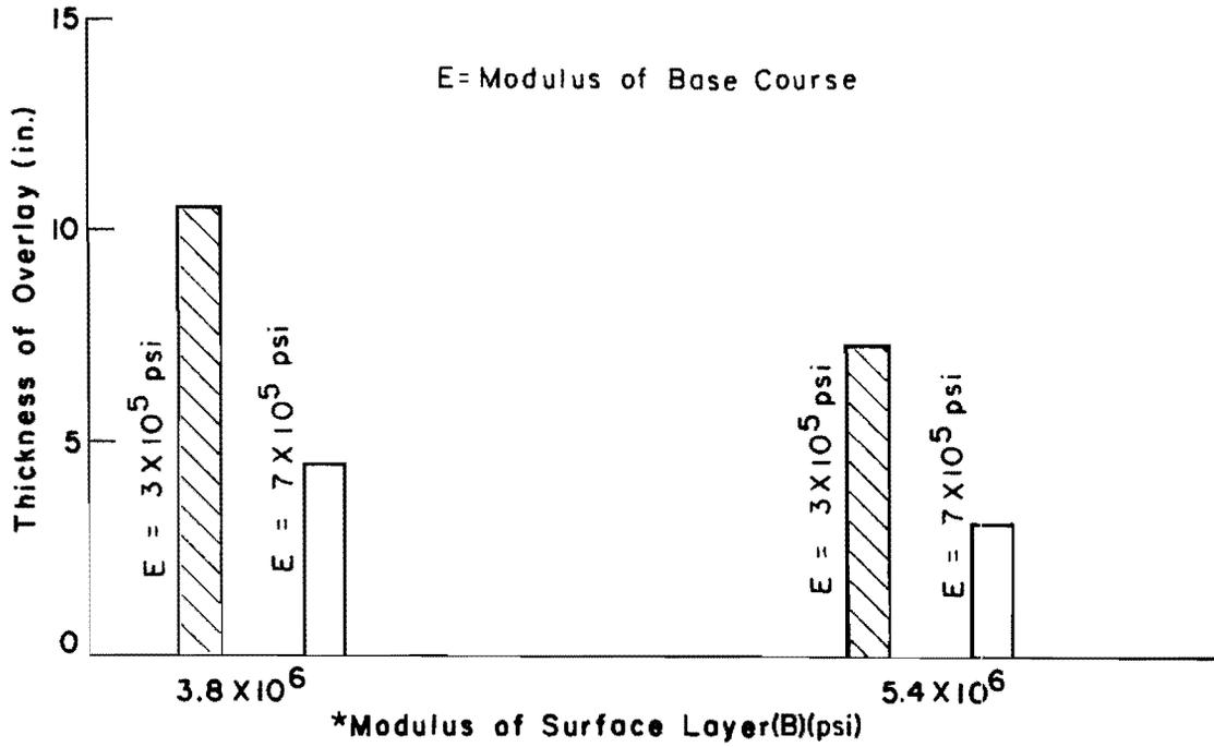
Fig 4.3. Interaction between modulus of surface layer (B) and modulus of base course (E).
