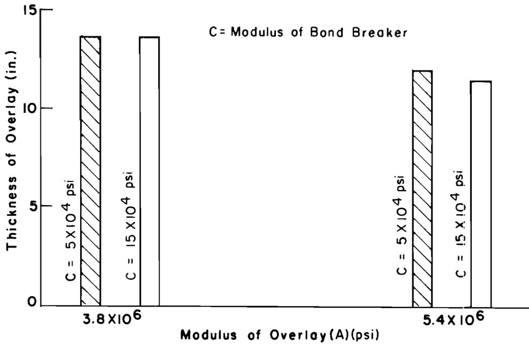
Fig 4.32. Interaction between modulus of overlay (A) and modulus of bond breaker (C).
