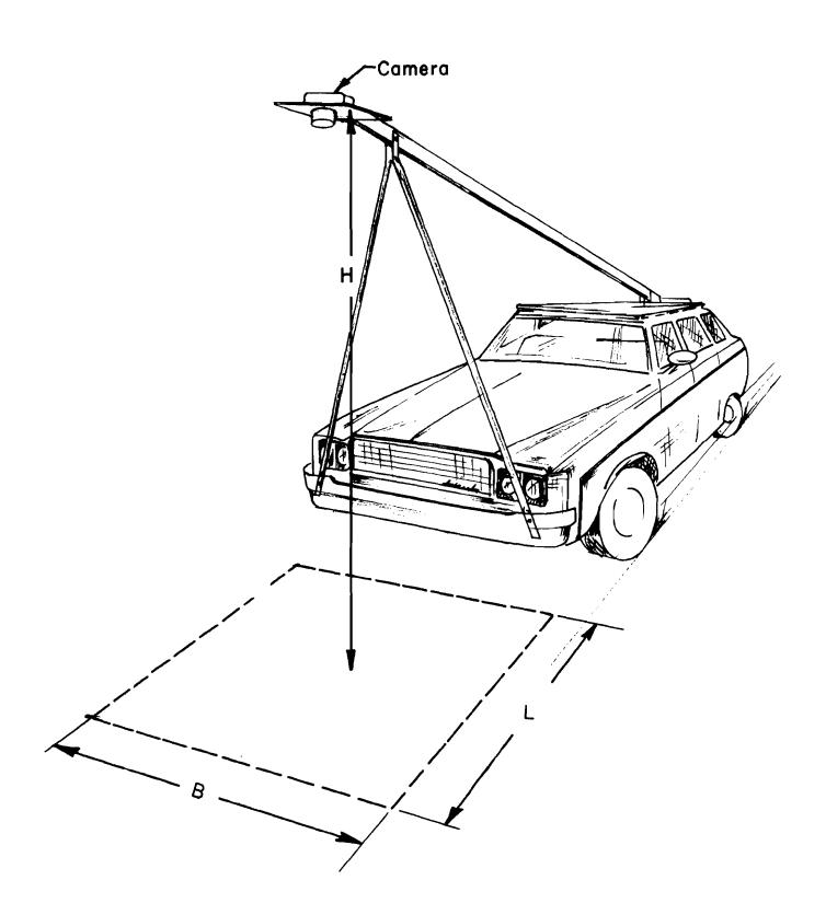
Fig 3.1. Relative position of camera on vehicle.
