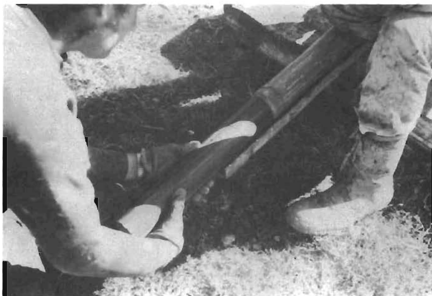
Fig 4.8. Soil sample almost completely pushed out of the push barrel. (Notice cracks forming on sample just after extraction.)
