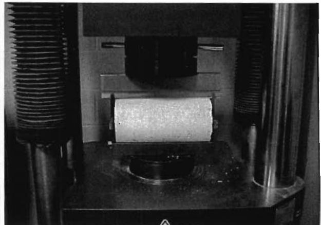
Figure 3.2 - Split Tensile Test in Progress
