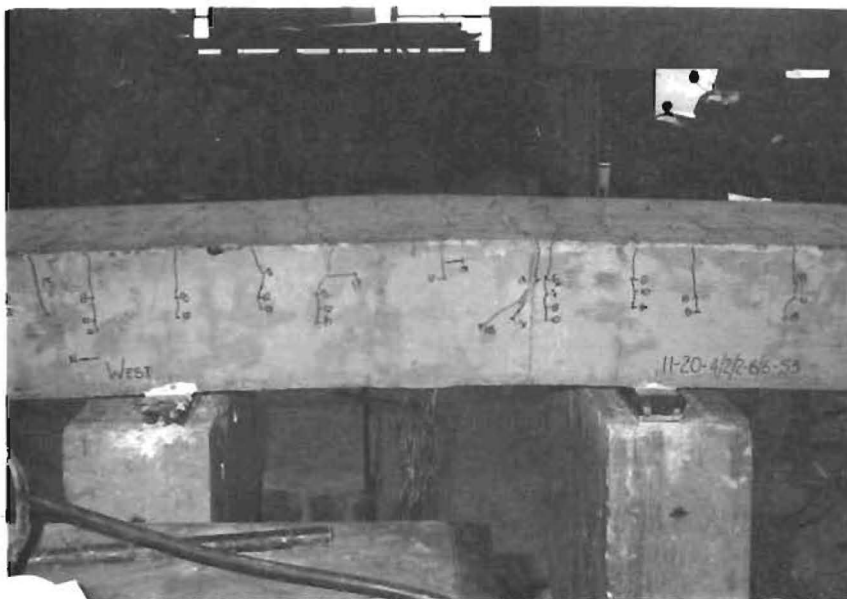
Fig. 3.17. Side view of 11-20-4/2/2-6/6-S3 after failure
