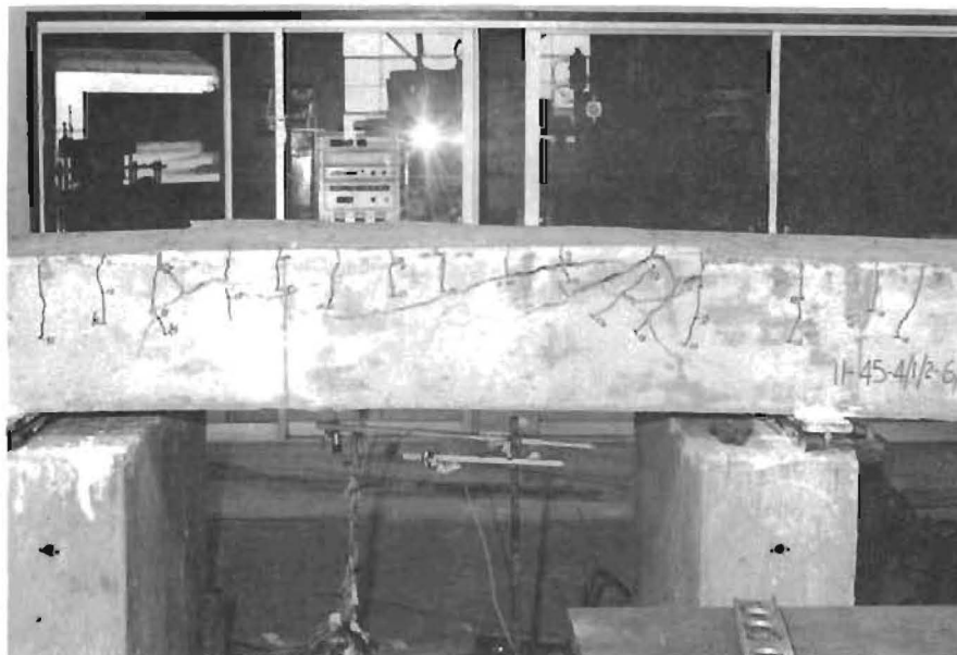
Fig. 3.7. Side view of 11-45-4/1/2-6/6 after failure
