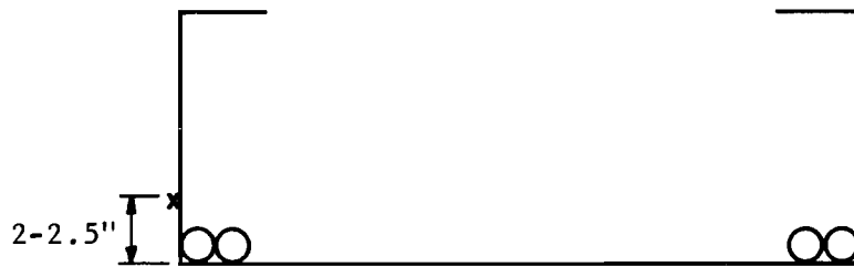
Detail of gage location on stirrups
