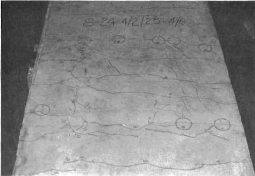
Fig. 3.14. Tension face of 8-24-4/2/2.5-4/6 after failure
