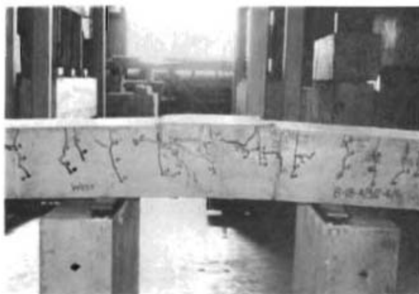
Fig. 3.13. Side view of 8-18-4/3/2-6/6 after failure
