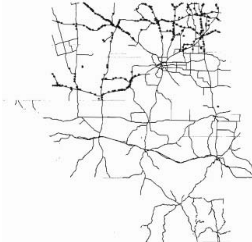
Figure 5.2 Bridges Recommended for Load-Posting in San Angelo District.
