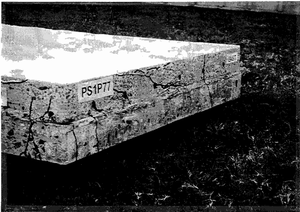
Figure 8.8: Saw cut face (transverse section) of precast prestressed panel pulsating fatigue test Specimen PS1P77.
