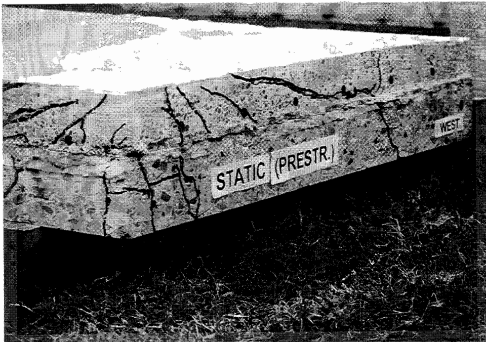
Figure 8.6: Saw cut face (transverse section) of a precast prestressed panel static test specimen.
