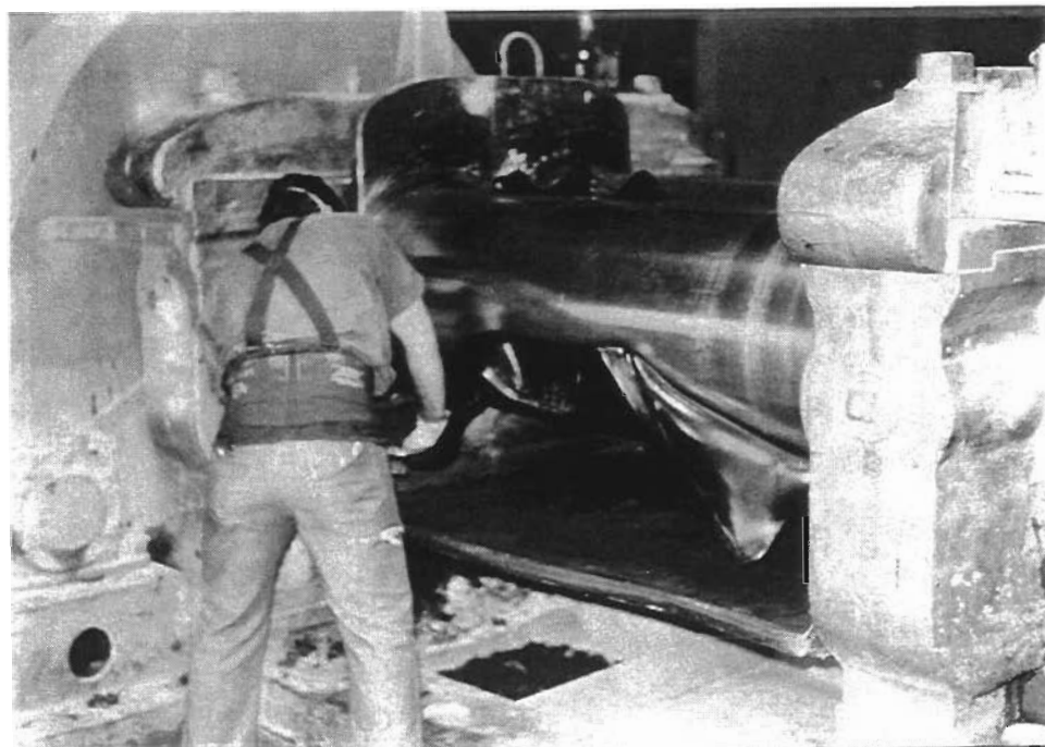
Figure 2- 4 The rubber band is cut from the mill
