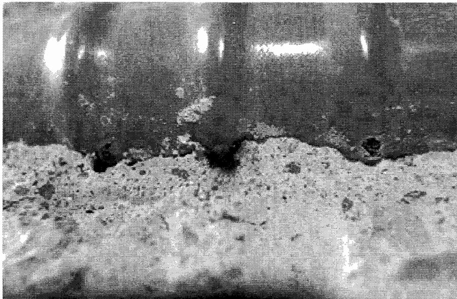
*Figure 4.1 Blister at bottom side of coated bar*
