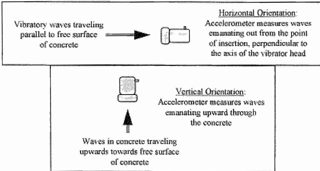
Figure 3.5 Accelerometer orientation
