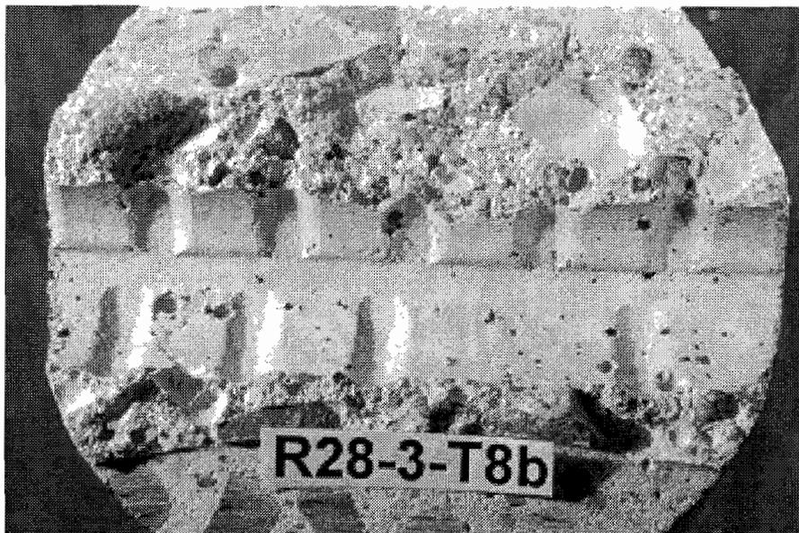
*Figure 4. 21 Typical distribution of voids under rebar*
