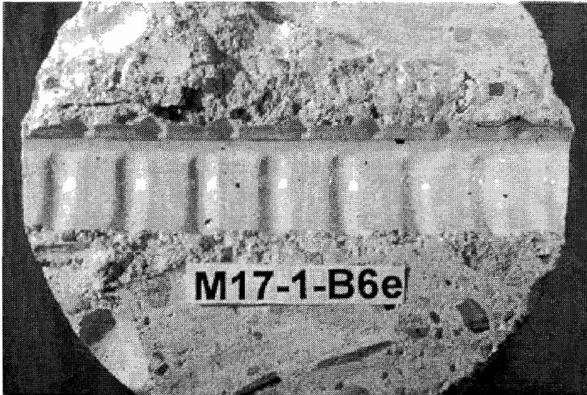
*Figure 4. 19 Smooth and shiny surface under epoxy-coated rebar*
