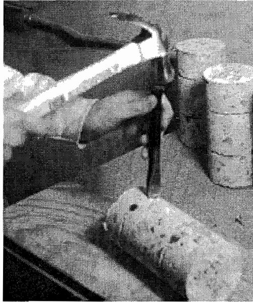
*Figure 4. 17 Splitting cores at level of reinforcement*
