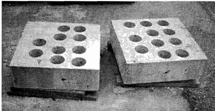
*Figure 4. 15 Specimens M8 and R8 after coring*
