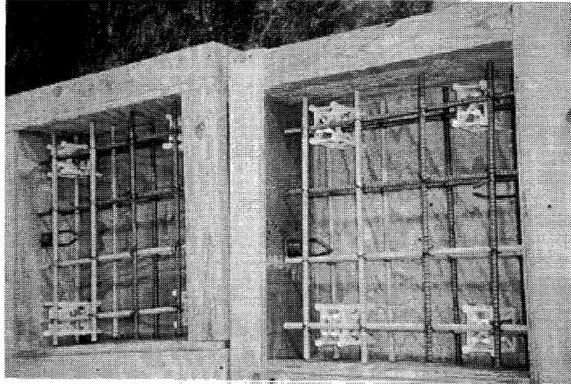
*Figure 4.4 Reinforcement of Specimens M8 and R8*
