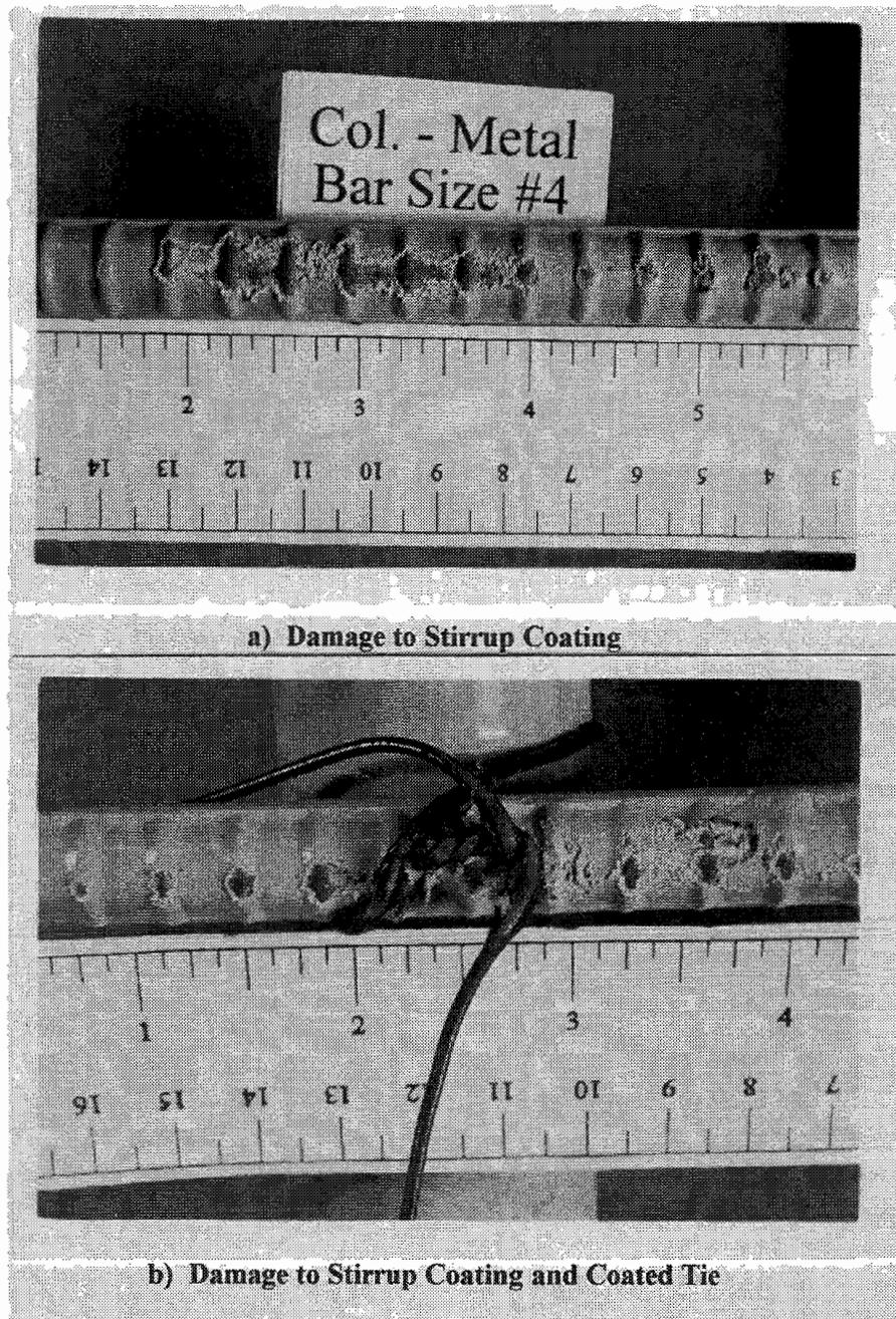
Figure 2. 20 Coating damage with metal vibrator head
