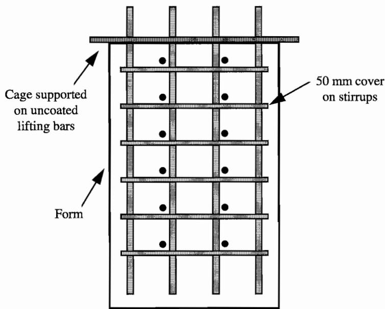
Figure 2.1 Details of column specimen
