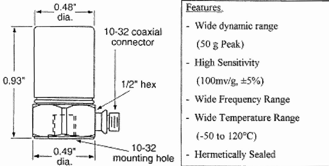
Figure 3.4 Accelerometer features
