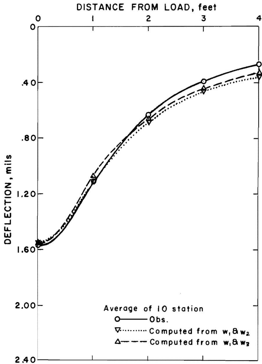
Figure 5c: Computed and average observed Dynaflect deflection basins, Section 5.  $E_1(w_1, w_2) \approx E_1(w_1, w_3)$  and  $E_2(w_1, w_2) \approx E_2(w_1, w_3)$  by statistical test.
