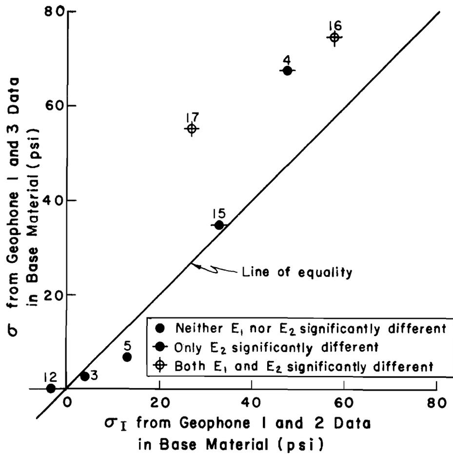
Figure 8: Comparison of the major principal stresses in the base material at the point  $x = 0, y = 0, z = h$ , as computed from data from different pairs of geophones. Significance data from Tables 7 and 8.
