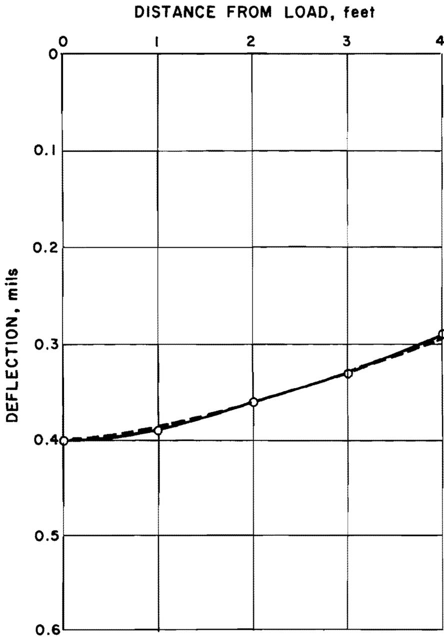
Figure 10d: Observed deflection basin (solid line through circled points) compared with theoretical basin (dashed line) computed from  $E_1 (w_1, w_3)$  and  $E_2 (w_1, w_3)$  at Test Point 25. Moduli are given in Table 10.
