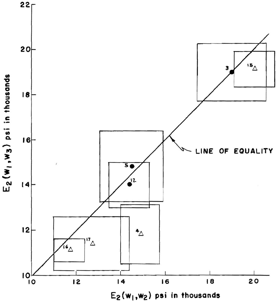
Figure 4b: Comparison of  $E_2$  computed from  $w_1$  and  $w_2$ , with  $E_2$  computed from  $w_1$  and  $w_3$ . The rectangles represent within-section standard deviations of  $E_2$ , with the mean value plotted at the center. Points shown as triangles indicate that the two moduli are significantly different according to a statistical test.
