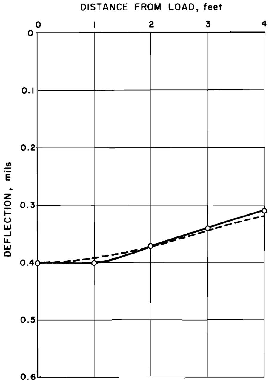
Figure 10a: Observed deflection basin (solid line through circled points) compared with theoretical basin (dashed line) computed from  $E_1 (w_1, w_3)$  and  $E_2 (w_1, w_3)$  at Test Point 6. Moduli are given in Table 10.
