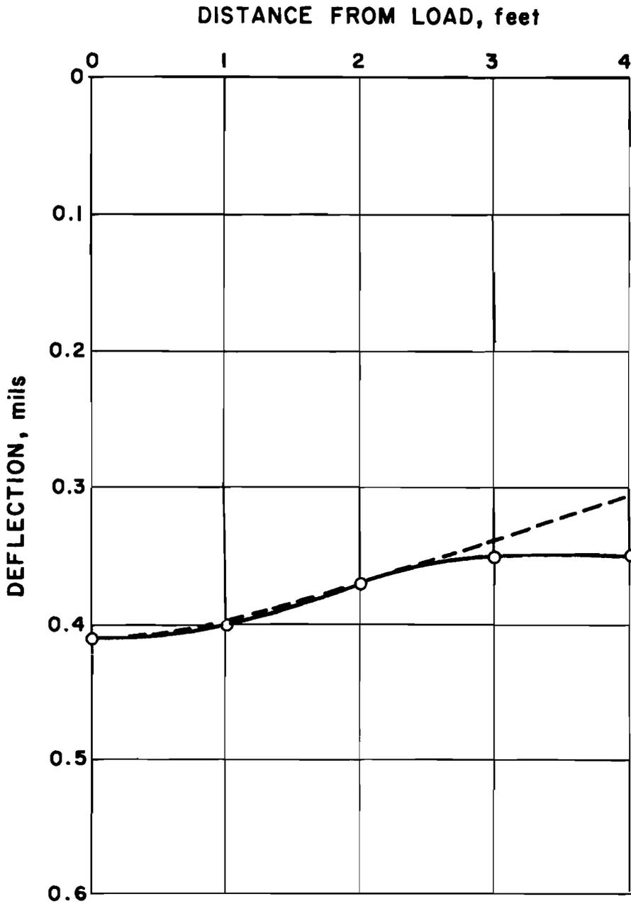
Figure 10h: Observed deflection basin (solid line through circled points) compared with theoretical basin (dashed line) computed from  $E_1 (w_1, w_3)$  and  $E_2 (w_1, w_3)$  at Test Point 49. Moduli are given in Table 10.
