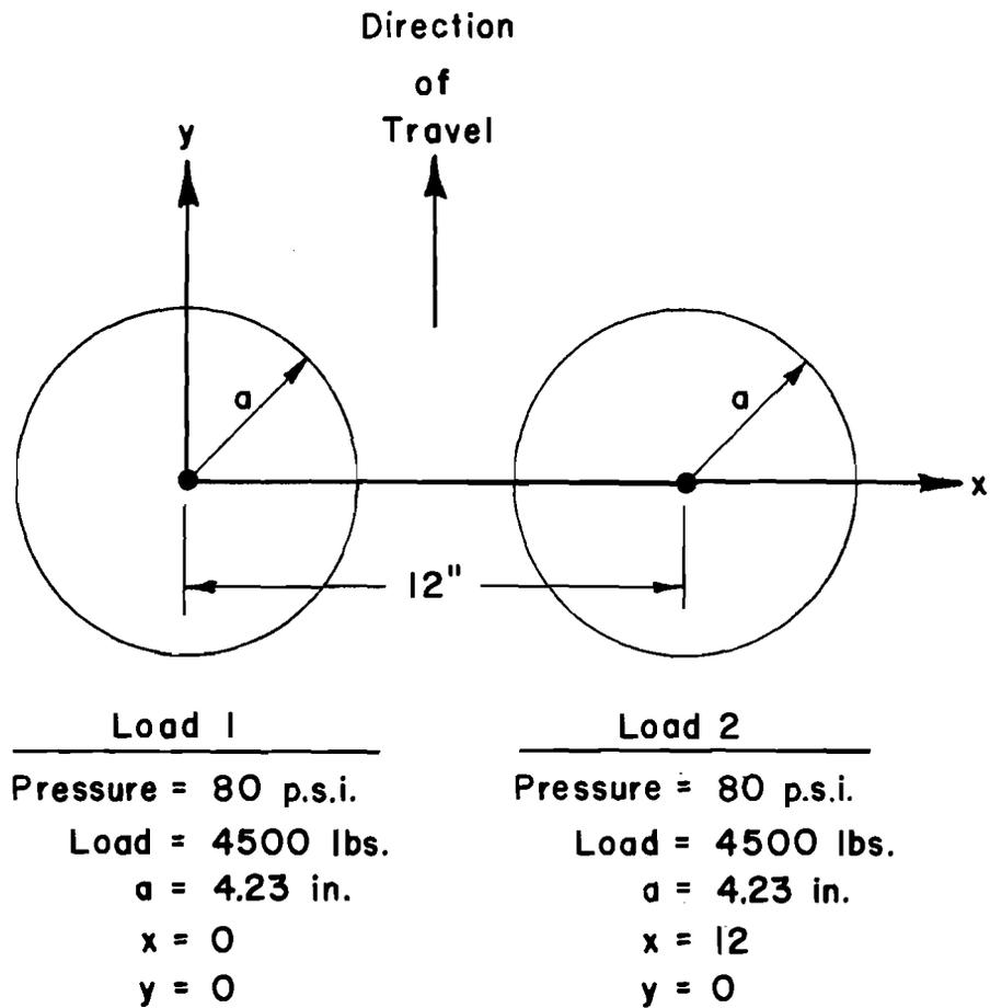
Figure 6: Plan view of simulated dual wheel tire-pavement contact areas, with parameters used in BISTRO for computing principal stresses at the base-subbase interface.
