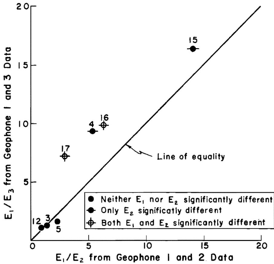
Figure 7: Comparison of the ratio,  $E_1/E_2$ , computed from data from different pairs of geophones. Significance data from Tables 7 and 8.
