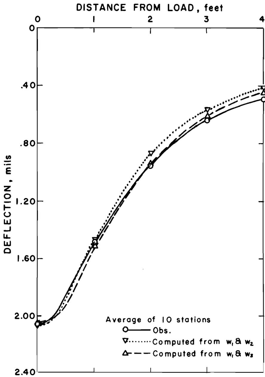
Figure 5f: Computed and average observed Dynaflect deflection basins, Section 16.  $E_1(w_1, w_2) < E_1(w_1, w_3)$  but  $E_2(w_1, w_2) > E_2(w_1, w_3)$  by statistical test.
