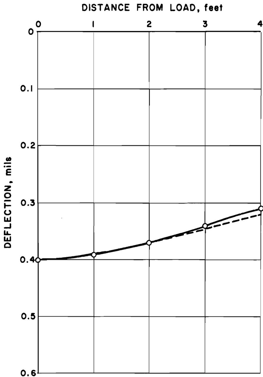
Figure 10g: Observed deflection basin (solid line through circled points) compared with theoretical basin (dashed line) computed from  $E_1 (w_1, w_3)$  and  $E_2 (w_1, w_3)$  at Test Point 34. Moduli are given in Table 10.
