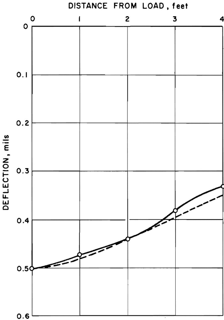
Figure 10b: Observed deflection basin (solid line through circled points) compared with theoretical basin (dashed line) computed from  $E_1 (w_1, w_3)$  and  $E_2 (w_1, w_3)$  at Test Point 10. Moduli are given in Table 10.
