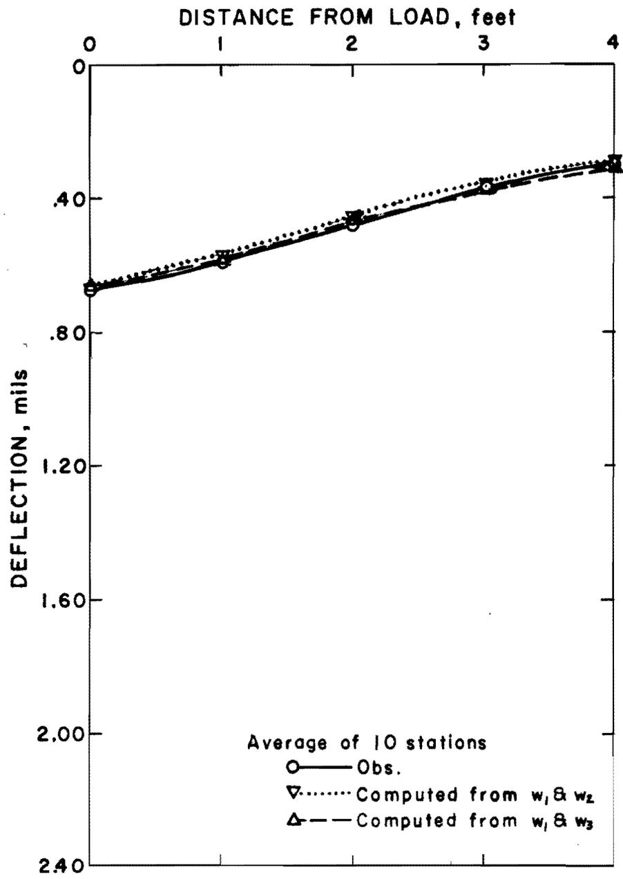
Figure 5e: Computed and average observed Dynaflect deflection basins, Section 17.  $E_1 (w_1, w_2) \approx E_1 (w_1, w_3)$  but  $E_2 (w_1, w_2) > E_2 (w_1, w_3)$  by statistical test.
