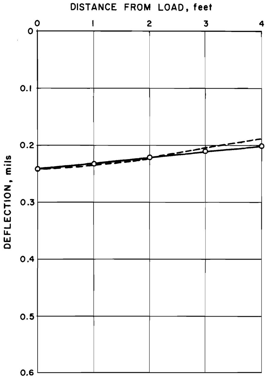
Figure 10k: Observed deflection basin (solid line through circled points) compared with theoretical basin (dashed line) computed from  $E_1 (w_1, w_3)$  and  $E_2 (w_1, w_3)$  at Test Point 69. Moduli are given in Table 10.
