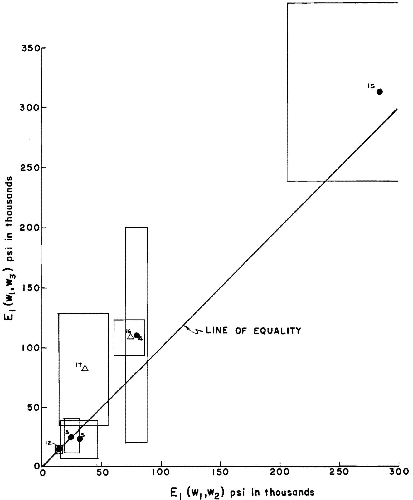
Figure 4a: Comparison of  $E_1$  computed from  $w_1$  and  $w_2$ , with  $E_1$  computed from  $w_1$  and  $w_3$ . The rectangles represent within-section standard deviations of  $E_1$ , with the mean value plotted at the center. Points shown as triangles indicate that the two moduli are significantly different according to a statistical test.
