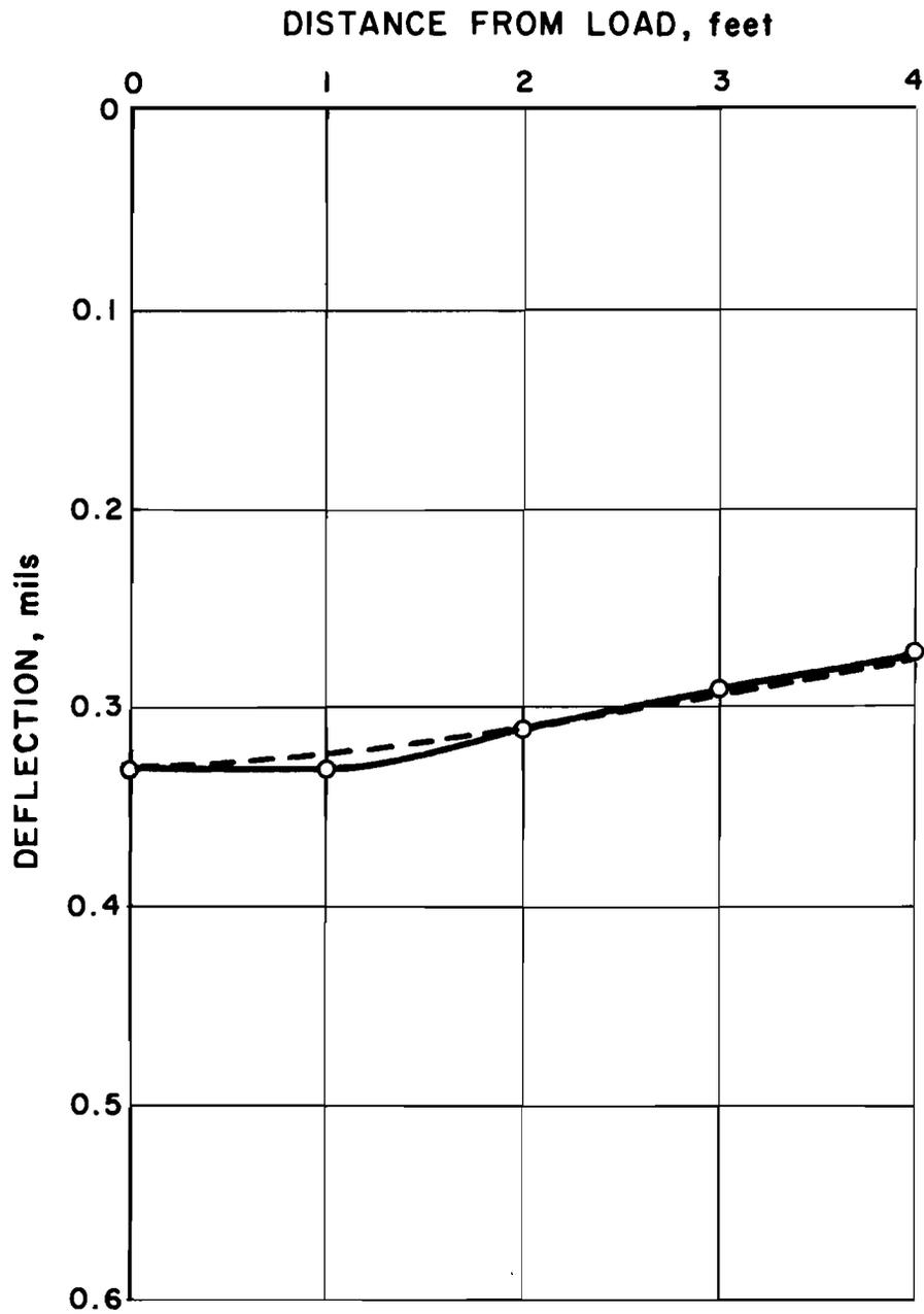
Figure 10i: Observed deflection basin (solid line through circled points) compared with theoretical basin (dashed line) computed from  $E_1 (w_1, w_3)$  and  $E_2 (w_1, w_3)$  at Test Point 56. Moduli are given in Table 10.
