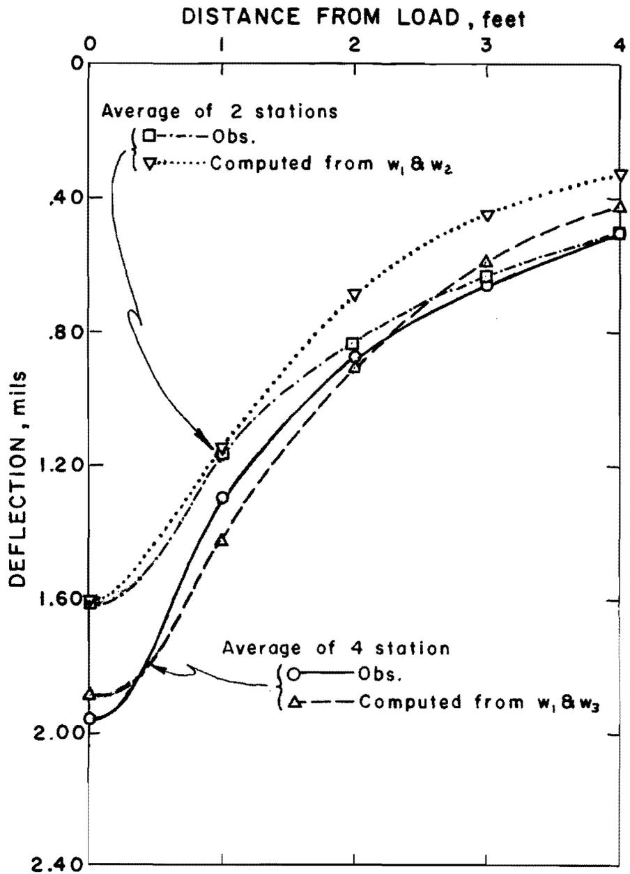
Figure 5b: Computed and average observed Dynaflect deflection basins, Section 4.  $E_1(w_1, w_2) \approx E_1(w_1, w_3)$  but  $E_2(w_1, w_2) > E_2(w_1, w_3)$  by statistical test.
