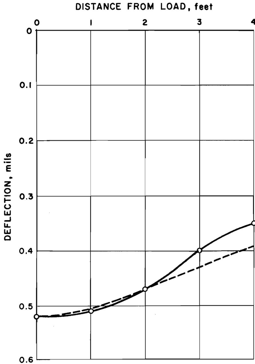
Figure 10c: Observed deflection basin (solid line through circled points) compared with theoretical basin (dashed line) computed from  $E_1 (w_1, w_3)$  and  $E_2 (w_1, w_3)$  at Test Point 13. Moduli are given in Table 10.
