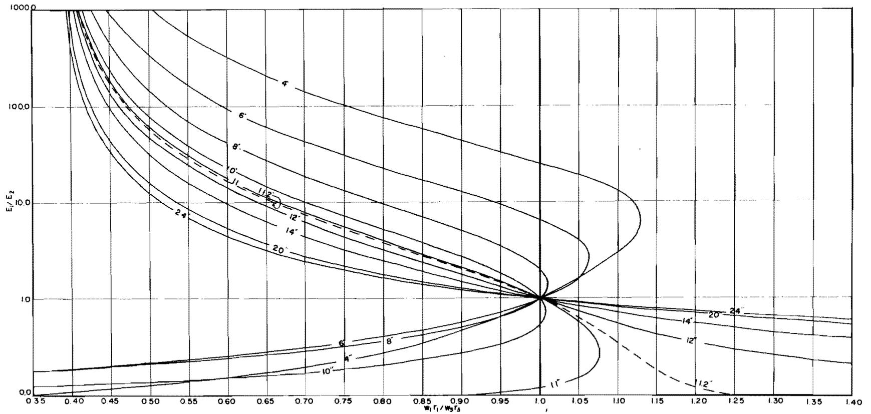
Figure 3: Contours of pavement thickness,  $h$ , plotted as a function of the ratios  $E_1/E_2$  and  $w_1 r_1 / w_3 r_3$ .
