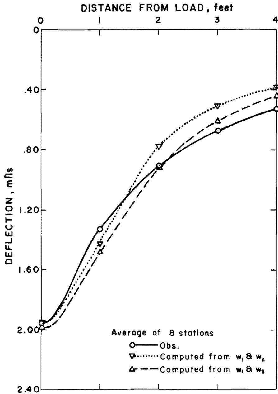
Figure 5g: Computed and average observed Dynaflect deflection basins, Section 17.  $E_1 (w_1, w_2) < E_1 (w_1, w_3)$  but  $E_2 (w_1, w_2) > E_2 (w_1, w_3)$  by statistical test.
