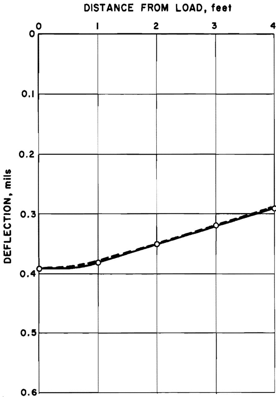
Figure 10j: Observed deflection basin (solid line through circled points) compared with theoretical basin (dashed line) computed from  $E_1 (w_1, w_3)$  and  $E_2 (w_1, w_3)$  at Test Point 63. Moduli are given in Table 10.
