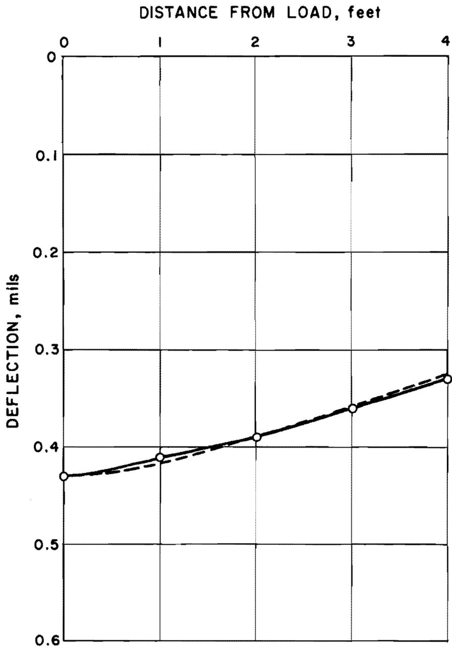
Figure 10e: Observed deflection basin (solid line through circled points) compared with theoretical basin (dashed line) computed from  $E_1 (w_1, w_3)$  and  $E_2 (w_1, w_3)$  at Test Point 28. Moduli are given in Table 10.
