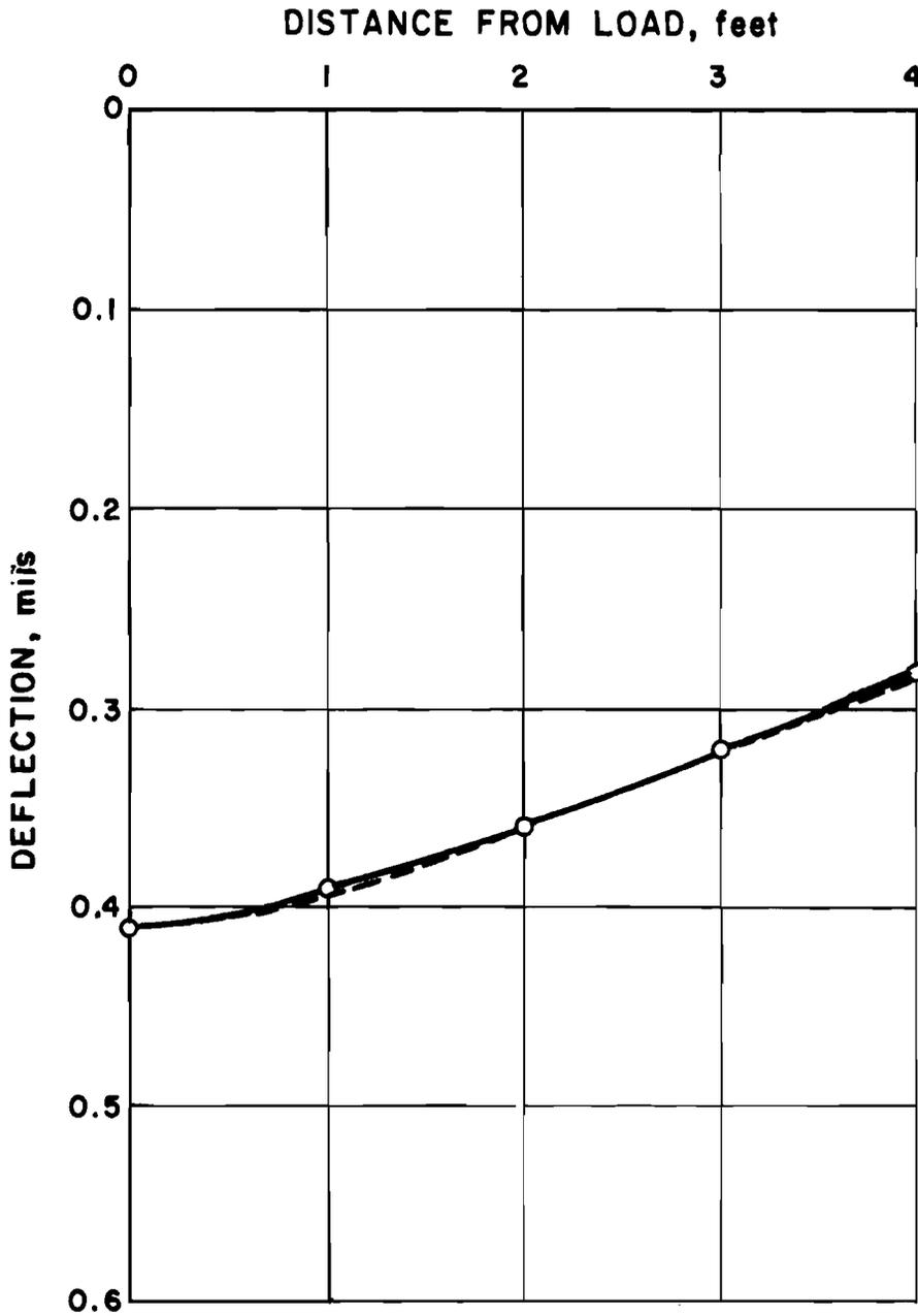
Figure 10f: Observed deflection basin (solid line through circled points) compared with theoretical basin (dashed line) computed from  $E_1(w_1, w_3)$  and  $E_2(w_1, w_3)$  at Test Point 32. Moduli are given in Table 10.
