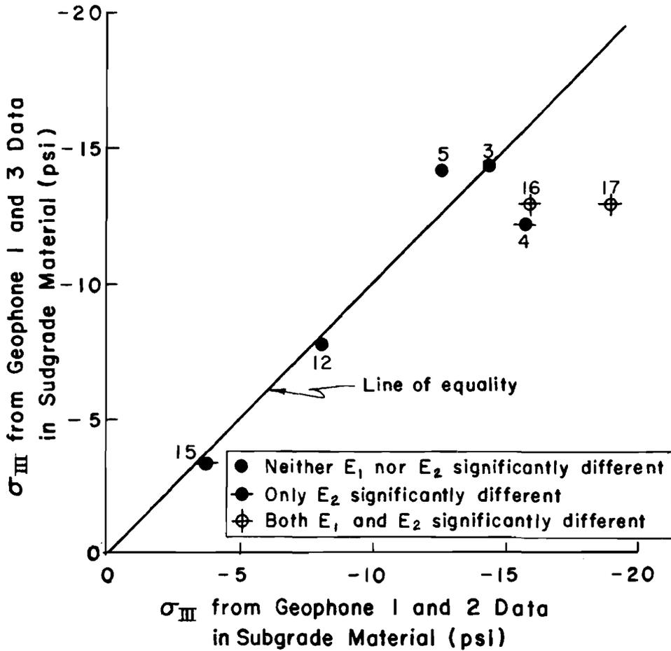
Figure 9: Comparison of the minor principal stresses in the subgrade at the point  $x = 0, y = 0, z = h$ , as computed from data from different pairs of geophones. Significance data from Tables 7 and 8.
