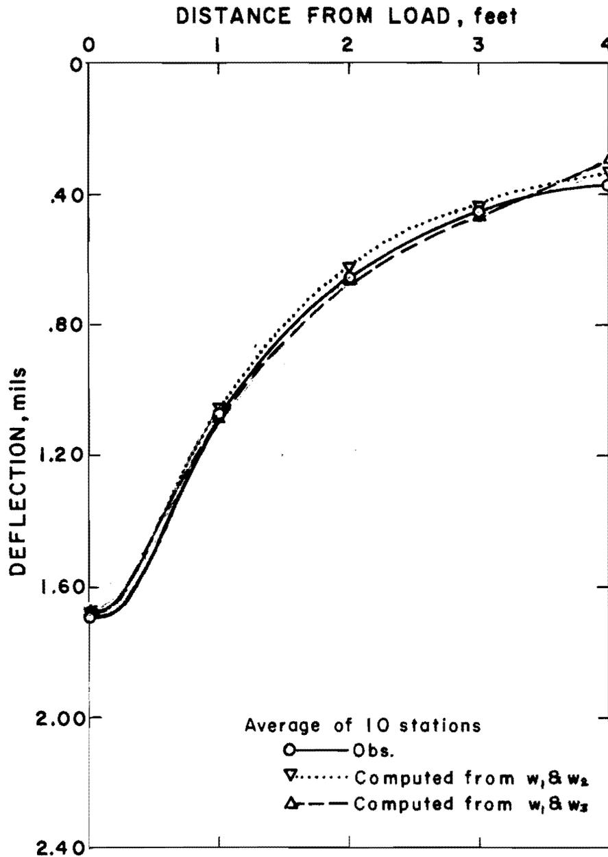
Figure 5d: Computed and average observed Dynaflect deflection basins, Section 12.  $E_1(w_1, w_2) \approx E_1(w_1, w_3)$  and  $E_2(w_1, w_2) \approx E_2(w_1, w_3)$  by statistical test.
