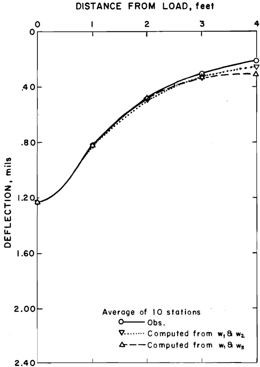
Figure 5a: Computed and average observed Dynaflect deflection basins, Section 3.  $E_1(w_1, w_2) \approx E_1(w_1, w_3)$  and  $E_2(w_1, w_2) \approx E_2(w_1, w_3)$  by statistical test.
