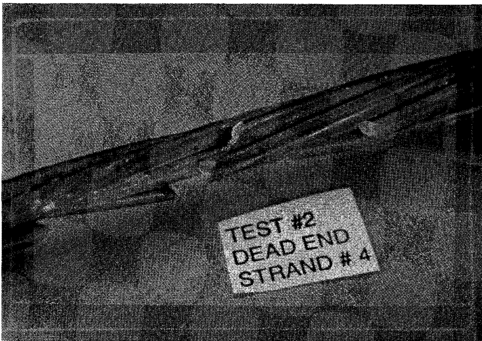
Figure 4.19 Example of Test #2 fracture surfaces.
