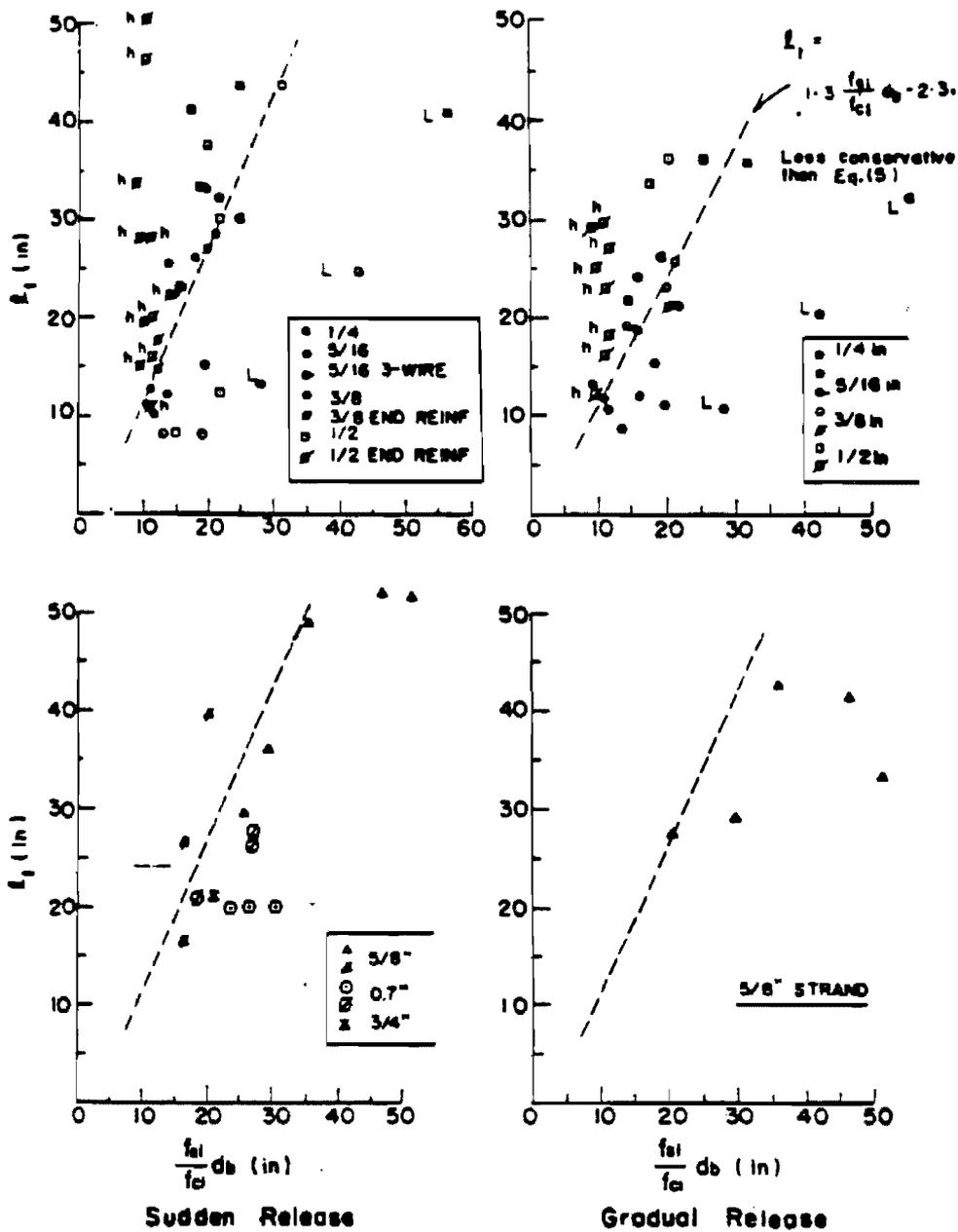
Figure 2.7 Comparison of the Zia-Mostafa equation with experimental results from various sources<sup>(12)</sup>.
