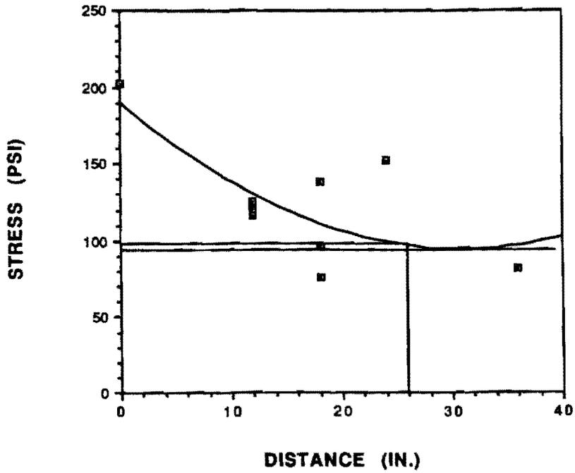
**0.6 INCH FULLY BONDED STRAND-STEEL STRESSES**
