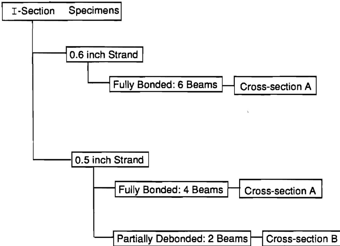
Figure 3.4 Details of I-Section Specimens.
