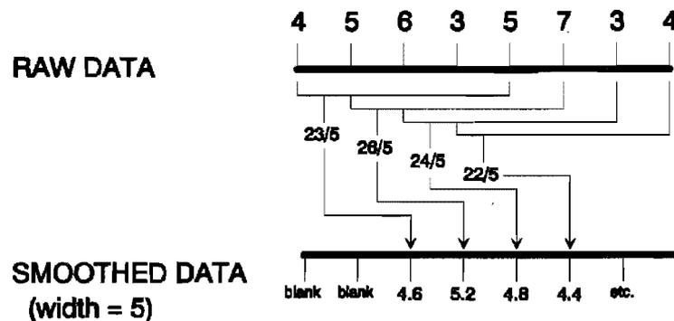
Figure 4.1 Schematic showing smoothing techniques on Cricket Graph using width = 5 (for analysis of concrete strains width = 3 is used)<sup>(23)</sup>.
