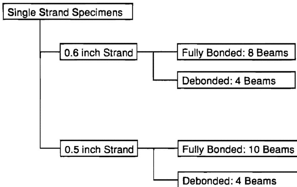
Figure 3.1 Details of single-strand specimens.
