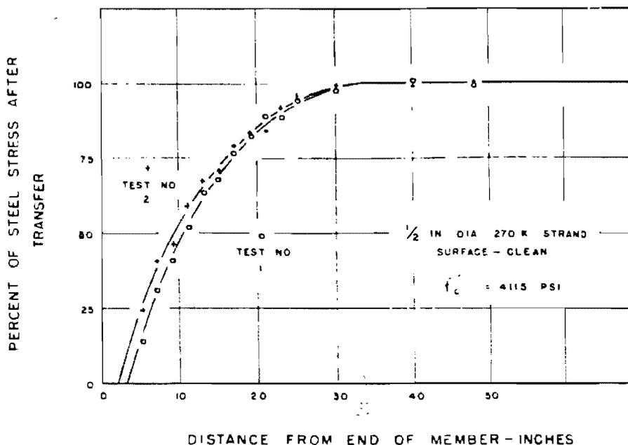
Figure 2.6 Steel stress profile of 0.5-inch diameter Grade 270K strand<sup>(7)</sup>.
