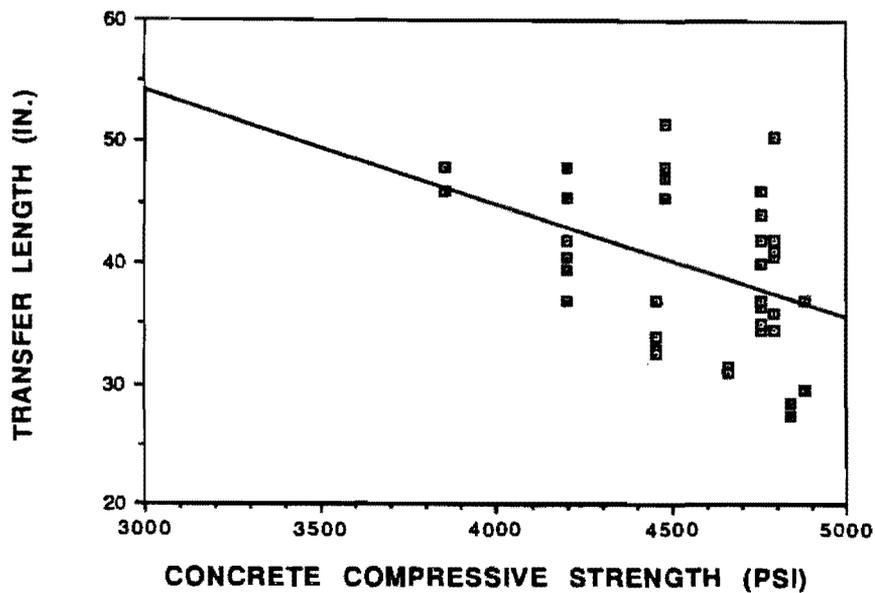
Figure 5.2 Measured transfer length vs. concrete compressive strength, 0.6-inch diameter strand.
