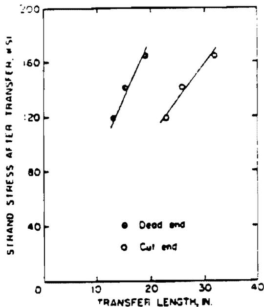
Figure 2.5 Effect of strand tension on transfer length specimens prestressed with 3/8-inch diameter strand<sup>(6)</sup>.
