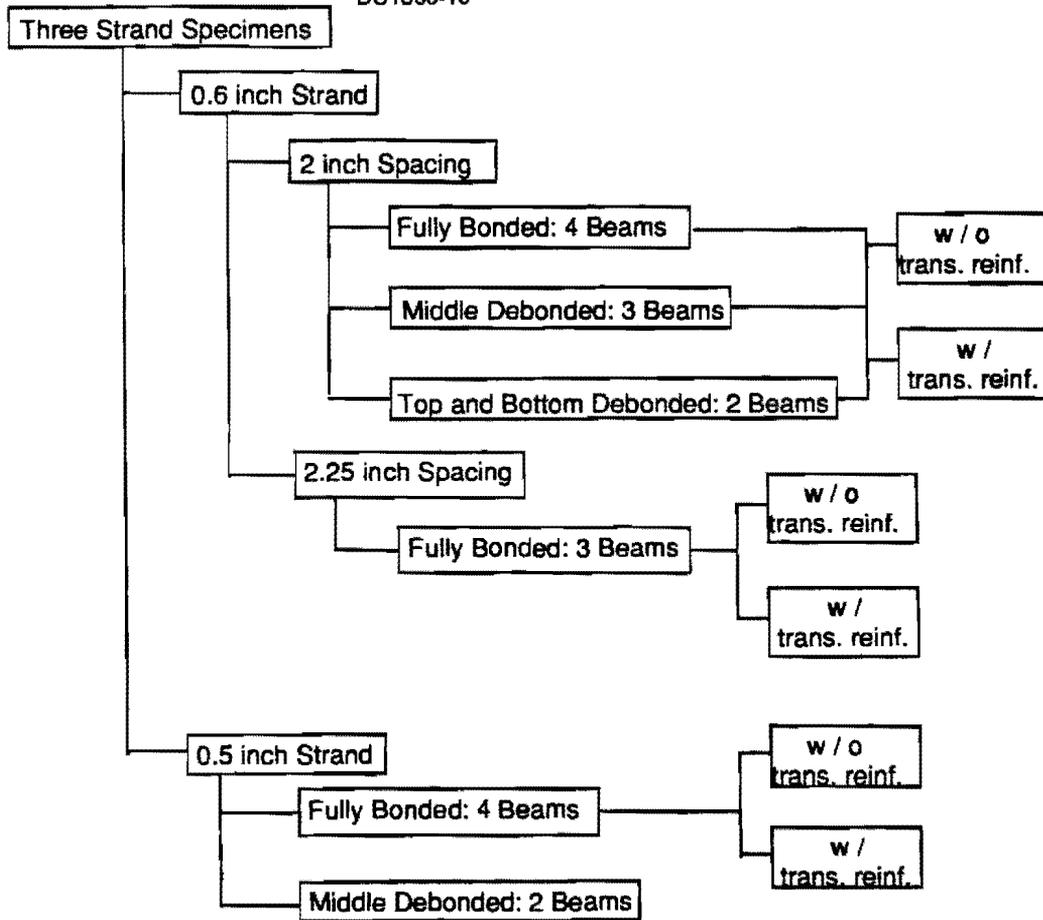
Figure 3.2 Details of three-strand specimens.
