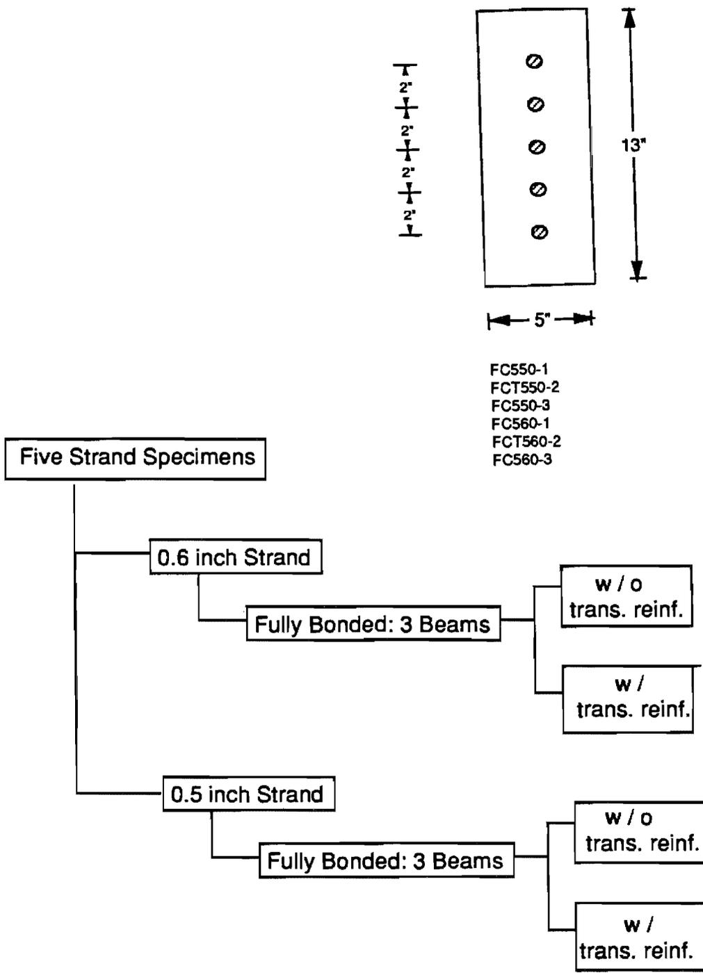
Figure 3.3 Details of five-strand specimens.
