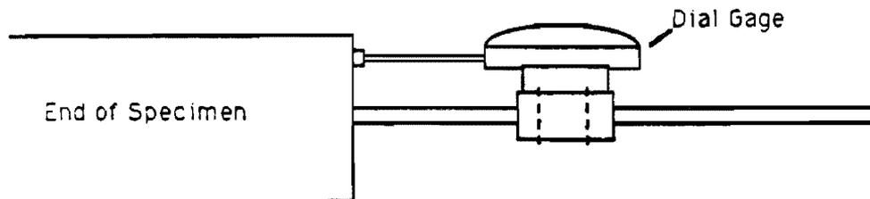
Figure 3.6 End slip device.
