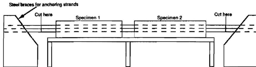
Figure 3.5 Test setup (figure not drawn to scale).
