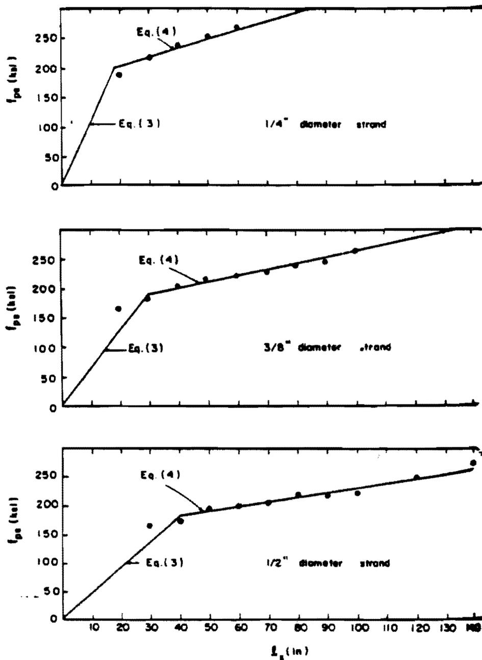
Figure 2.8 Comparison of the Martin-Scott Equations with test results by Hanson and Kaar<sup>(10)</sup>.
