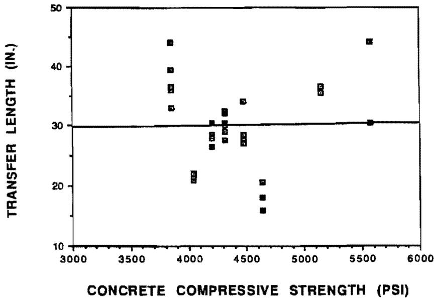
Figure 5.1 Measured transfer length vs. concrete compressive strength, 0.5-inch diameter strand.
