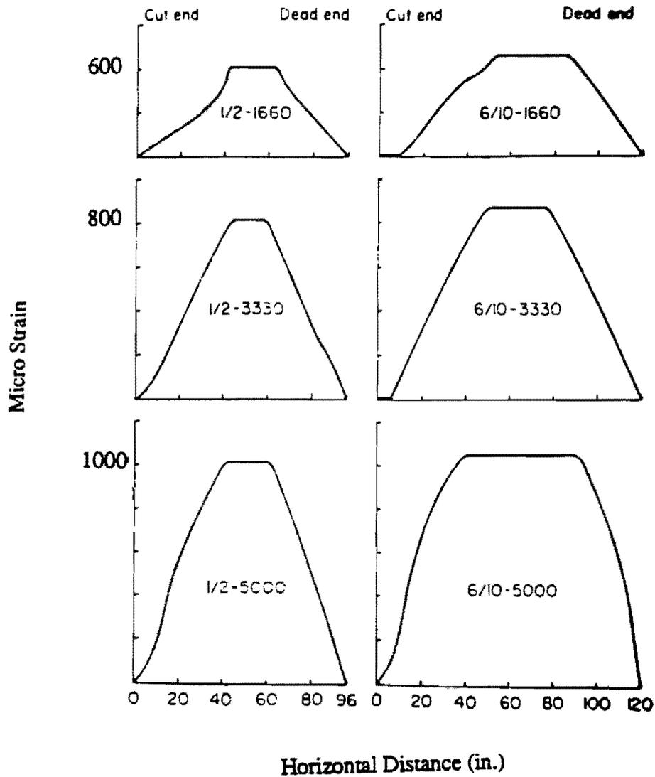
Figure 2.4 Effect of concrete strength at transfer on transfer length of 0.5-inch and 0.6-inch diameter strand<sup>(6)</sup>.
