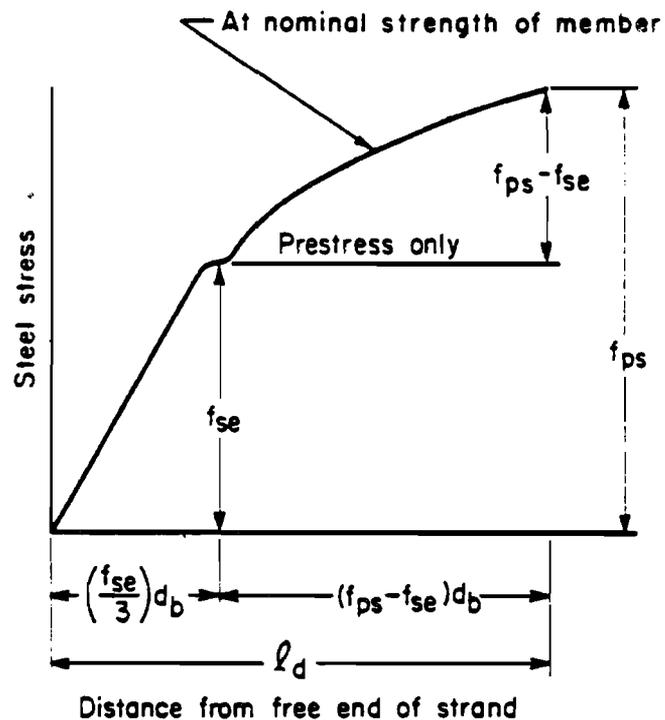
Figure 2.1 Variation of steel stress with distance from free end of strand. Used as the basis for ACI/AASHTO formula<sup>(21,22)</sup>.
