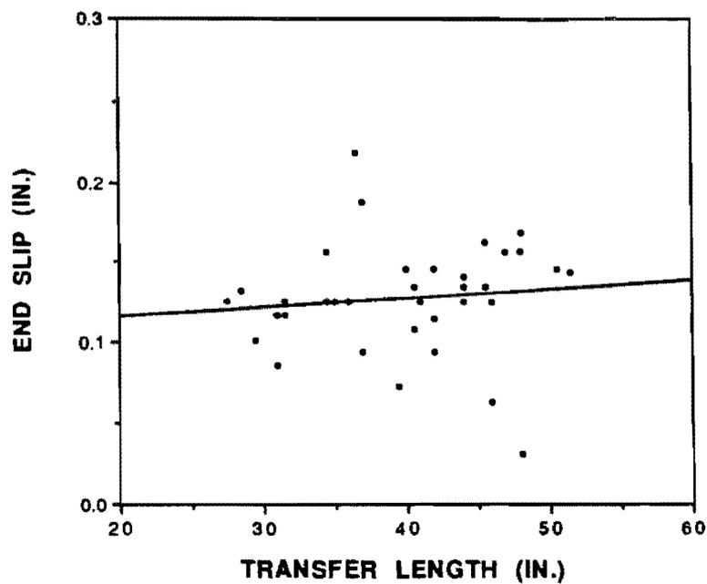
Figure 5.4 Measured transfer length vs. end slip, 0.6-inch diameter strand.
