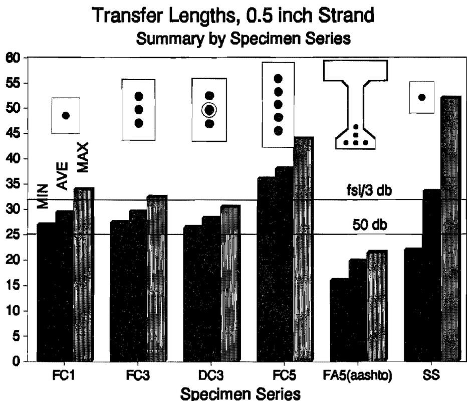
Figure 4.5 Measured transfer length, 0.5-inch fully bonded strand (minimum, mean and maximum values compared with ACI required value).
