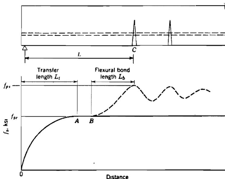
Figure 2.2 Flexural bond overlapping with transfer length<sup>(15)</sup>.
