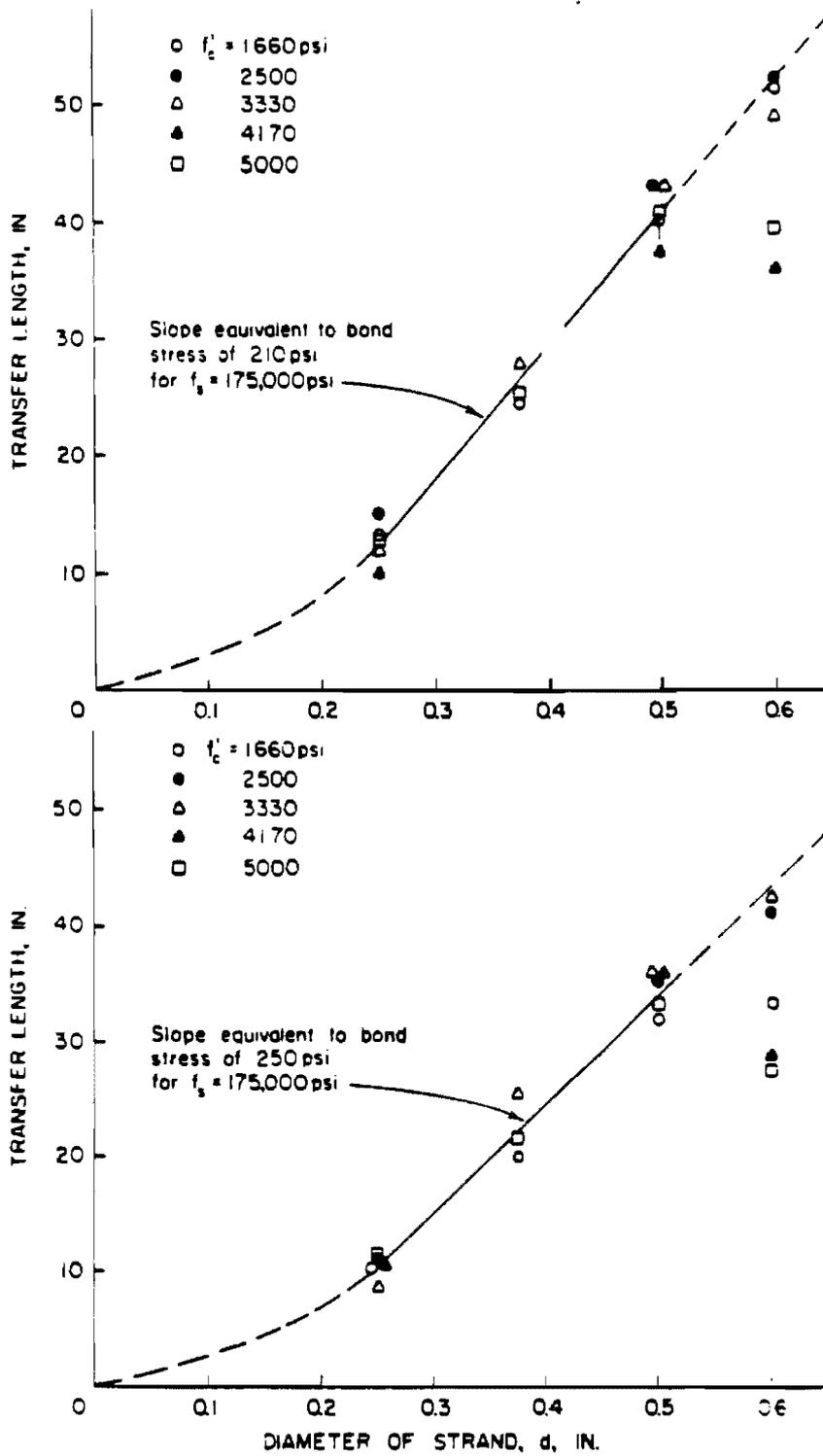
Figure 2.3 Relation of prestress transfer length to strand diameter at a) cut end and b) dead end<sup>(6)</sup>.
