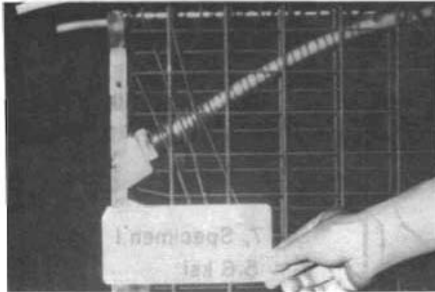
Fig. 5.26(a) Set 7, Specimen 1 before casting showing long spiral reinforcement
