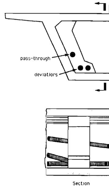
Figure 1.6 Typical shape for rib deviator (adapted from Ref. 2).
