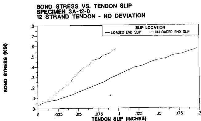
Figure 3.27 Bond Stress-Slip Response for Specimen 3A-12-0°.
