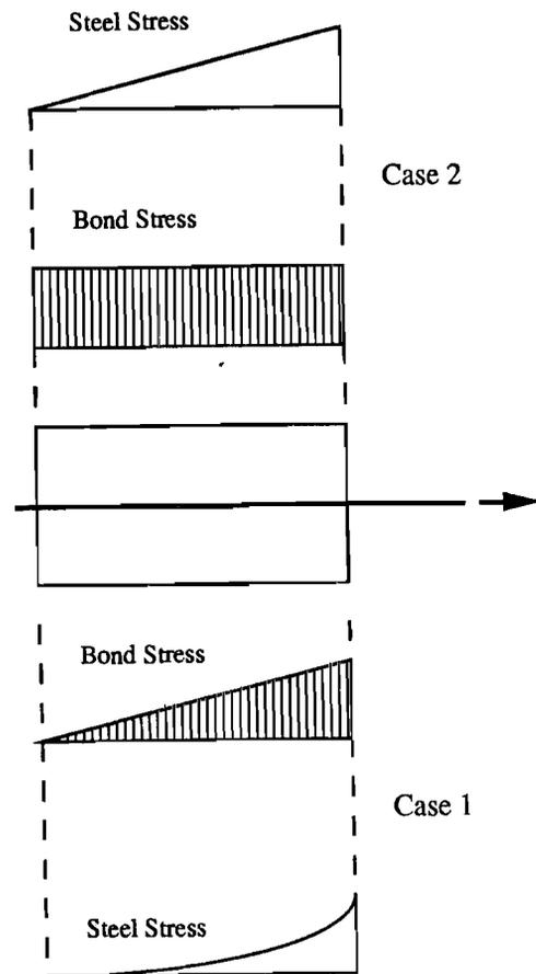
Figure 2.7 Bond and steel stress distributions along bonded length.
