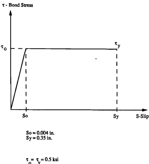
Figure 4.14 Proposed Bond-Slip Relationship for Grouted Multi-Strand Tendons in Smooth Steel Ducts.
