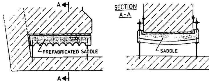
Figure 1.8 Prefabricated saddle block (from Ref. 8).
