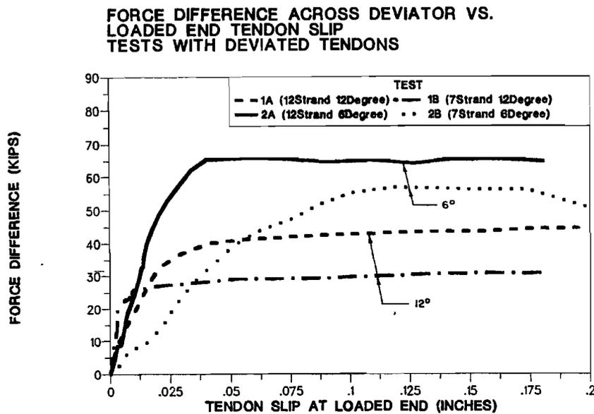
Figure 4.2 Pullout Force -Slip Performance of Specimens with Deviated Tendons.
