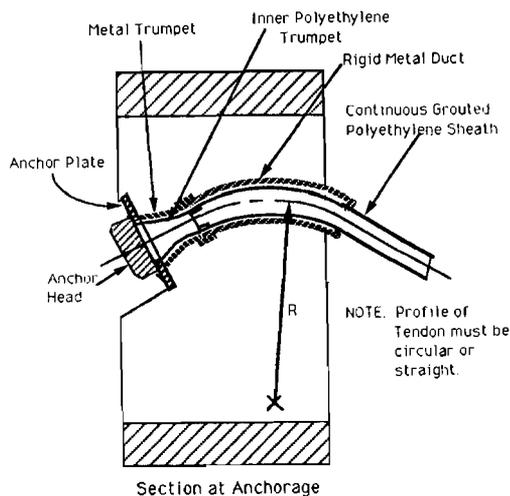
Figure 1.10 "Double duct" for replaceable tendons (from Ref. 2).
