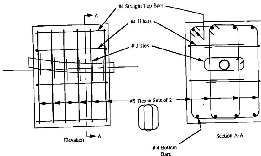
Figure 3.2 Deviator Block Reinforcement Details.
