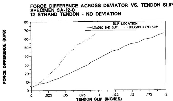
Figure 3.28 Pullout Force-Slip Response for Specimen 3A-12-0°.
