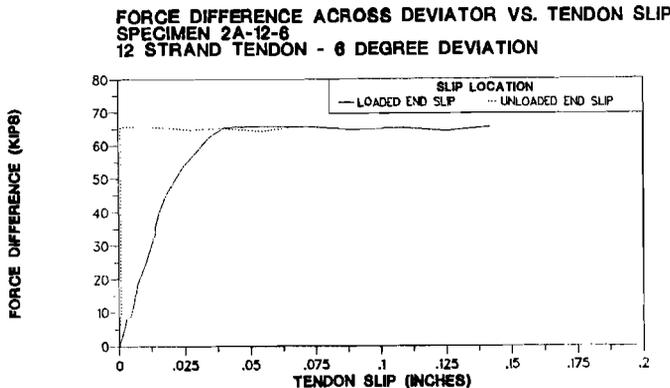
Figure 3.24 Pullout Force-Slip Response for Specimen 2A-12-6°.
