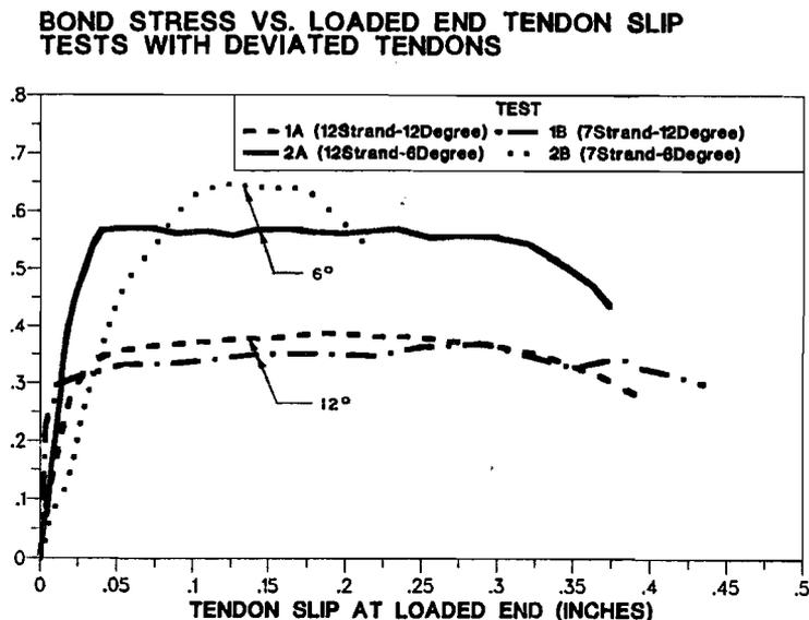
Figure 4.3 Bond Stress-Slip Performance of Specimens with Deviated Tendons.
