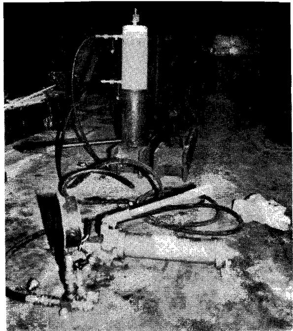
Figure 3.8 Post-Tensioning Anchor Bolts for South Reaction Frame.
