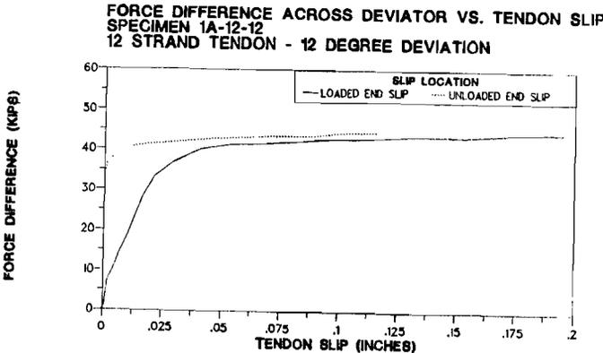
Figure 3.20 Pullout Force-Slip Response for Specimen 1A-12-12°.
