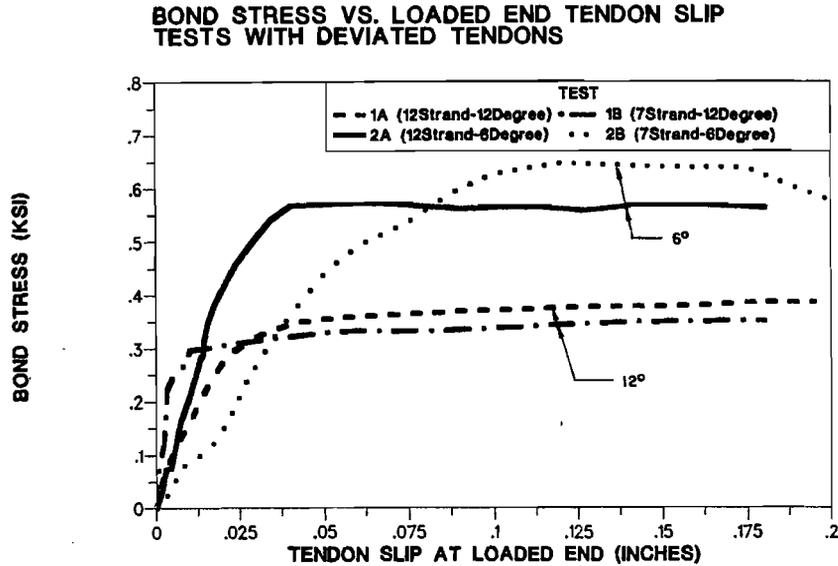
Figure 4.1 Bond Stress-Slip Performance of Specimens with Deviated Tendons.
