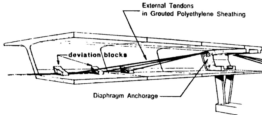
Figure 1.1 External post-tensioning in Long Key Bridge (from Ref. 3).
