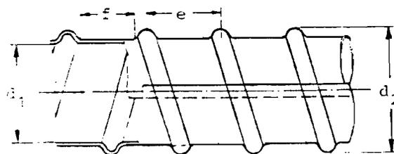
Figure 2.18 Steel duct detail for tests by Trost (from REf. 17).
