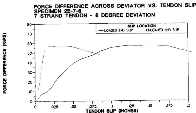
Figure 3.26 Pullout Force-Slip Response for Specimen 2B-7-6°.
