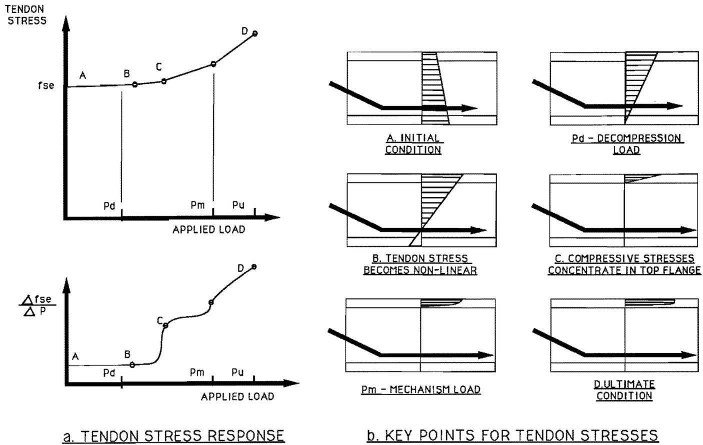
Figure 2.1 Tendon Stress Response to Applied Load (From Ref. 3)
