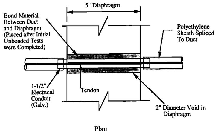
Figure 3.37 Duct-Deviator Detail in Bridge Model.
