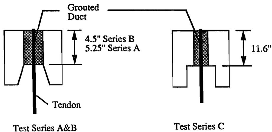
Figure 2.17 Pullout specimens tested by Trost (from Ref. 17).
