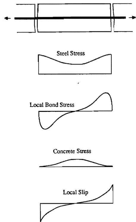
Figure 2.2 Distribution of stress and local slip along cracked element.
