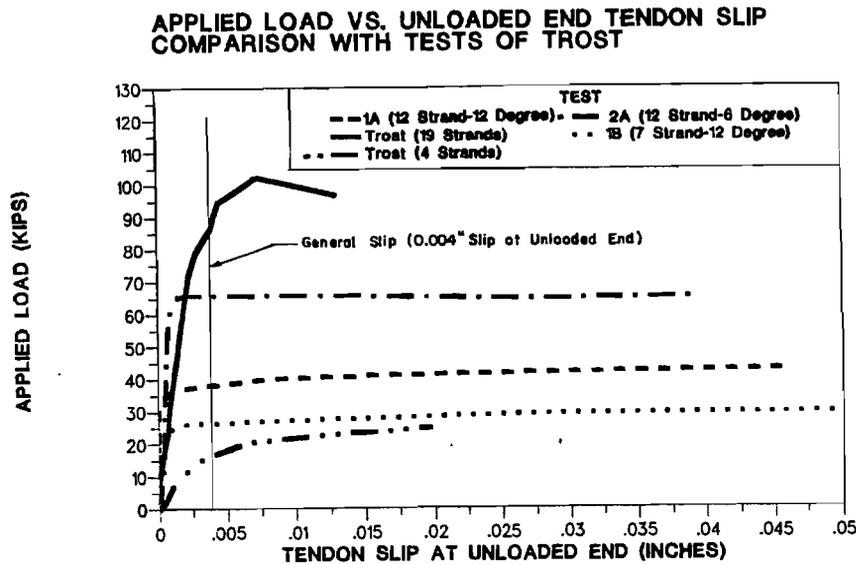
Figure 4.13 Comparison of Tendon Slip Values at Unloaded End.
