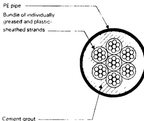
Figure 1.12 Tendon consisting of HDPE sheathed monostrands, grouted before stressing (from Ref. 8).
