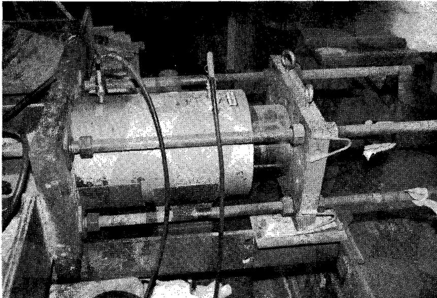
Figure 3.6 500-Ton Stressing Ram at South End of Bed.
