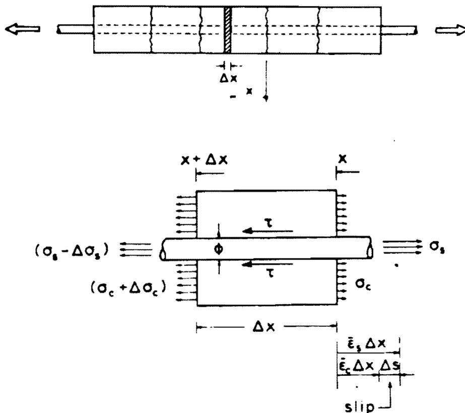
Figure 2.4 Strand slip due to differential strain (from Ref. 20).
