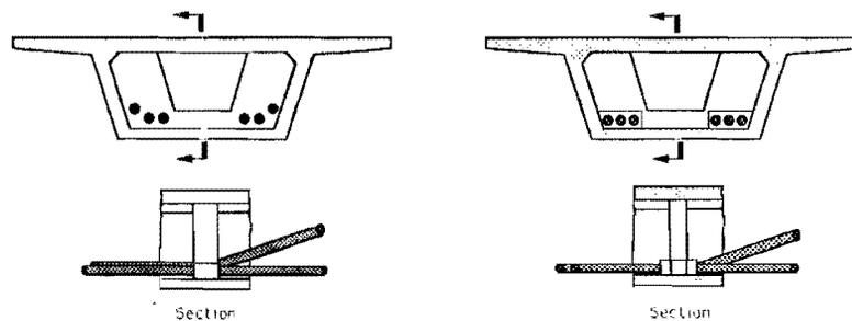
Figure 1.5 Typical shapes for diaphragm deviators (from Ref. 2).
