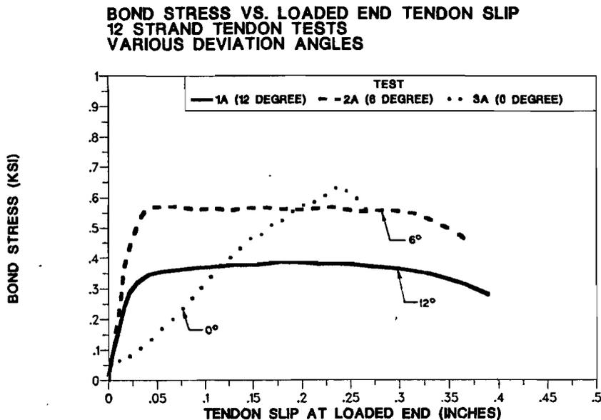
Figure 4.8 Bond Stress-Slip Performance of 12-Strand Tendon Specimens with 0, 6, and 12 Degree Deviations.
