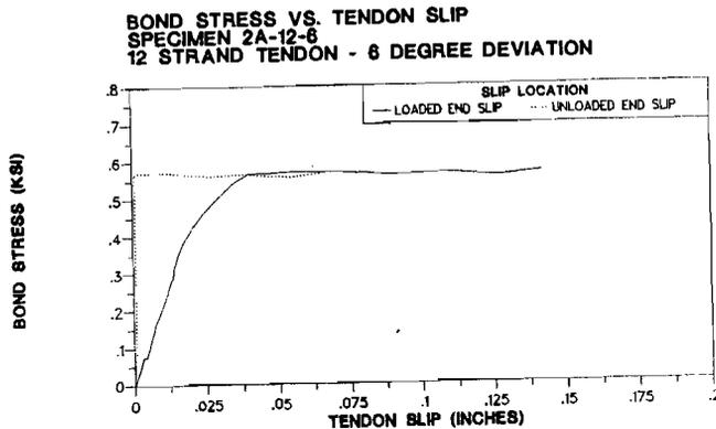
Figure 3.23 Bond Stress-Slip Response for Specimen 2A-12-6°.
