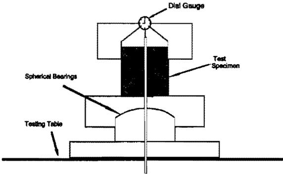
Test Setup for Pullout Test
