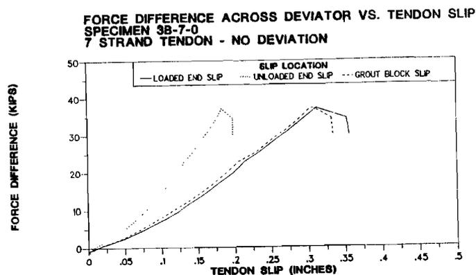
Figure 3.30 Pullout Force-Slip Response for Specimen 3B-7-0°.
