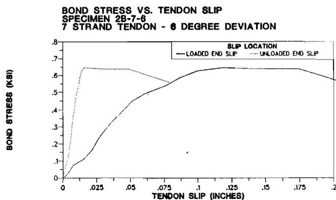
Figure 3.25 Bond Stress-Slip Response for Specimen 2B-7-6°.
