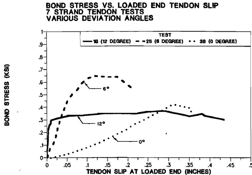
Figure 4.9 Bond Stress-Slip Performance of 7-Strand Tendon Specimens with 0, 6, and 12 Degree Deviations.
