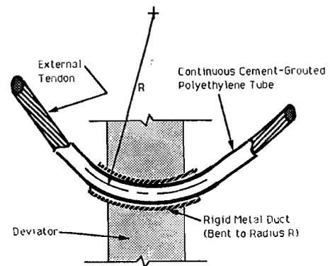
Figure 1.11 "Double duct" configuration at deviators (from Ref. 2).
