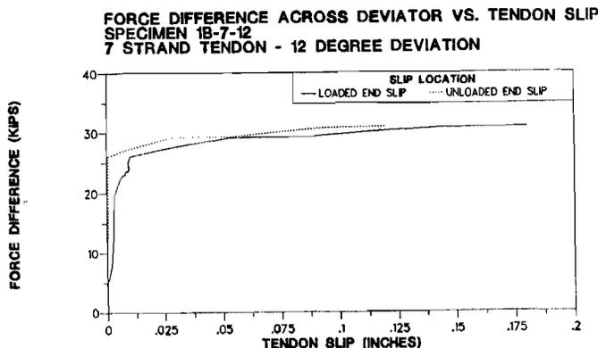
Figure 3.22 Pullout Force-Slip Response for Specimen 1B-7-12<sup>o</sup>.
