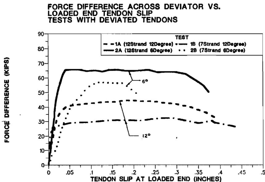
Figure 4.4 Pullout Force-Slip Performance of Specimens with Deviated Tendons.
