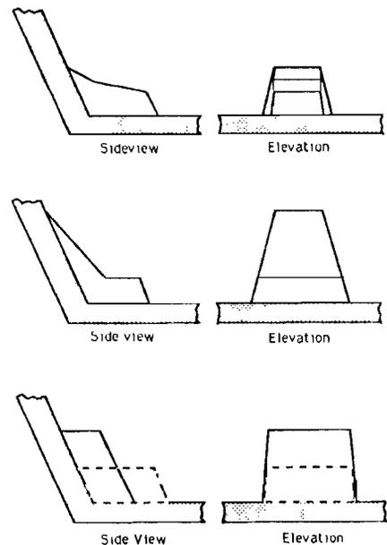
Figure 1.7 Typical shapes for deviator blocks (from Ref. 2).
