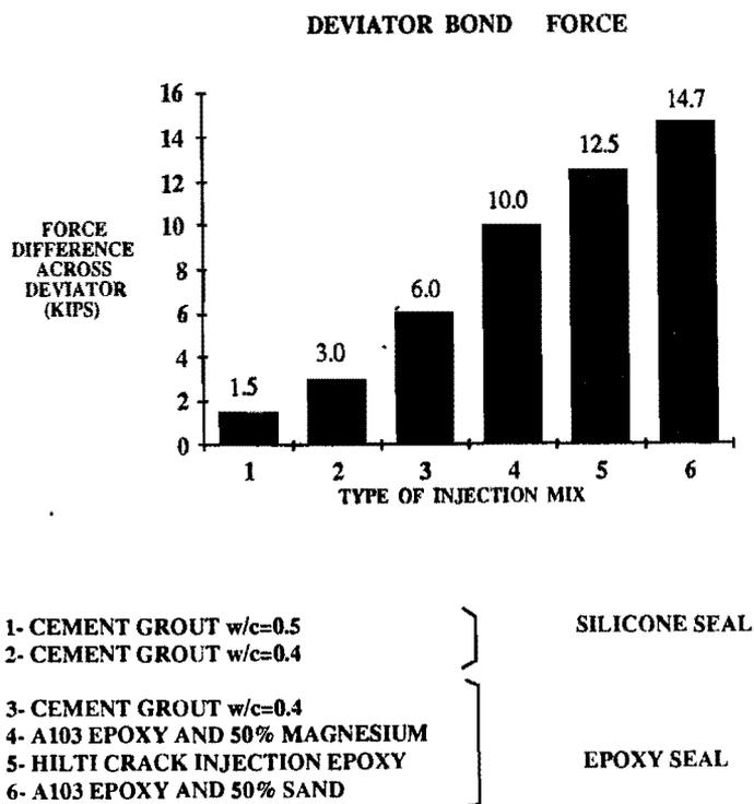
Figure 3.39 Bond Specimen Test Results.
