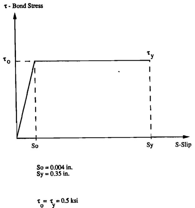
Figure 5.1 Proposed Bond-Slip Relationship for Grouted Multi-Strand Tendons in Smooth Steel Ducts.
