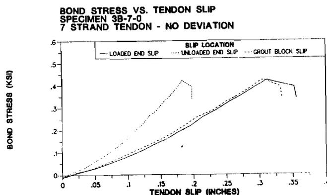
Figure 3.29 Bond Stress-Slip Response for Specimen 3B-7-0°.
