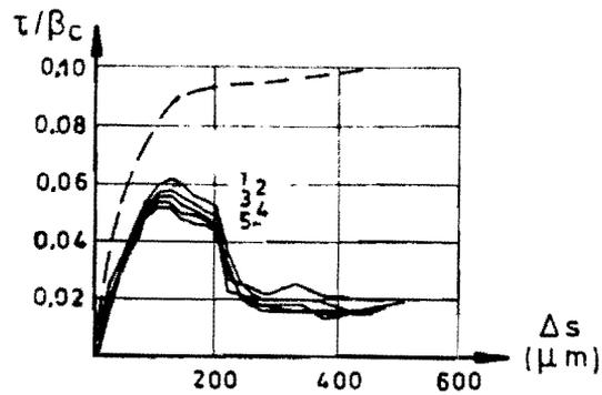
Test Series B-9 (4-0.6" Strands in the Middle of the Duct)
