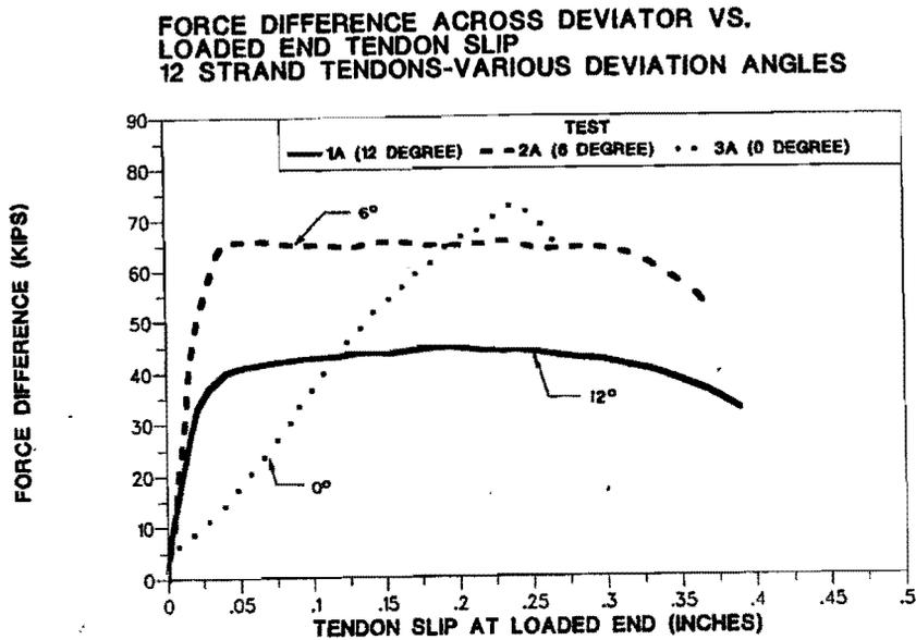
Figure 4.10 Pullout Force-Slip Performance of 12-Strand Tendon Specimens with 0, 6, and 12 Degree Deviations.
