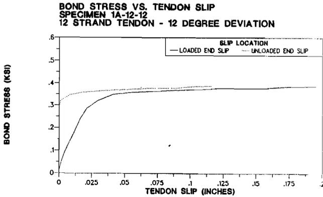
Figure 3.19 Bond Stress-Slip Response for Specimen 1A-12-12°.
