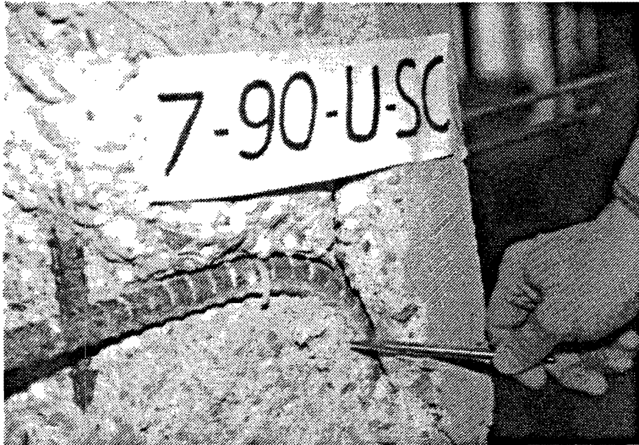
(a) Uncoated bar specimen
