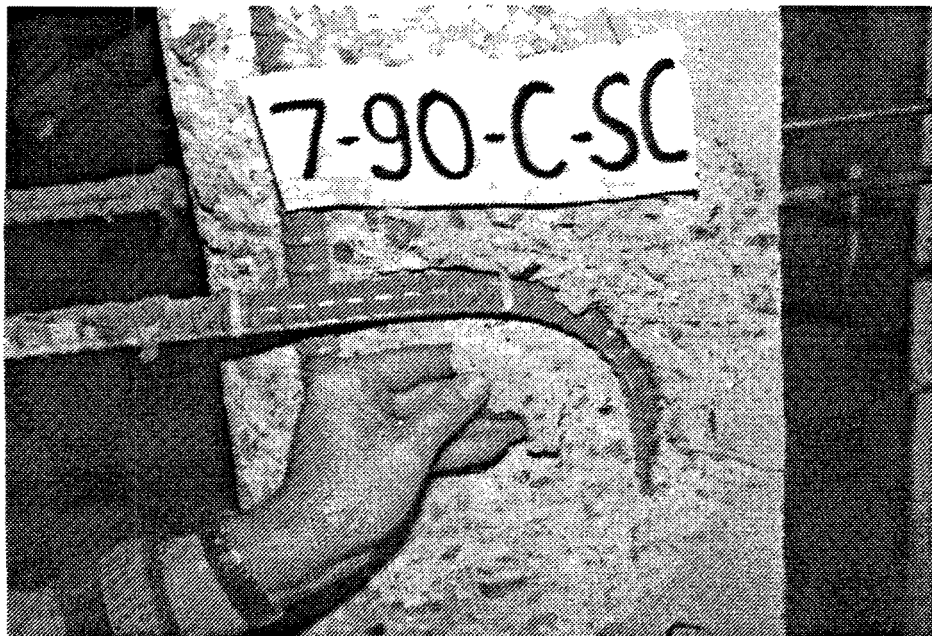
(b) Epoxy-coated bar specimen
