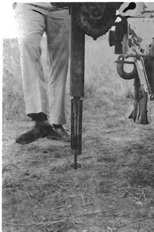
(a) Method of driving heave points and psychrometer access tubes.
