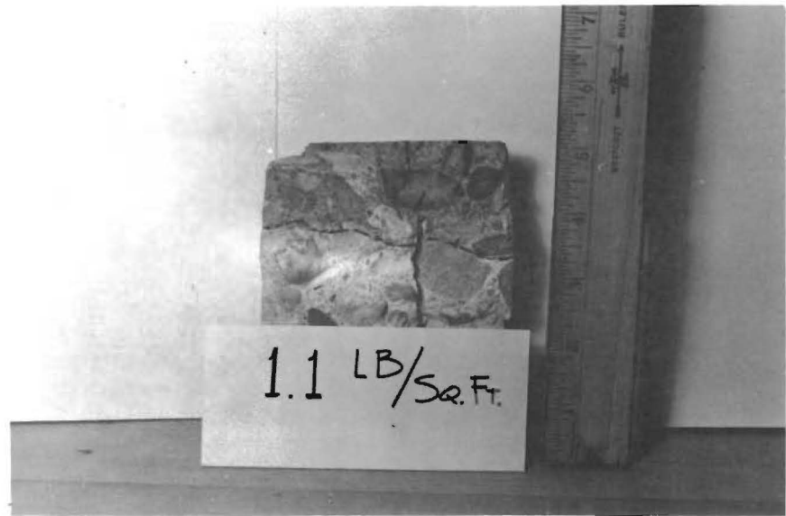
Fig. 5.4 Photographs of Cores from Areas of Different Monomer Application Rates
