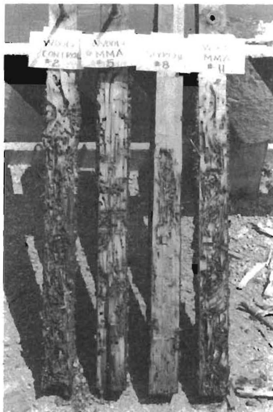
FIG. 6.2 COMPARISON OF TREATED AND UNTREATED WOOD PILES AFTER 7 MONTHS EXPOSURE
