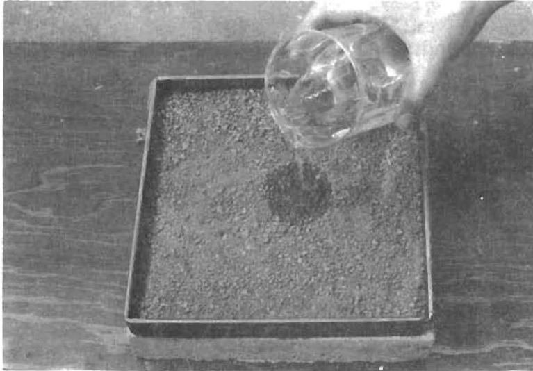
FIG. 3.1 APPLICATION OF MONOMER TO 2 IN. SLAB COVERED WITH FINE AGGREGATE
