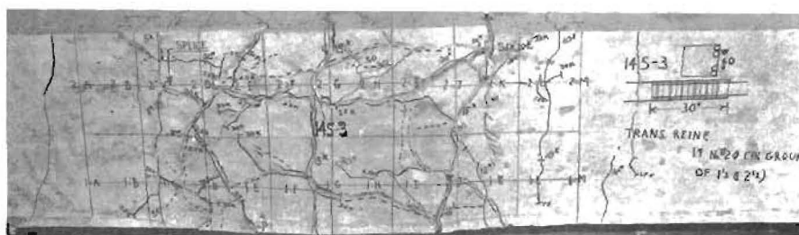
(b) Failure #14 splice with 19 #2 U in L_s = 30 in.
