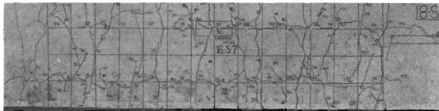
(d) Tension face. Note lower bar is continuous.
