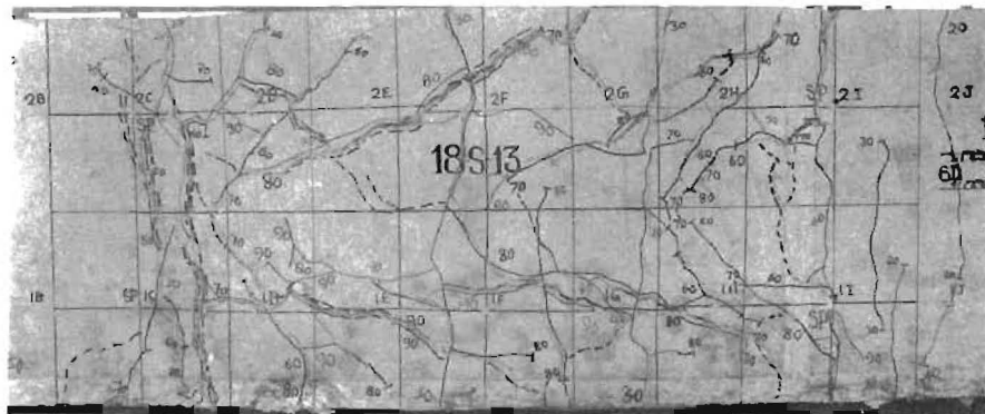
(b) Tension face cracking.
