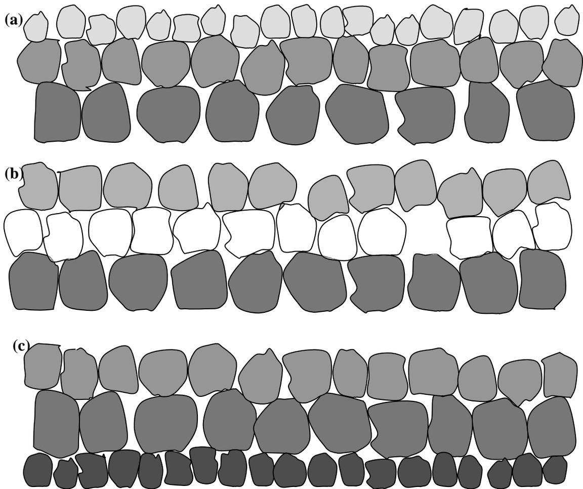
Figure 3.6 Aggregate Grade Combinations Used in 3-CST (a) Grade 5 on Grade 4 on Grade 3 (b) Grade 4 on Grade 4 on Grade 3 (c) Grade 4 on Grade 3 on Grade 5.
