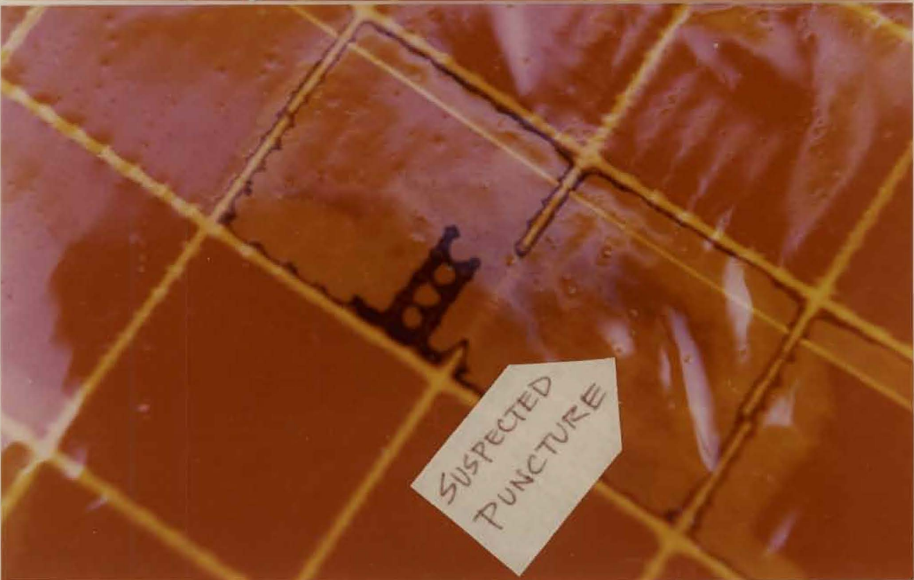
Picture 2 - Result of torn reflective sheeting of flexible roll-up sign
