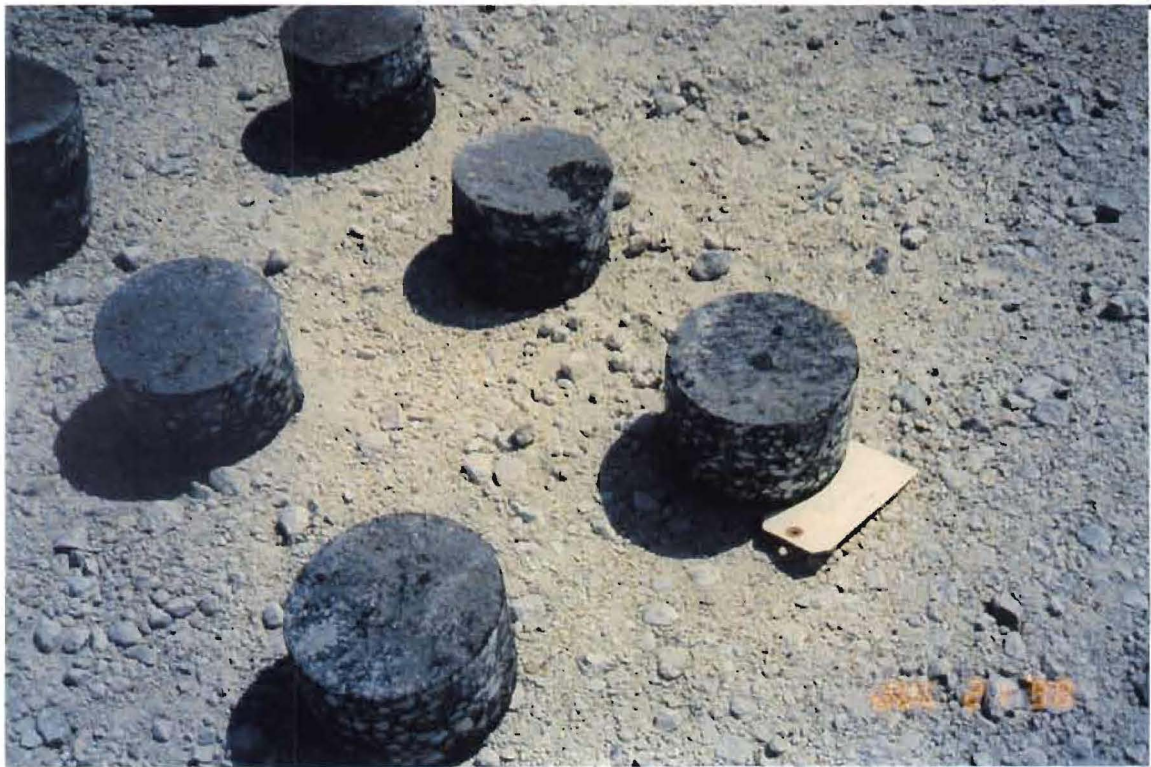
Photos showing the difference in surface texture one month after treatment. (Reclamite)
