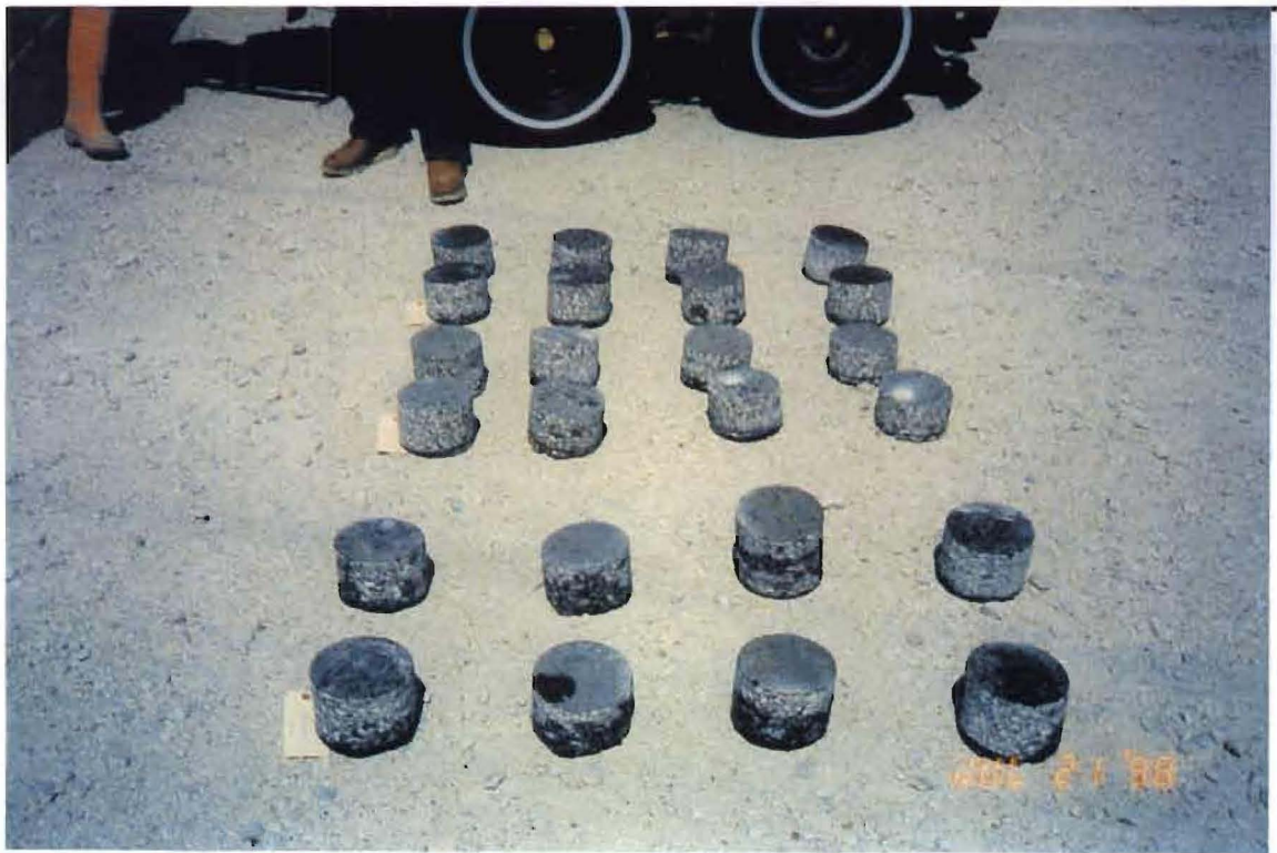
Photos showing the difference in surface texture one month after treatment. (CRF – back; Untreated – middle; Reclamite – front)
