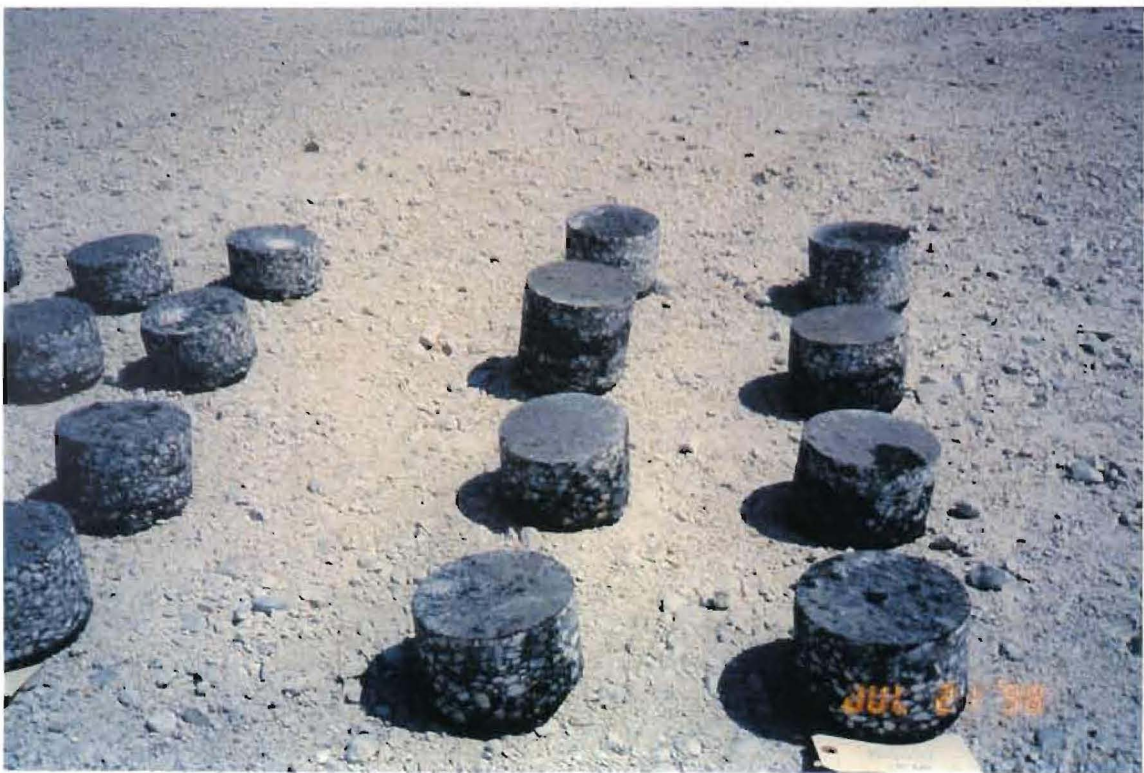
Photos showing the difference in surface texture one month after treatment. (Reclamite – right; Untreated – left)
