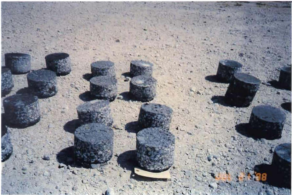
Photos showing the difference in surface texture one month after treatment. (CRF – left; Untreated – middle; Reclamite - right)
