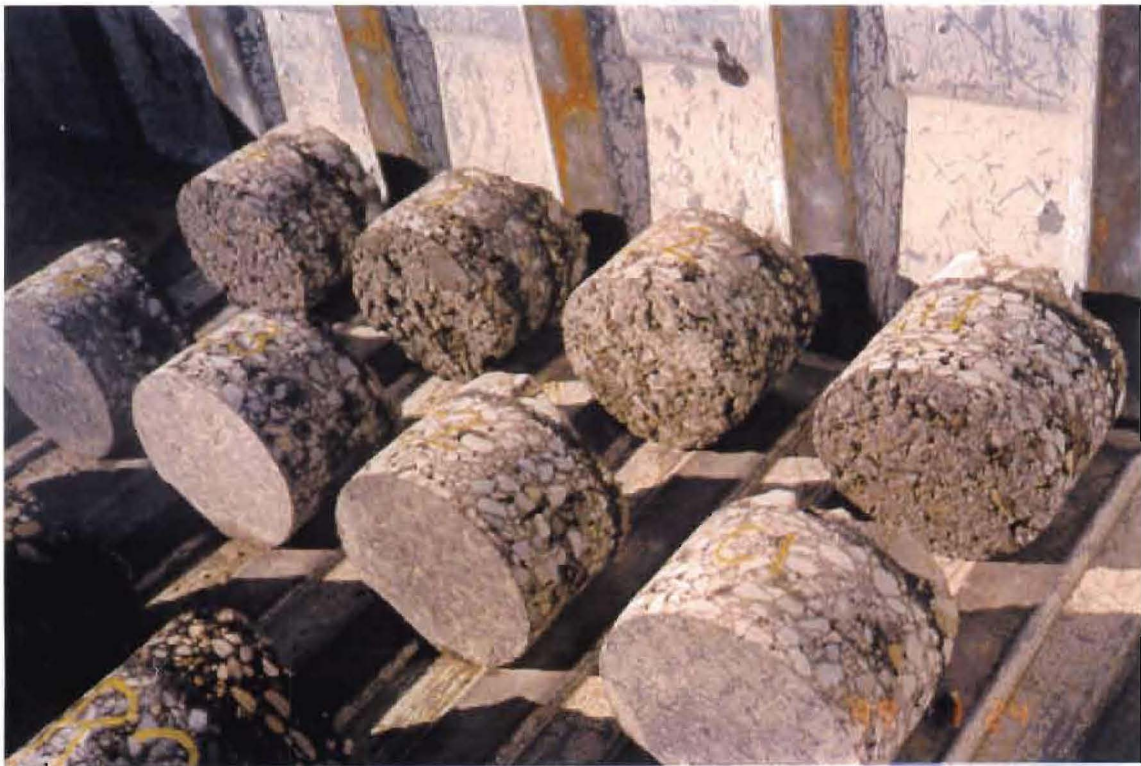
Photos showing the difference in surface texture six months after treatment (untreated - back; CRF - middle; Reclamite - front)
