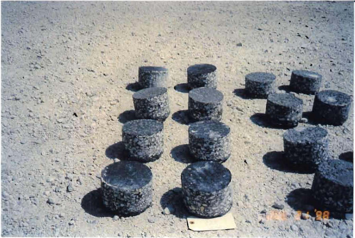
Photos showing the difference in surface texture one month after treatment. (CRF - left; Untreated -right)
