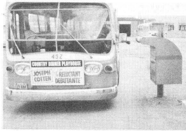
DRIVER DROPS DEFECT CARD INTO COLLECTION BOX AFTER EACH RUN.
