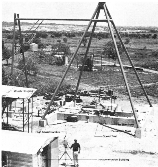
Figure 2. SwRI pendulum impact tester.
