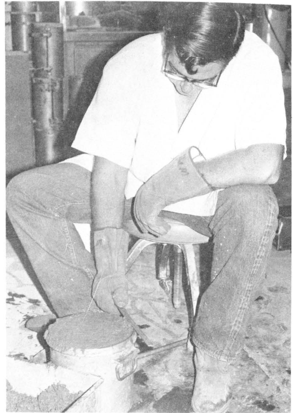
Figure 8 The unit weight and air content are tested by standard procedures. It was noted that wire fibers do flip off the edges during screeding, so safety precautions are necessary.
