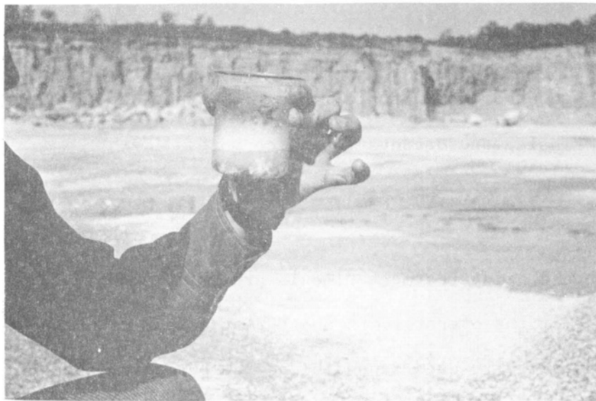
Fig. 4. Reaction of a limestone aggregate to the hydrochloric acid treatment. Note darker organic residue floating to the top of the foam.
