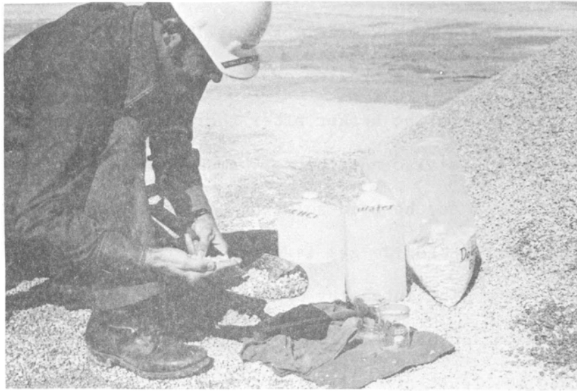
Fig. 3. Removing about 50 g of representative aggregate for placement in beaker and acid treatment.
