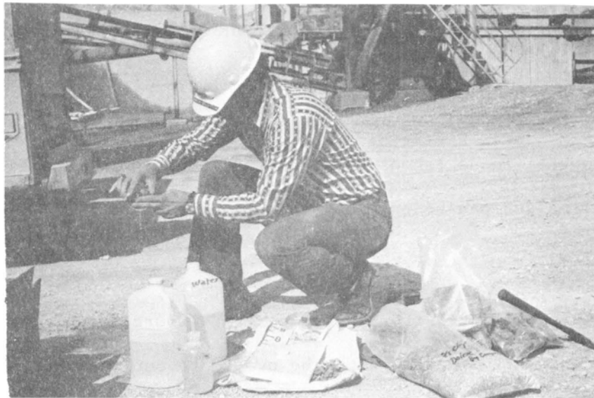
Fig. 6. Rinsing and decanting the acid-treated sample.
