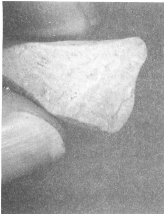
Figs. 8 and 9. View of two carbonate aggregate particles which have been acid treated for 20 seconds. Sample on left is a relatively high-purity limestone which exhibits a very smooth surface texture, whereas, the particle on the right is an impure, sandy limestone showing a high degree of surface texture.
