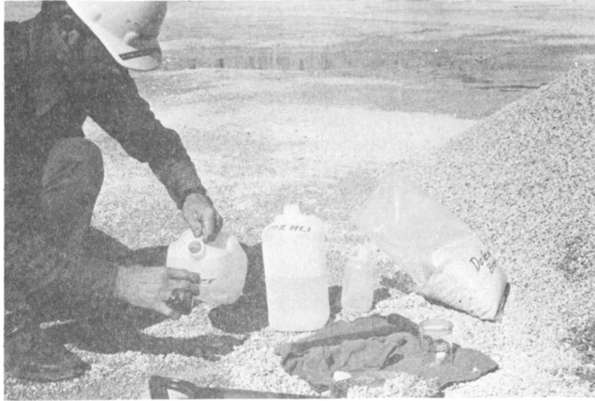
Fig. 5. Flushing and rinsing the acid-treated aggregate sample with water.
