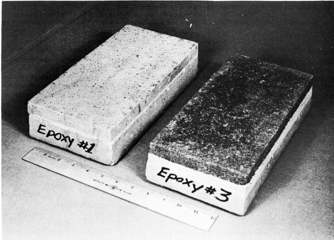
Figure 3 Composite Blocks Used in Freeze-Thaw Test
