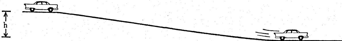
car at rest on a hill PE = weight \times height = ft \text{ lbs}
