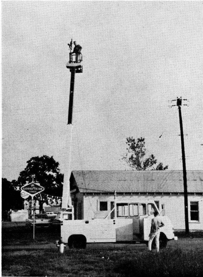
Figure 2. Aerial bucket truck used to elevate cameraman.
