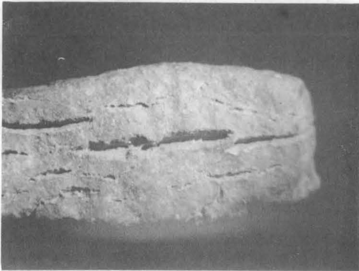
Fig. 2 Pull-apart features formed along or parallel to bedding planes. These features result from preferred directional expansion perpendicular to bedding planes. (Mag. 7.5X)
