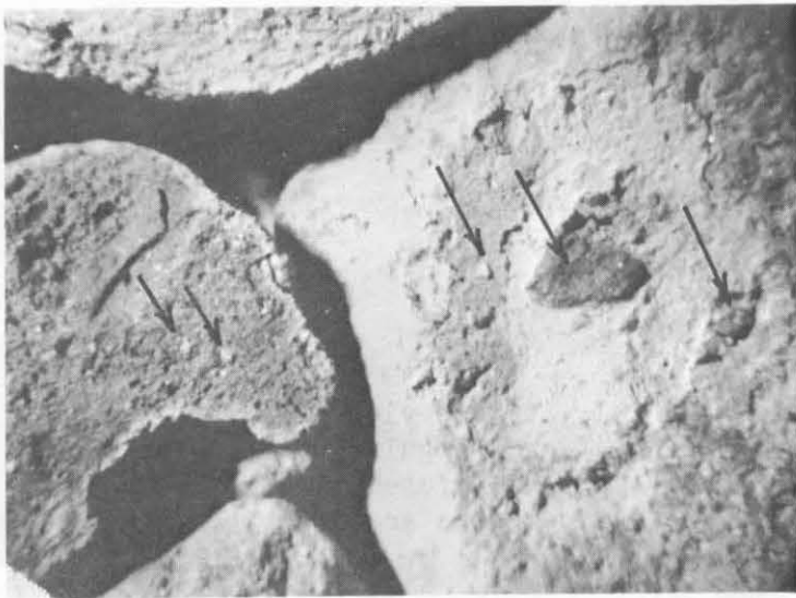
Fig. 3 Particles exhibiting abrasion characteristics after nine hours in the British Polishing Machine. A darker interior color in particle on left can be noted. Sand grains and other mineral inclusions are indicated. (Mag. 7.5X)
