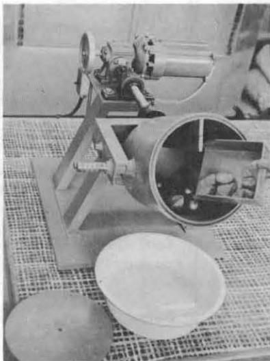
Figure 1a Wet Ball Mill Showing Baffle and Charge
