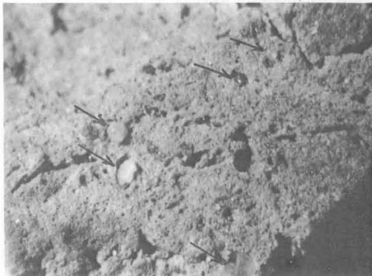
Fig 5 Particle surface after nine hours of polishing showing microvesicular texture formed by trapped gases. Included sand grains are noted. (Mag. 23X)
