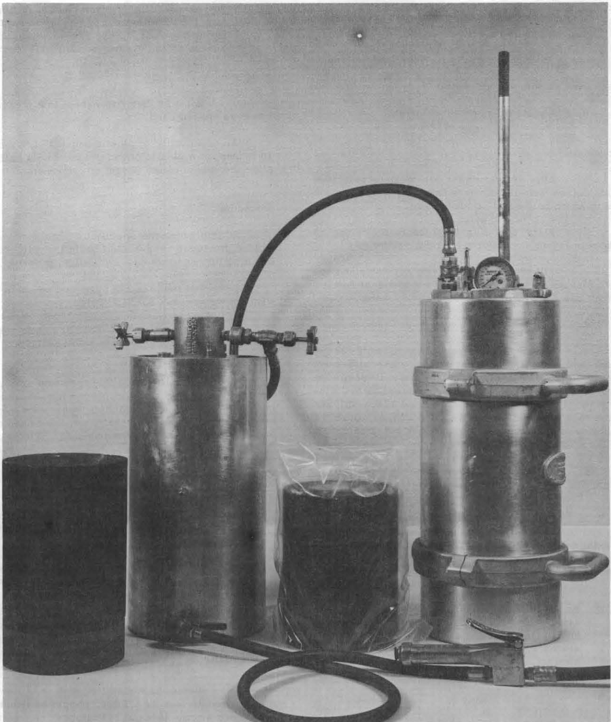
Pycnometer Used as a Pressure Vessel
