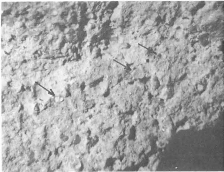
Fig. 4 Particle surface after nine hours of polishing showing irregular surface resulting from irregular wearing rates, protruding sand grains, and cavities left by plucked grains. (Mag. 23X)
