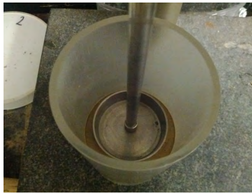
Figure 6: Measurement of Compacted Specimen Using Metal Plate and Mounted Caliper
