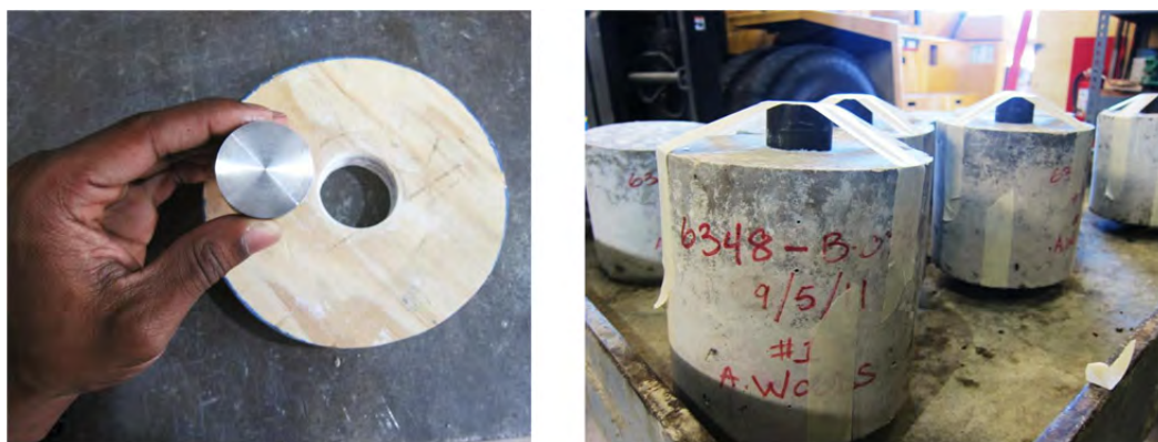
Figure F-69: Steel punch centering guide and masking tape used to secure against eccentric loading effects
