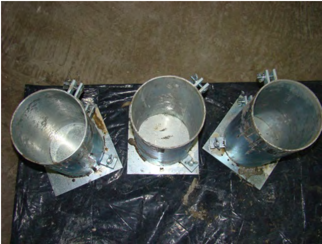
Figure F-9: Steel molds used to prepare specimens in Phase 3 at UT Arlington
