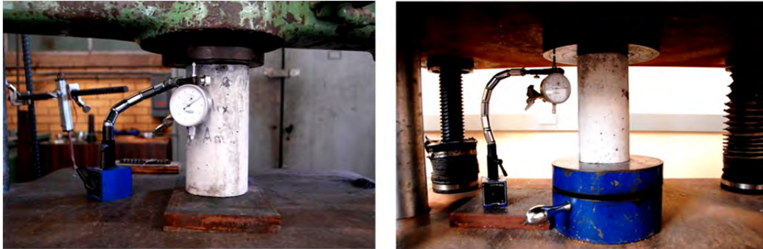
Figure G-11: Calibration setup for Baldwin (left) and Olsen (right) UTMs
