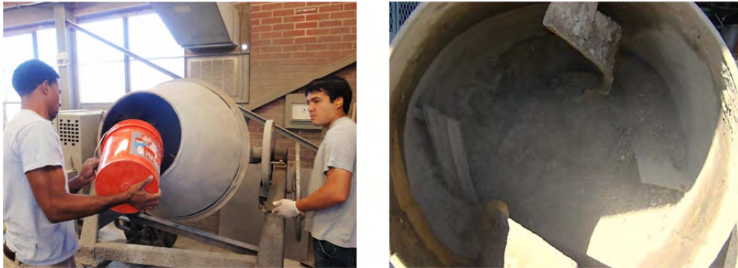
Figure F-52: SFRC mixing sequence, Step 2
