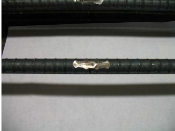
(a) Grind surface of reinforcing bar
