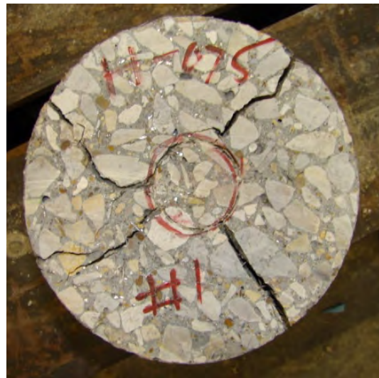
Figure F-12: Typical test specimens with various fiber volume fractions (Phase 4, UT Arlington)
