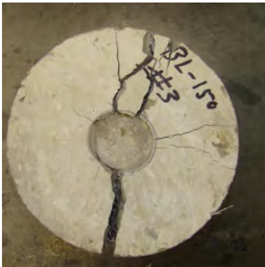
Figure F-12: Typical test specimens with various fiber volume fractions (Phase 4, UT Arlington)
