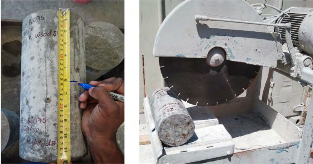
Figure F-60: Using wet-saw to cut 6 x 12-in. cylinder in half
