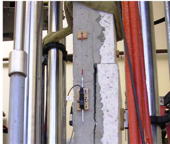
Figure 2-13: Delamination during DTT (Foster 2010)
