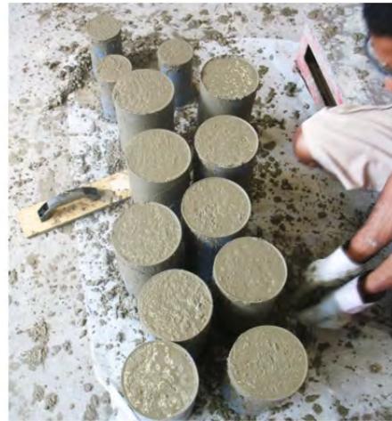
Figure F-58: SFRC mixing sequence, Step 7
