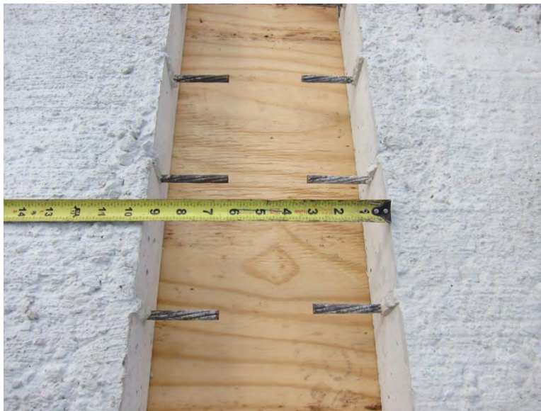
Figure 4-10: Space between PCPs, restrained-shrinkage test
