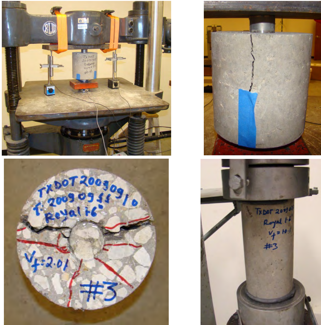
Figure F-7: Typical stages of testing for Phase 1 at UT Arlington (DPT and compressive-strength tests)
