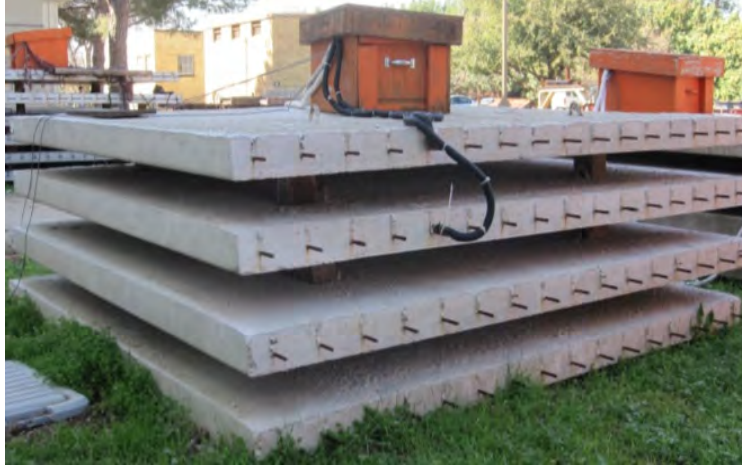
Figure 2-15: Long-term monitoring of prestress loss in PCPs
