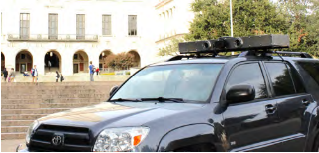
Fig. 7. The University of Texas Sensorium is a platform for automated and connected vehicle perception research. It includes stereo visible light cameras, an industrial-grade IMU, an automotive radar unit, a dual-antenna, dual-frequency software-defined GNSS receiver, 4G cellular connectivity, and a powerful internal computer.
