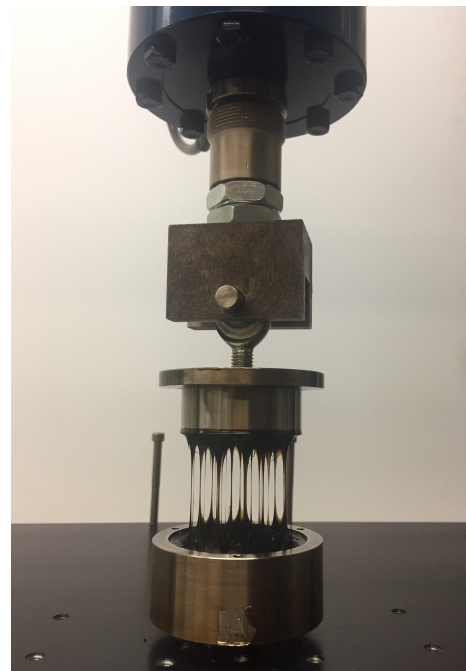
Figure 1. Test specimen at the end of a poker chip test, a simple and accurate way to assess asphalt binder ductility in a realistic stress state.
