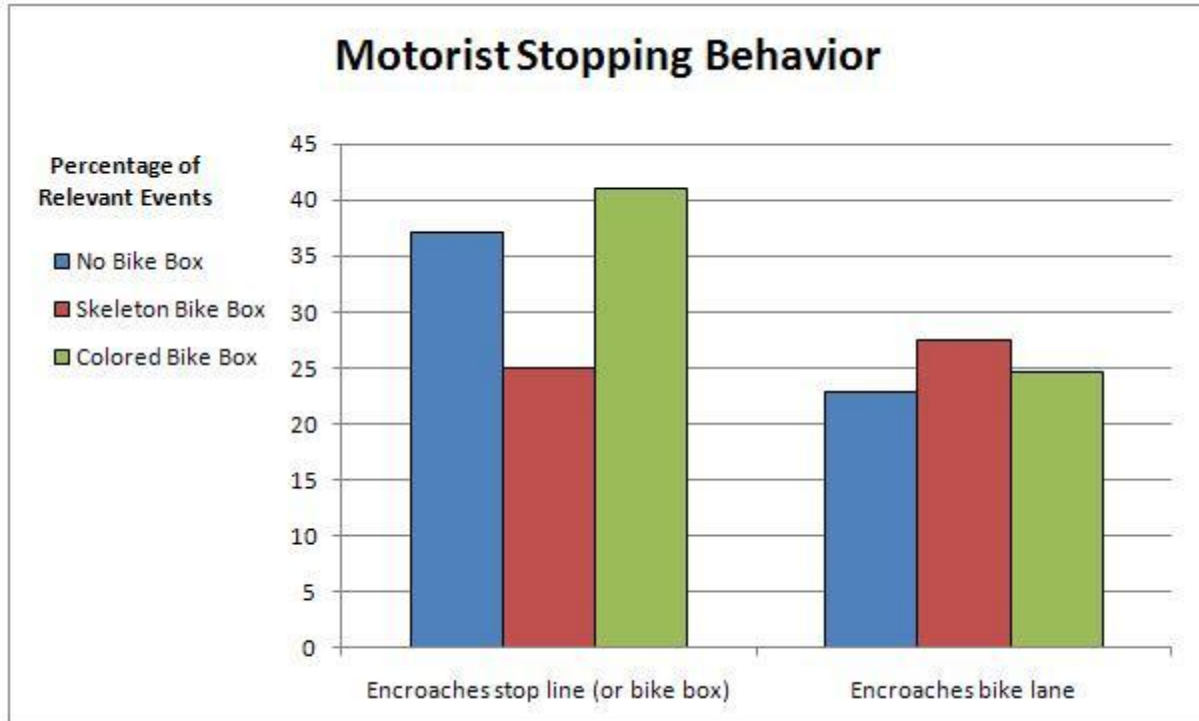
Figure 7. Motorist stopping position when a bicyclist is present at Anderson Lane and Shoal Creek Boulevard
