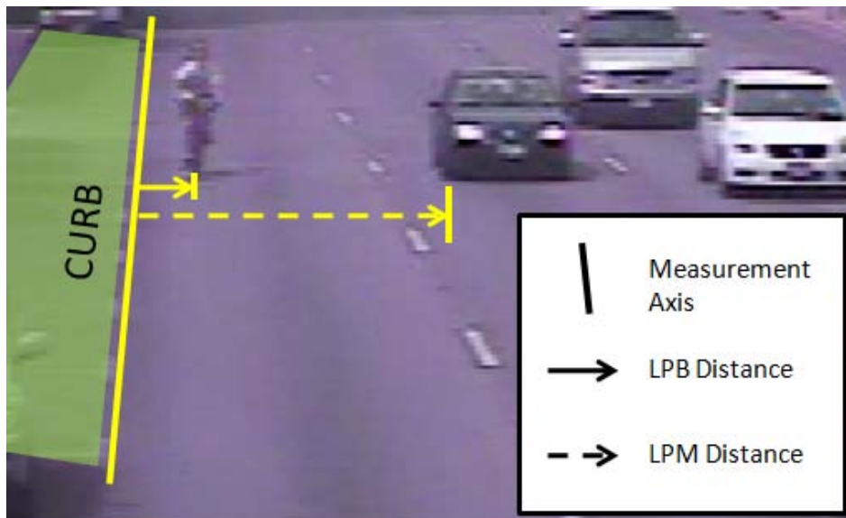
Figure 9. Method for measuring LPB and LPM during passing events
