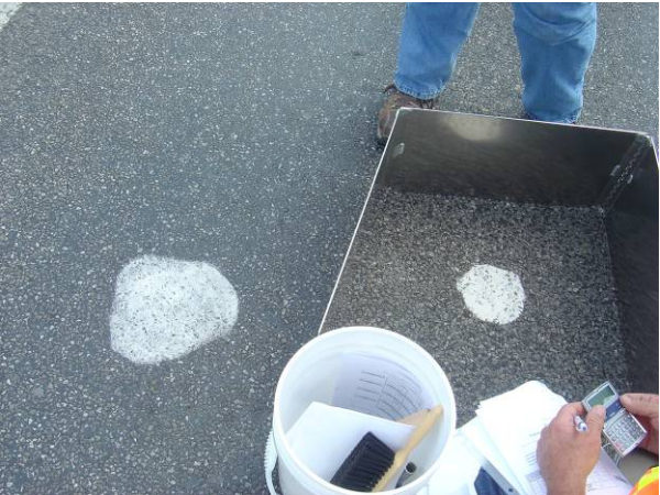
Figure 9. High Pavement Texture Difference
