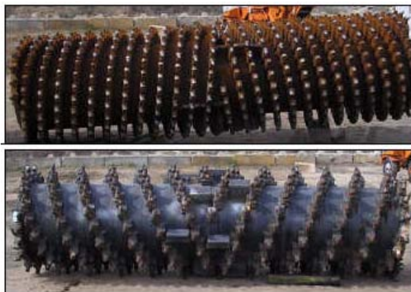
Micromilling Drum (top) and Conventional Milling Drum (bottom) (TRB 09-1857 pg. 4)
