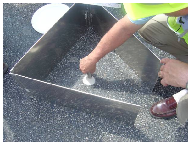
Figure 6. The Sand Patch Test
