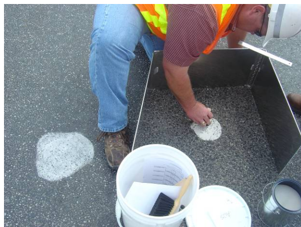
Figure 9. Performing the Sand Patch Test
