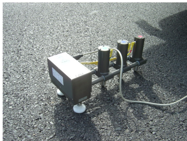
Portable Seismic Pavement Analyzer Equipment
