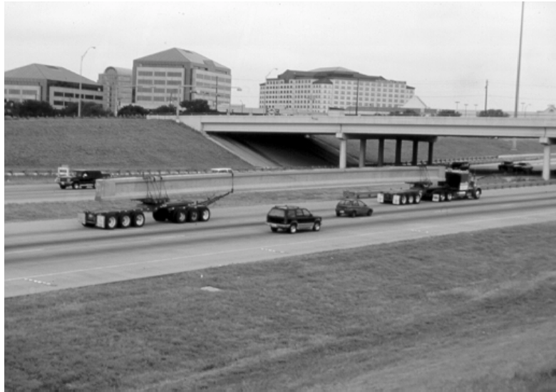
Figure 10.3 - Transportation of San Angelo Eastbound HPC Type IV Beams
