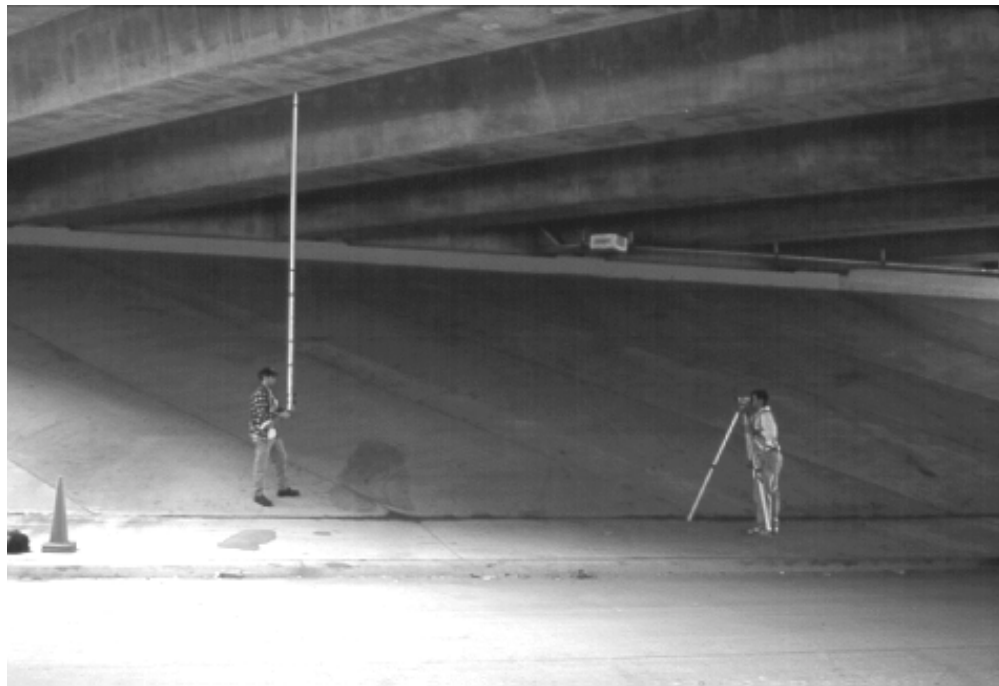
Figure 3.10 - Measurement of Camber Using the Precise Surveying System
