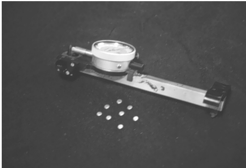
Figure 3.4 - DEMEC Mechanical Strain Gauge and Target Discs
