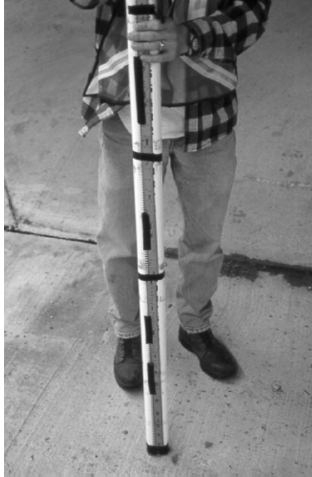
Figure 3.11 - Surveying Rod with Precision Scales Attached
