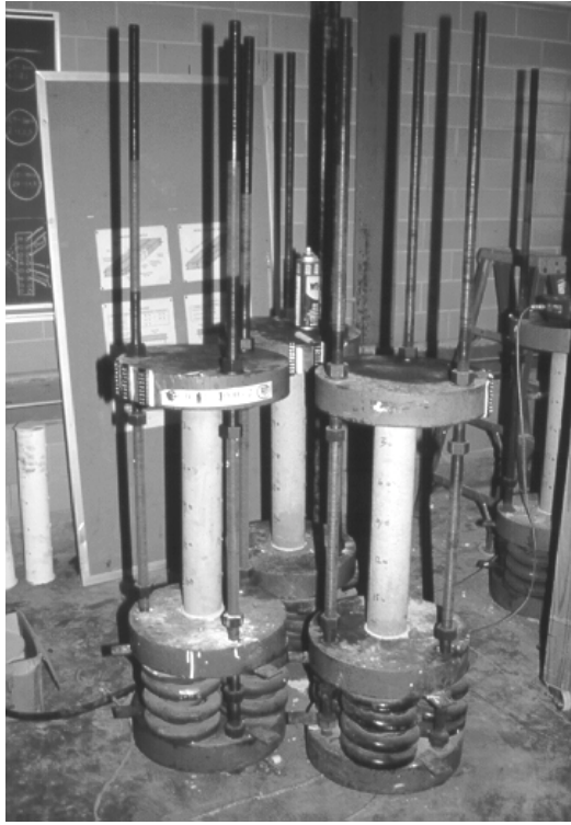
Figure 4.6 - Creep Test Frames with Specimens Under Sustained Load
