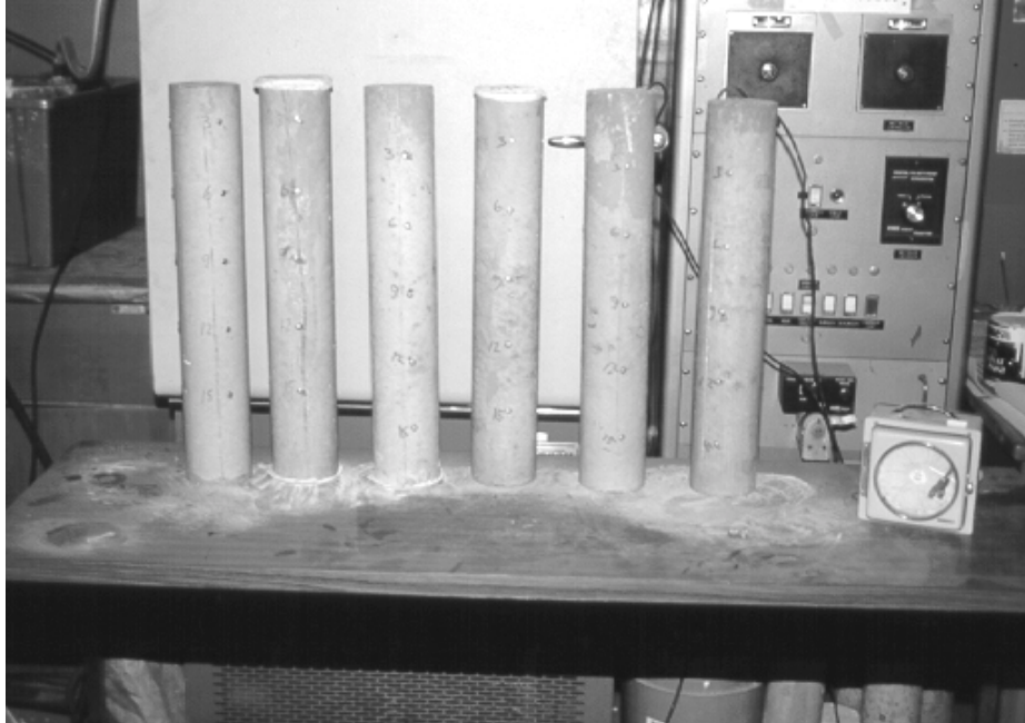
Figure 4.11 - Shrinkage (Unloaded) Specimens in Testing Room
