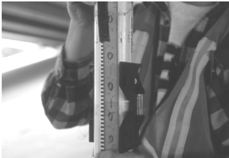
Figure 3.12 - Use of Post Level with Surveying Rod
