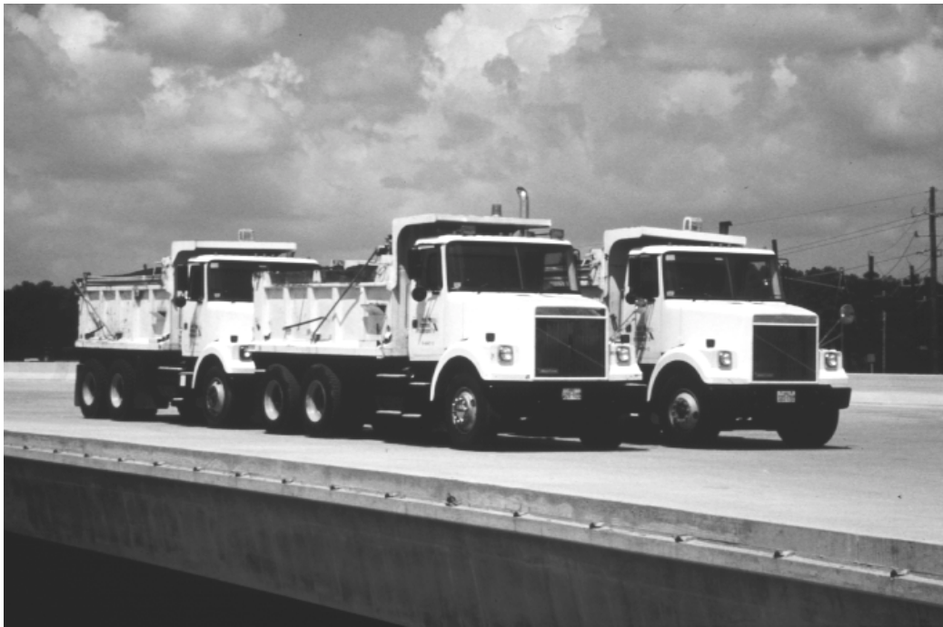
Figure 9.2 - Test Trucks Positioned in Louetta Loading Arrangement LS-B
