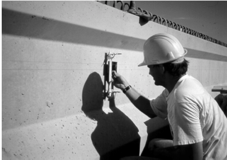
Figure 3.9 - Reading the Tensioned-Wire Deflection System
