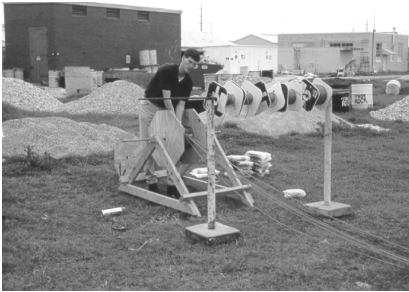
Figure 3.29 - Spooling of Leadwire for a Group of Gauges
