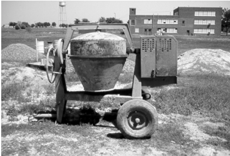
Figure 5.5: Rotary Mixing Unit used for Laboratory-Produced Concrete
