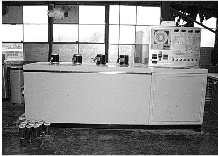
Figure 5.18: Freeze-Thaw Testing Machine
