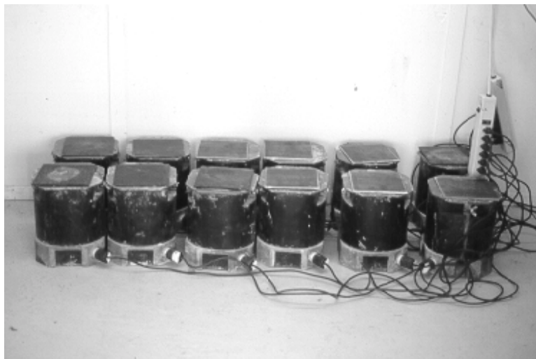
Figure 5.9: Cylinder Molds of the Match-Curing System
