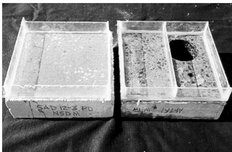
Figure 5.17: Chloride Ponding Blocks after 90-Day (left block) and 365-Day (right) Cycles
