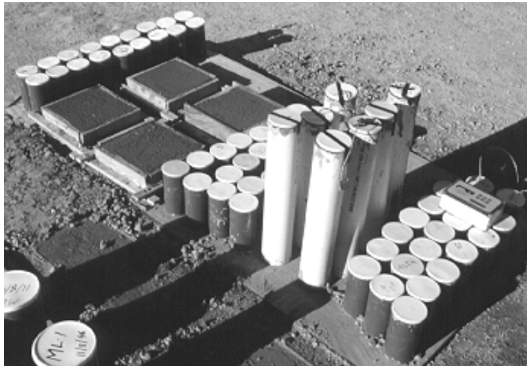
Figure 5.6: Representative QC/QA Test Specimens Cast for a Standard Deck Pour
