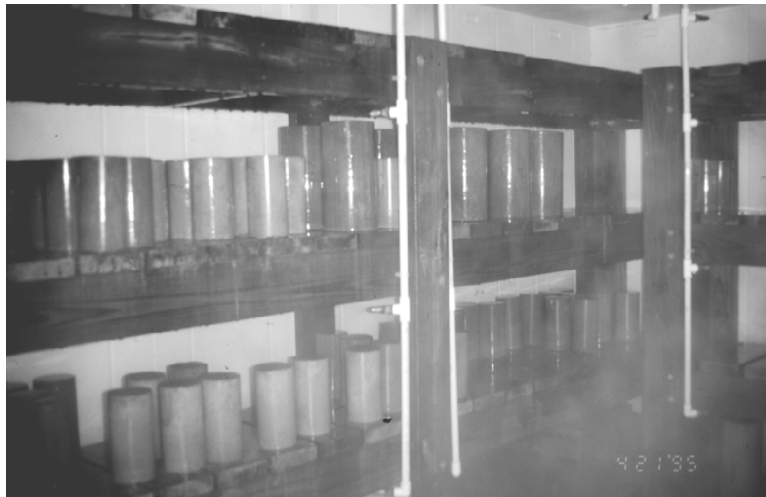
Figure 5.20: ASTM Moist-Curing Room
