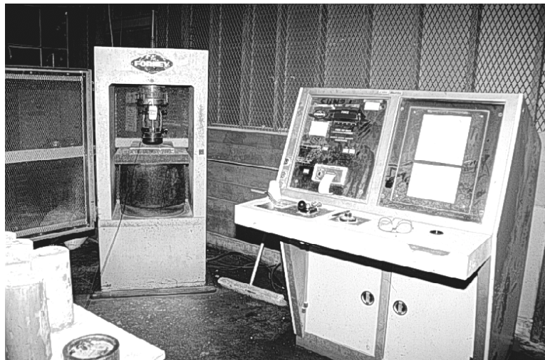
Figure 5.11: Compressive Strength and Elastic Modulus Forney Hydraulically Operated 600 kip Capacity Multiple Loading Rate Machine
