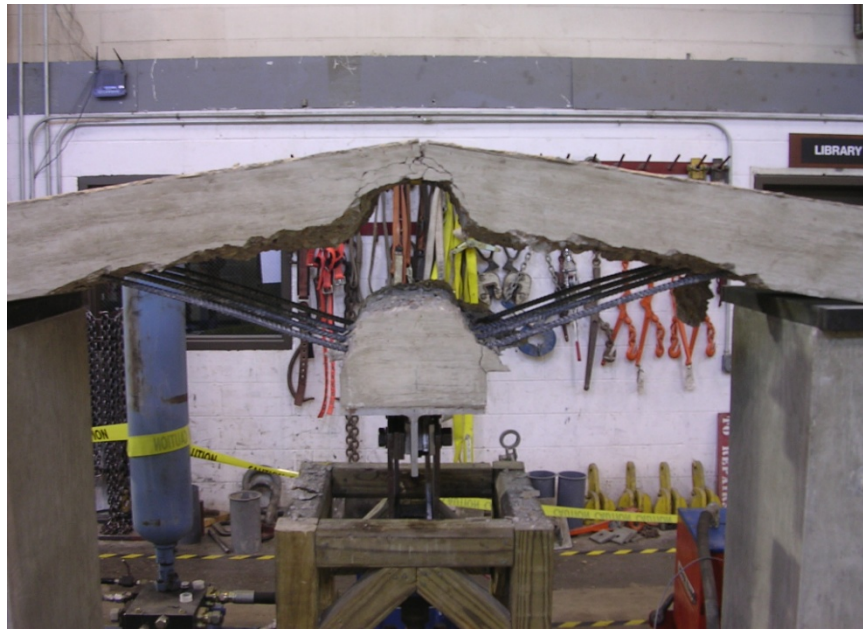
Figure 4.26: Specimen Showing Significant Arching
