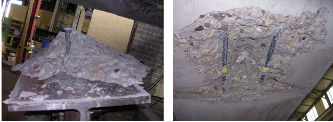
(a) (b) Figure 4.1: Failure Cone (a) Around Stud (b) Cone Void in Slab
