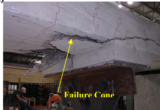
Figure 4.29: Failure Sequence for 7-in Studs Spaced Transversely (a) Horizontal Crack Formation (b) Haunch Splitting (c) Split Haunch with Failure Cone
