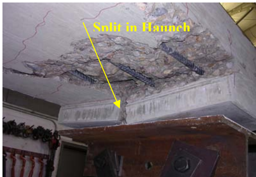
Figure 4.29: Failure Sequence for 7-in Studs Spaced Transversely (a) Horizontal Crack Formation (b) Haunch Splitting (c) Split Haunch with Failure Cone
