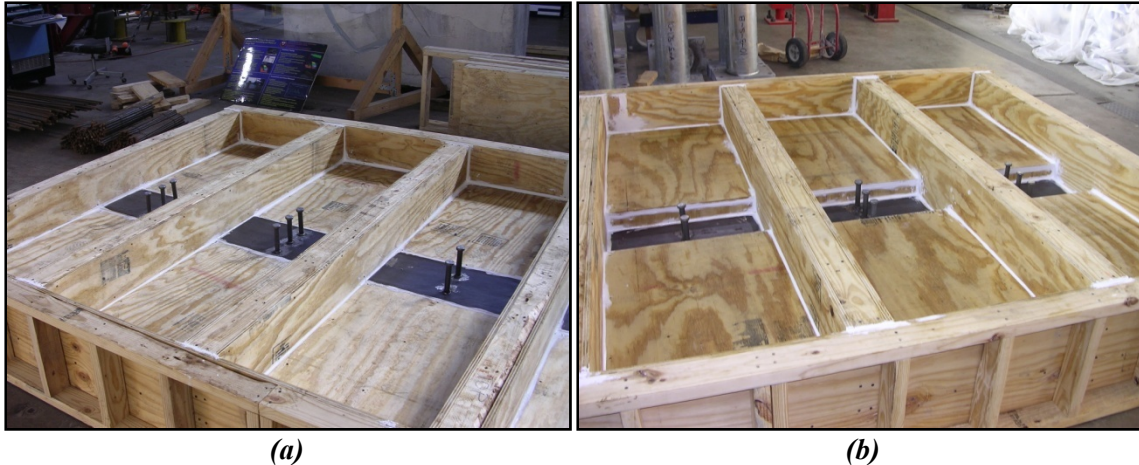
Figure 3.8: Formwork for Specimens with (a) No Haunch (b) 3-in. Haunch
