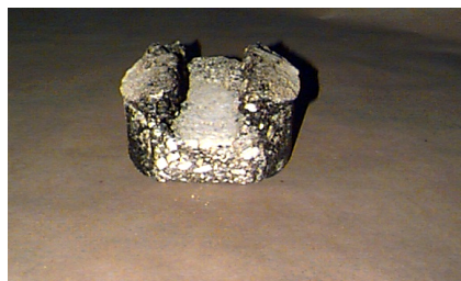
Figure 3. Specimen after HWTd Test (smooth surface-high degradation)
