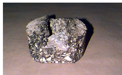
Figure 5. Specimen after HWTd Test (rough surface-low degradation)
