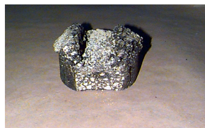
Figure 4. Specimen after HWTd Test (intermediate degradation)
