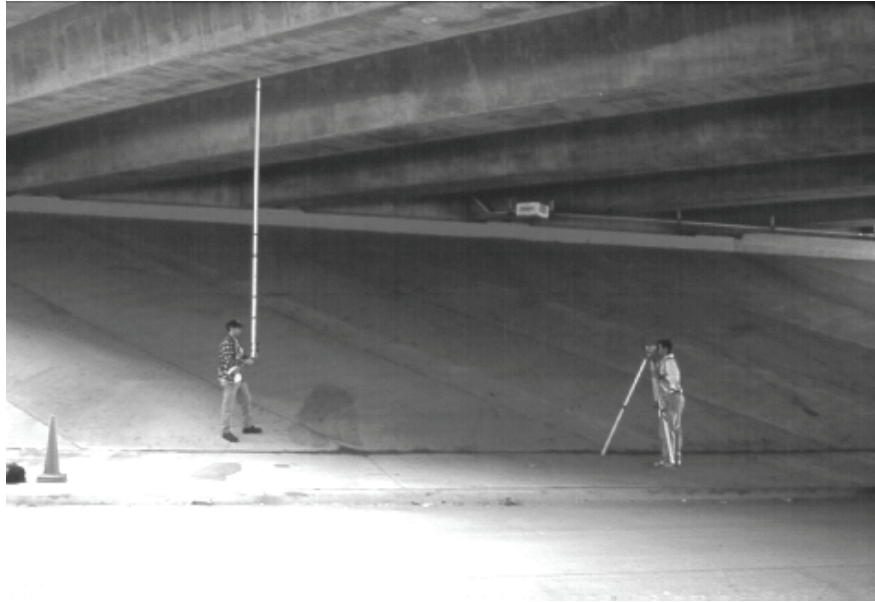
Figure 6.22 - Measurement of Camber Using the Precise Surveying System
