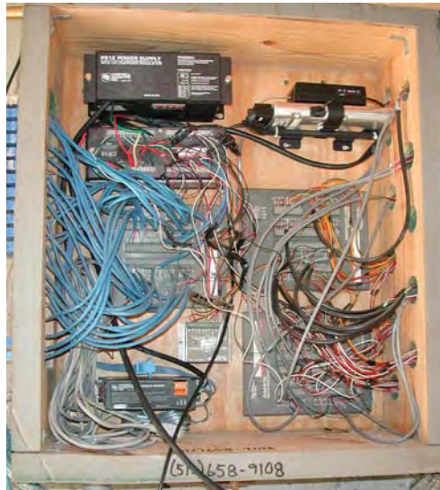
Figure 3.9: Remote-Monitoring Equipment in DAS Box
