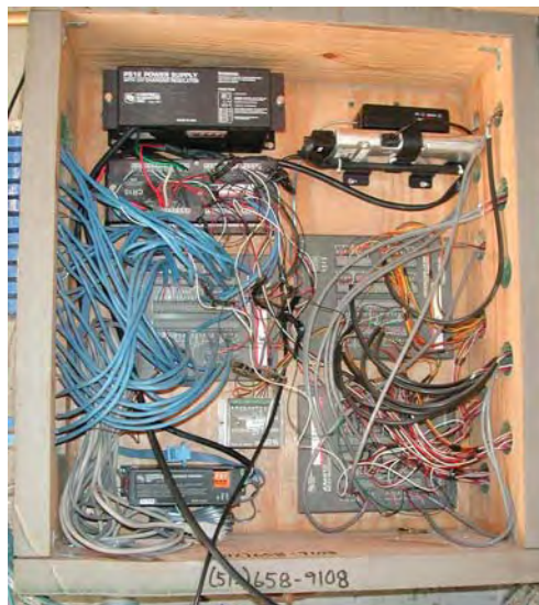
Figure 3.9 Remote-Monitoring Equipment in DAS Box
