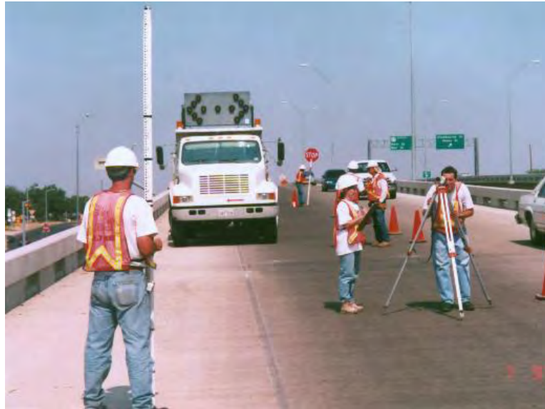
Figure 4.5 Camber Measurements at San Angelo
