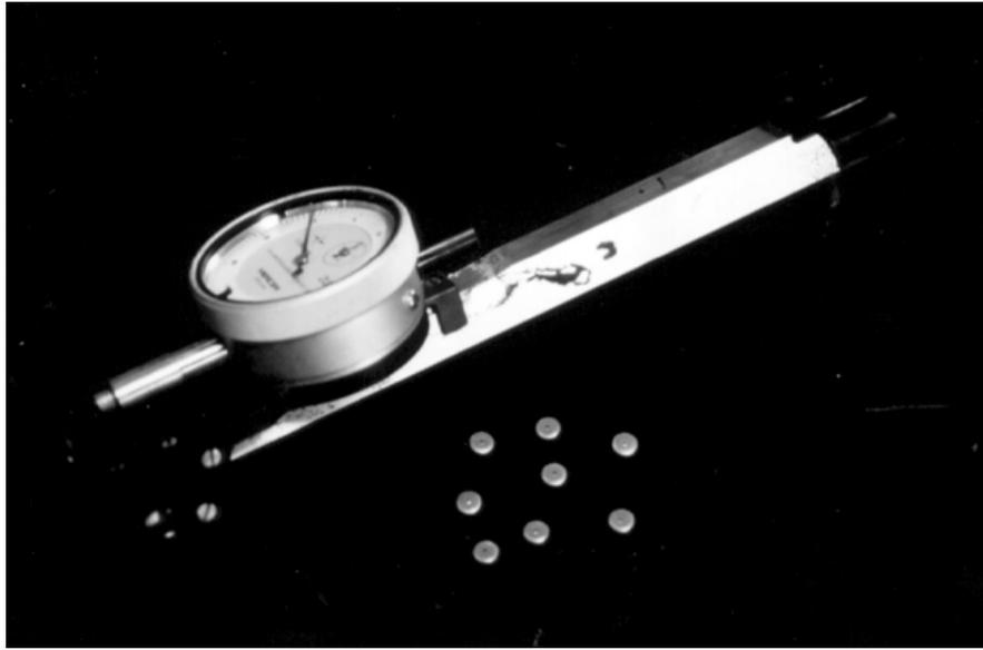
*Figure 3.13 Demec surface strain measuring system*
