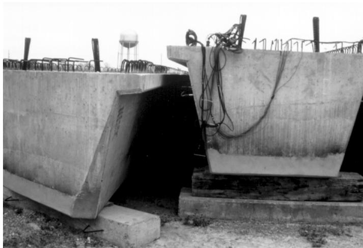
*Figure 4.5 Typical instrumented beam in storage at the prestressing plant*
