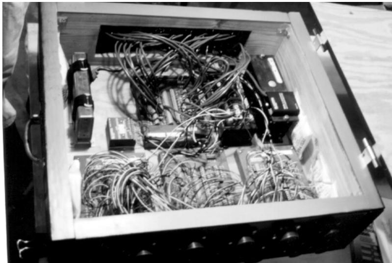
*Figure 3.18 Data acquisition system (DAS) box*
