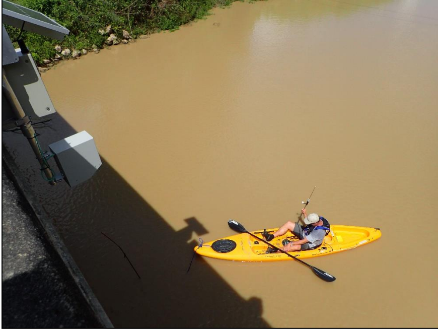
Figure 3-11 Spot velocity measurement taken in the field within the radar beam of the project stream gage
